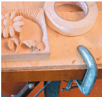
Double-sided turner's tape attaches work piece to clamped board
