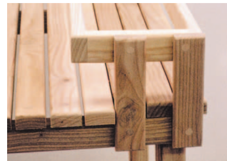
Horizontal frame consists of 2 long and 2 short boards
