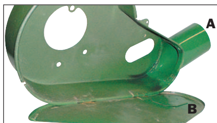
A. New port installed B. Old port covered
