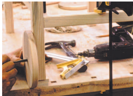
Block rear legs with 1" spacer and mark legs
