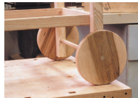
Apply glue to holes in wheels and press onto dowel ends
