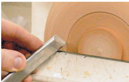
Use 3/4" skew to form 'v' grooves at texture borders
