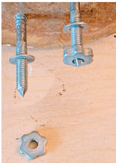
Carver's screws hold work piece to workbench
