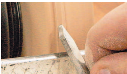
Use 1/4" parting tool as skew to create bead
