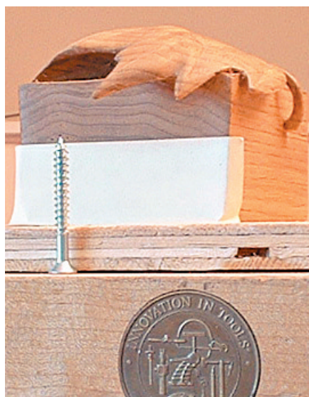
Masking tape marks depth of screw
