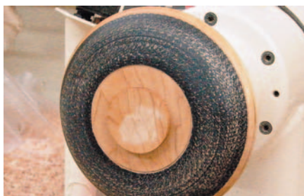
Highlight texturing with heavy tipped black marker
