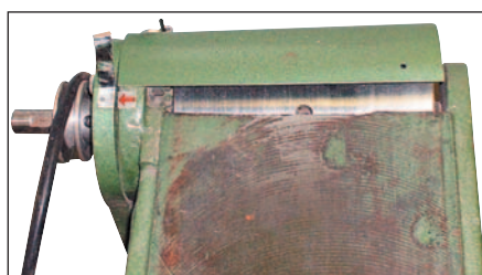
Original belt guard (at driven end of belt)
