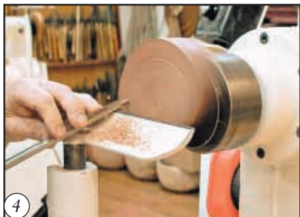
4 Make an outside cut with a gouge
