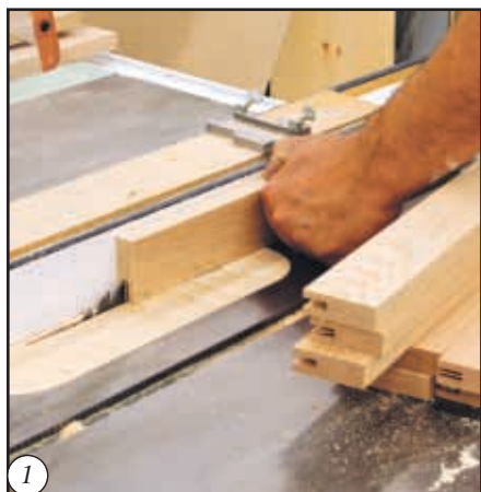
1 Cut grooves in stiles and rails
