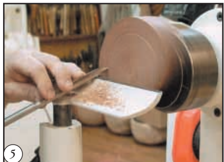
5 Move the toolrest to the face, and make a facing cut
