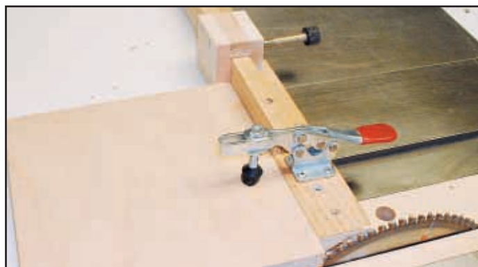
Toggle clamp and stop block fastened to fence
