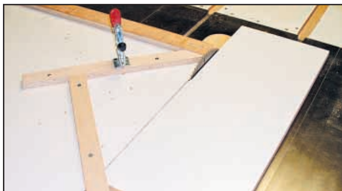
Temp fence and cut-off support
