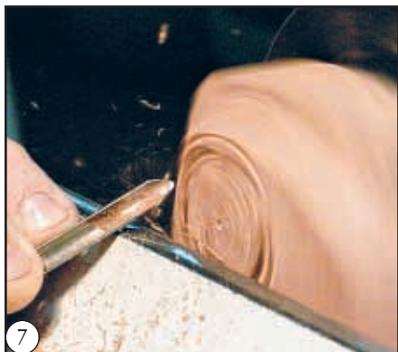
7 Move wood to remaining hole, find the centre of the plinth, and shape
