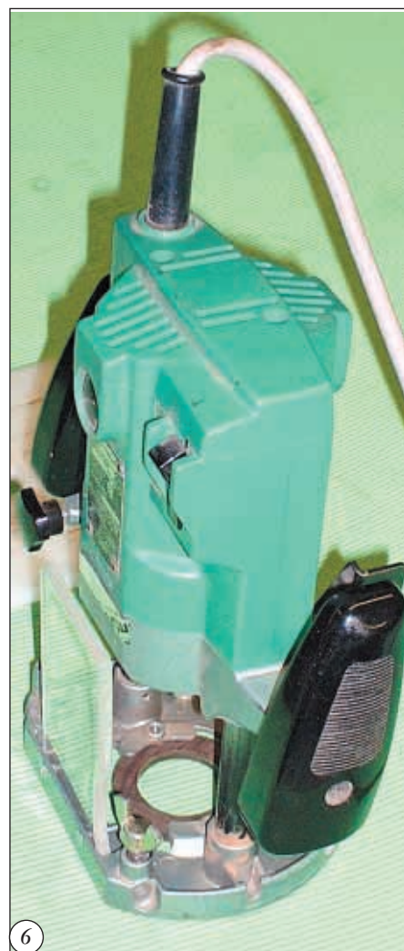
Add shield to control shaving direction and air flow
