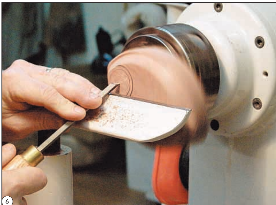
6 Find centre of plinth and drill hole for the screw of the trumpet
