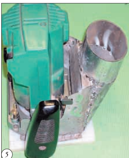
Welded hood with baffle
