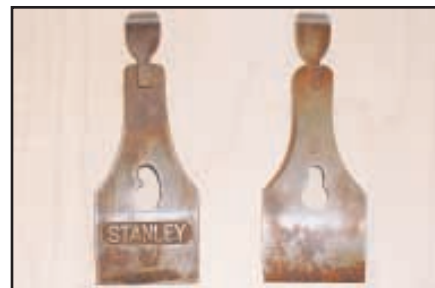
Kidney and keyhole lever cap styles.
