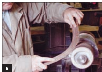
5 Profile the boomerang on a pneumatic drum sander.
