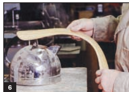
6 Tune the boomerang wing for proper lift by using a kettle to steam it and twist the wings slightly.
