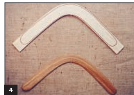
4 Trace the outline of your boomerang onto the boomerang blank.
