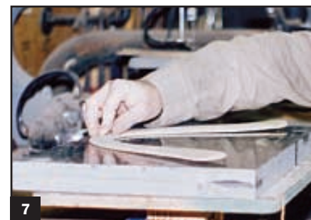
7 Checking the boomerang for proper wing twist after tuning it.
