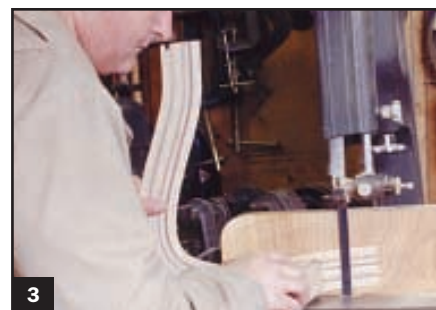
3 The easiest way to level the sides of the glued-up blank and to cut the blank into boomerangs is with the bandsaw.
