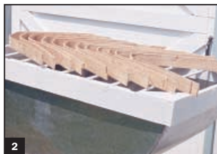
2 A typical mold with strips fully clamped.
