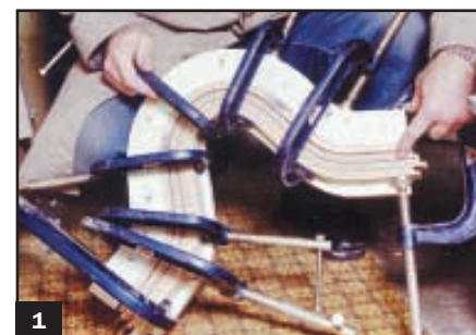
1 The inside surface of the boomerang mold must be waxed to prevent the glued layers of strips from sticking to it.
