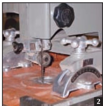
Under table area for best pick-up of fine dust and across-blade airflow.
