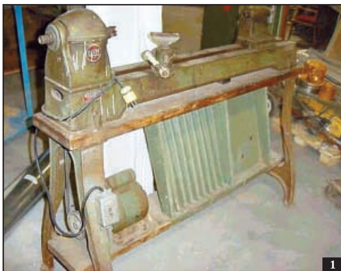
What I bought at the auction: a 1948 Delta 12"x36" Lathe (Model 1460).
