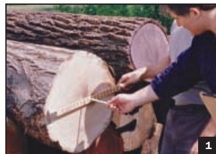
The author examines the timber for radial cutting. Normally, many sawmills will not radial or quarter cut logs because of the waste material created.
