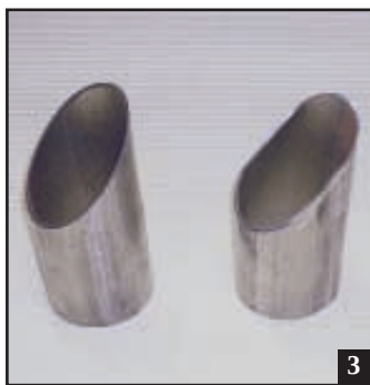
3" exhaust pipe. Left, cut at 45 degrees. Right, cut at 45 degrees and flattened to oval.
