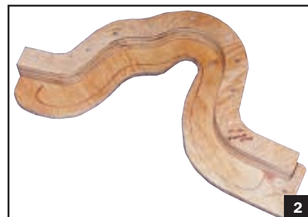
The boomerang mold is used first to shape the steamed wood strips and then to glue the strips together.
