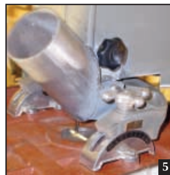
Dust chute in place and ready to be hooked up.
