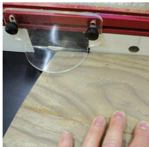
Pic.2 The finished doors. Walnut is notoriously difficult to match when gluing up the panels. Notice how the panel on the right is more consistent than the one on the left. Fortunately with time the colours will change, and the contrast won't be as obvious. Instead of using a lead-in pin for moulding the panels, bring the fences right up close to the cutter guide bearing (right)
