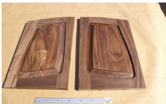
Pic.2 The finished doors. Walnut is notoriously difficult to match when gluing up the panels. Notice how the panel on the right is more consistent than the one on the left. Fortunately with time the colours will change, and the contrast won't be as obvious. Instead of using a lead-in pin for moulding the panels, bring the fences right up close to the cutter guide bearing (right)
