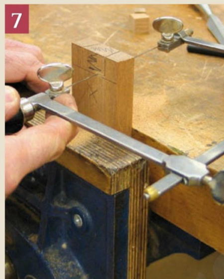
5 Marking Transfer the dovetail shape to the second piece (left) with a pencil, mark the waste and an X to remind you which way round the joint goes, but no other lines, then cut 'freestyle' to the waste side (above) vertically
