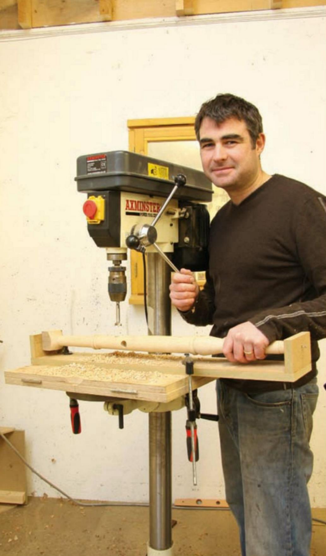
Drilling With the carriage for drilling the holes in the legs for the stretchers. Rob found that it helped to put a sash clamp across the ends for extra strength
