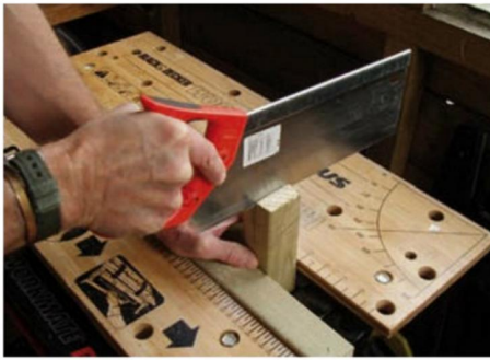
Joints Cutting the halving joint (above) using a piece of scrap to offset the leg in the Workmate. Gluing up the legs (left)
