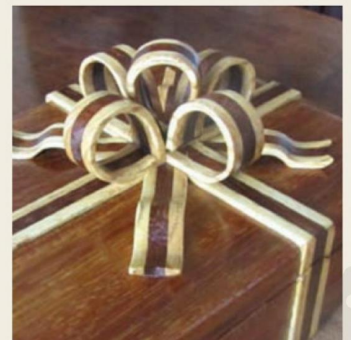
Pic.3 The first try at laying out the pieces proved the idea would work, but the ribbon loops are still uneven and rough, before sanding with a home-made 'flap wheel' to a finish (below)
