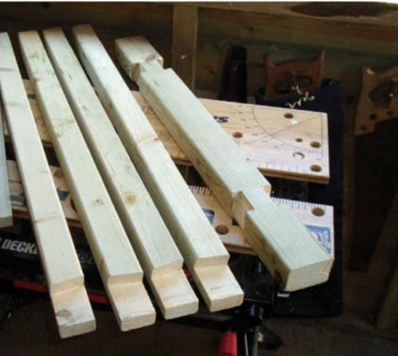
Parts The materials you need to make a sawhorse (above) and the angled halving joint glued up with polyurethane adhesive for a waterproof bond (left). The finished sawhorse (below) in treated timber should last for years
