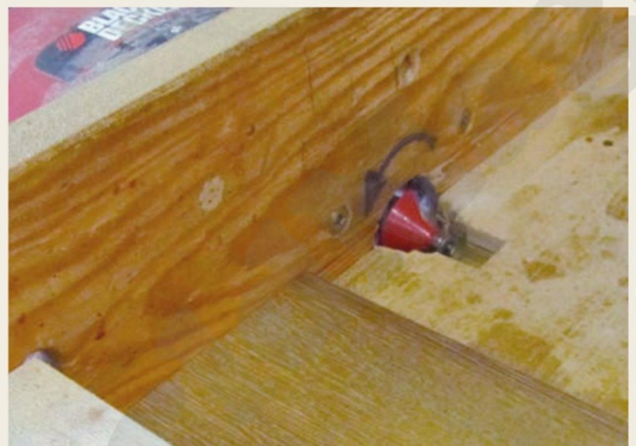
Pic.4 Tony uses a V-cutter in his horizontal router table to cut the mitres on the end of the box sides. Use a backing piece to reduce tear-out and push along the fence. Leaving a flat on the end of the mitre helps with running against the fence and during glue-up
