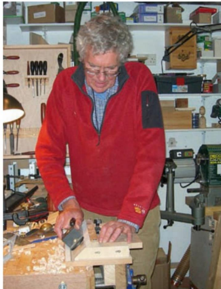
Inset The Inset Plane fitted into a wooden 'body' with 45° cheeks for chamfering
