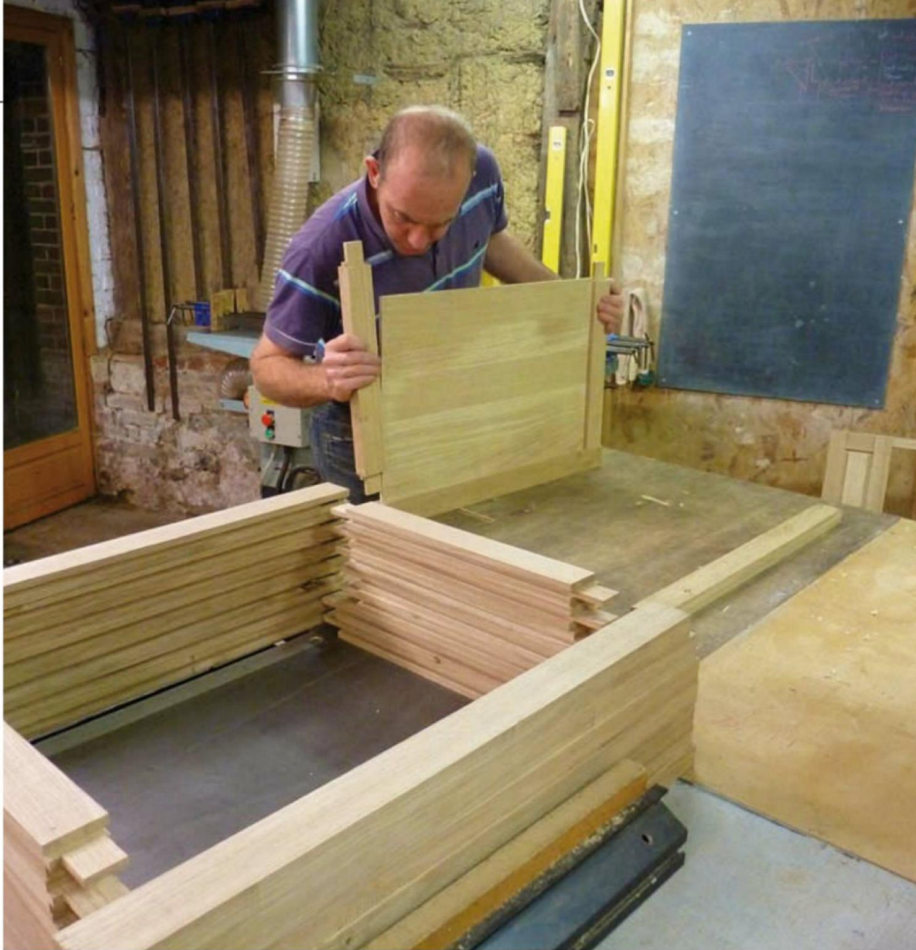
Tenons Dry assembling the doors and panels (above). Notice how many tenons Gordon had to cut! Checking the fit of the small panels to the top and bottom rails (left)
