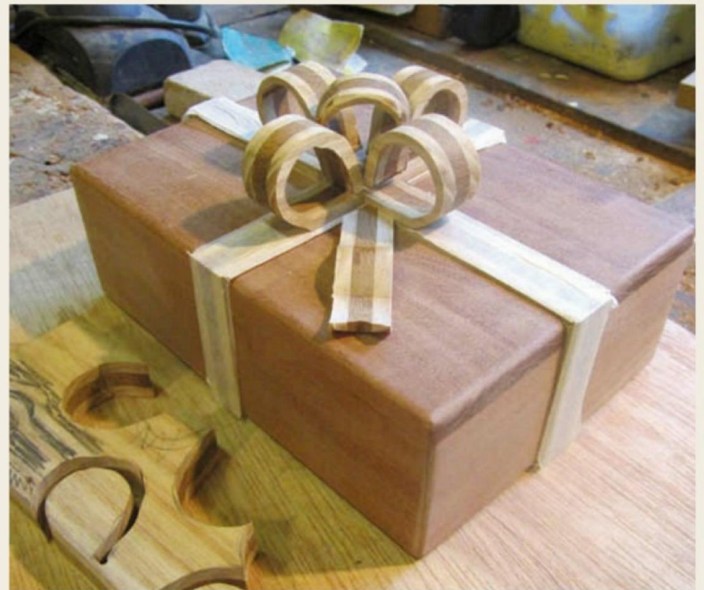
Pic.3 The first try at laying out the pieces proved the idea would work, but the ribbon loops are still uneven and rough, before sanding with a home-made 'flap wheel' to a finish (below)
