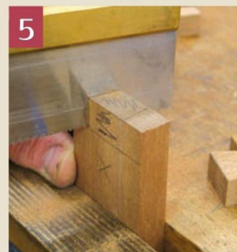
5 Marking Transfer the dovetail shape to the second piece (left) with a pencil, mark the waste and an X to remind you which way round the joint goes, but no other lines, then cut 'freestyle' to the waste side (above) vertically
