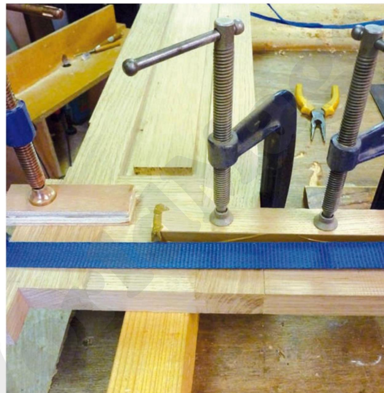
Pic.5 Offset sash cramps (left) being used to pull one of the sections of the face frame into square when gluing. Gordon used stabilising blocks to make sure the bottom rail remains flush with the dividing panel (right). The cramps weren't that tight, so that the ratchet cramps would pull the joint up firmly
