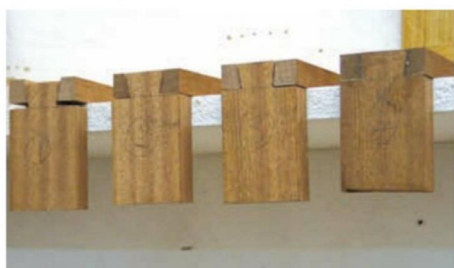
8 Finishing Chop the last of the waste away (right), chiselling on a block and assemble the joint (above). Make sure you number the joints to monitor your progress (left)
