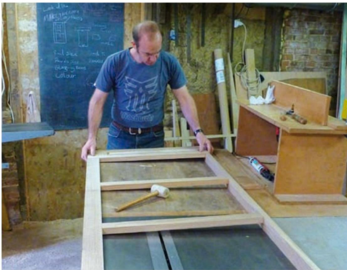
Pic.5 Offset sash cramps (left) being used to pull one of the sections of the face frame into square when gluing. Gordon used stabilising blocks to make sure the bottom rail remains flush with the dividing panel (right). The cramps weren't that tight, so that the ratchet cramps would pull the joint up firmly
