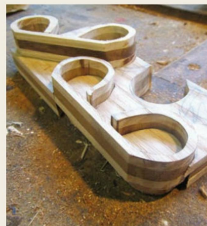
Pic.1 For a bow, cut two B-shaped pieces, leaving a straight section between the loops as long as the ribbon is wide. Chisel a halving joint so that the two half-bows sit flat across each other. Glue a single loop diagonally on top to hide the join
