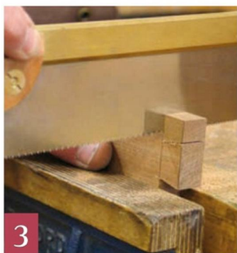
3 Shoulders A couple of completed five-minute joints (top) and making a cut to the shoulder lines on the tail piece (above)
