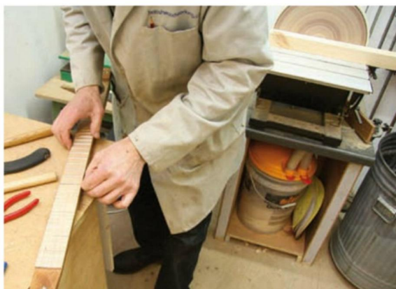
Frets I used the Mini Silky Saw which I had reground last year with a Japanese tooth configuration to cut the fret slots. Each fret was 'sanded' to length on the disc sander
