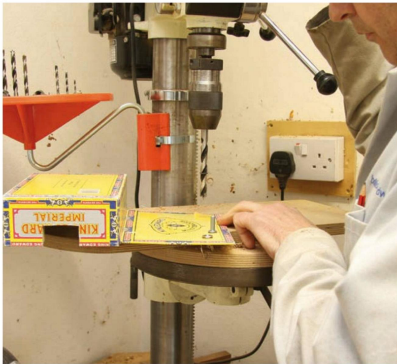
Inside Nick used Fisch drill bits that Axminster have started bringing in recently to make the holes for the volume control and output jack. They are really sharp. The neck (above) is supported by reinforcement inside the box, with corner blocks holding it all
