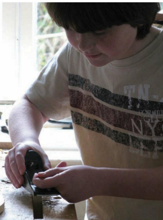
Towels Tom planing the end-grain on the towel tidy with a Stanley block plane (left). Preparation is good: plans show the parts marked out for the towel tidy (above), showing which tools are used and where. Boring a corner hole with the brace and a 1in centre bit (below)
