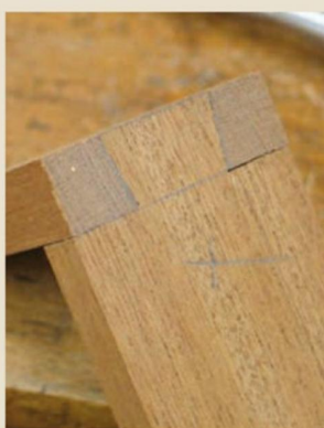
8 Finishing Chop the last of the waste away (right), chiselling on a block and assemble the joint (above). Make sure you number the joints to monitor your progress (left)
