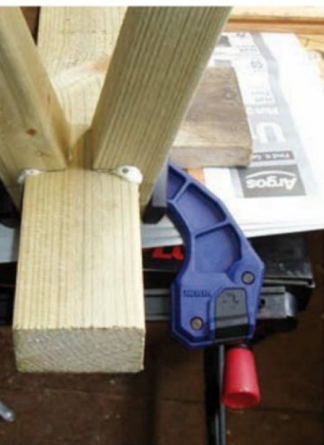
Parts The materials you need to make a sawhorse (above) and the angled halving joint glued up with polyurethane adhesive for a waterproof bond (left). The finished sawhorse (below) in treated timber should last for years
