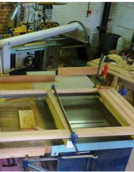
Pic.5 Offset sash cramps (left) being used to pull one of the sections of the face frame into square when gluing. Gordon used stabilising blocks to make sure the bottom rail remains flush with the dividing panel (right). The cramps weren't that tight, so that the ratchet cramps would pull the joint up firmly
