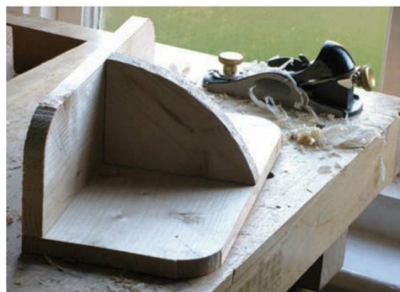
Finishing The cut out parts of the towel tidy offered up for fine tuning the fit (above)
