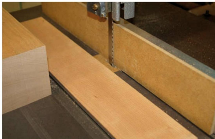
Pic.3 The finish off the Premium blade is superb, with only the slightest marking, especially if you keep it moving
