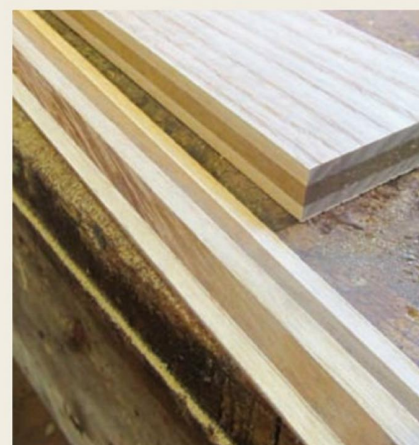
caption Glue thin boards together using contrasting colours and slice the sandwich into slim pieces. The sandwiched can be thickened to suit a straight router cutter for grooving (below). Cut the box in half after routing the grooves
