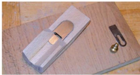
Inset The Inset Plane fitted into a wooden 'body' with 45° cheeks for chamfering
