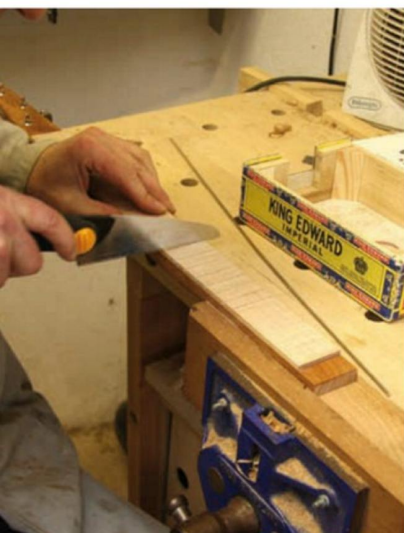
Frets I used the Mini Silky Saw which I had reground last year with a Japanese tooth configuration to cut the fret slots. Each fret was 'sanded' to length on the disc sander
