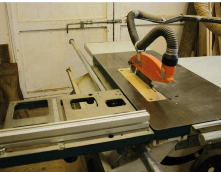
False Gerwyn already has a sliding table for his sliding carriage (above) on his tablesaw (left). The crown guard has to be removed for tenoning, which makes it dustier but otherwise not particularly dangerous if your hands are kept well away from the blade
