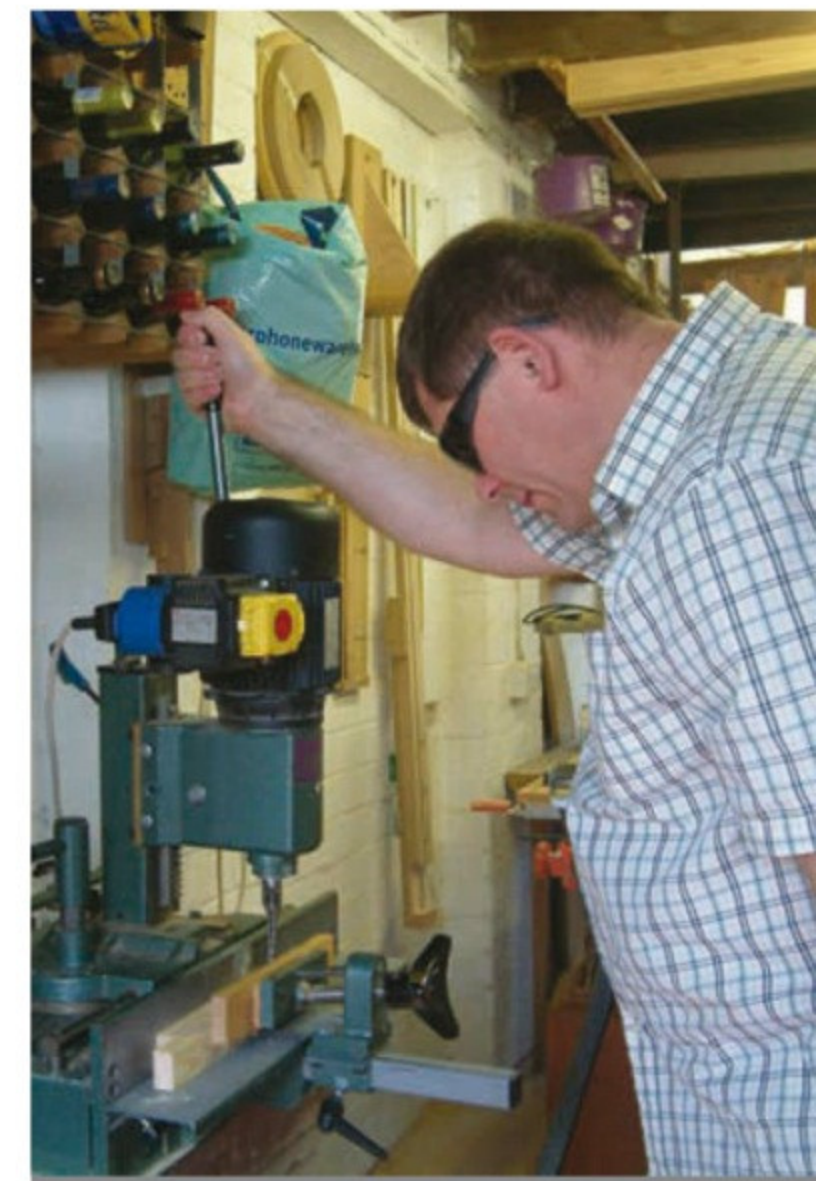
Traditional One of the options was to cut a traditional mortise and a traditional tenon. Here Steve is cutting the mortise with a 1/4in hollow mortise chisel
