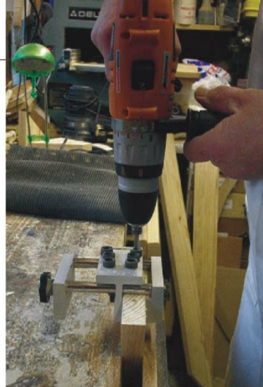
Pic.4 Joining the two frames with the turned stretchers is very fiddly. This attempt (left) failed and Bill had to fix the pieces to a board to keep it all true
