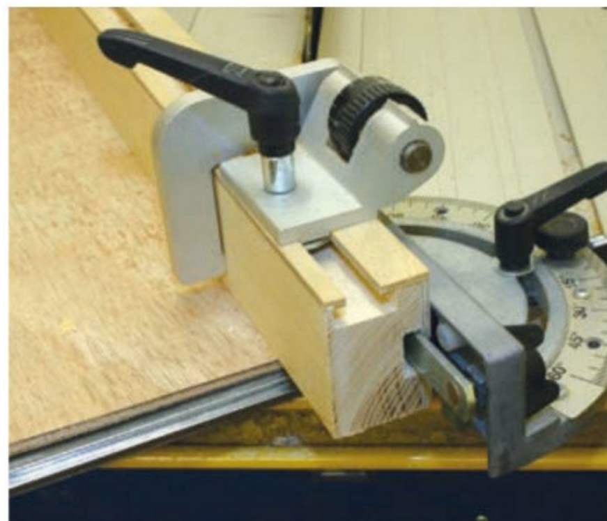
Pic.3 To make a sliding fence with a slot for adjustable stops you have to rout channels in the fence, then cover them with ply
