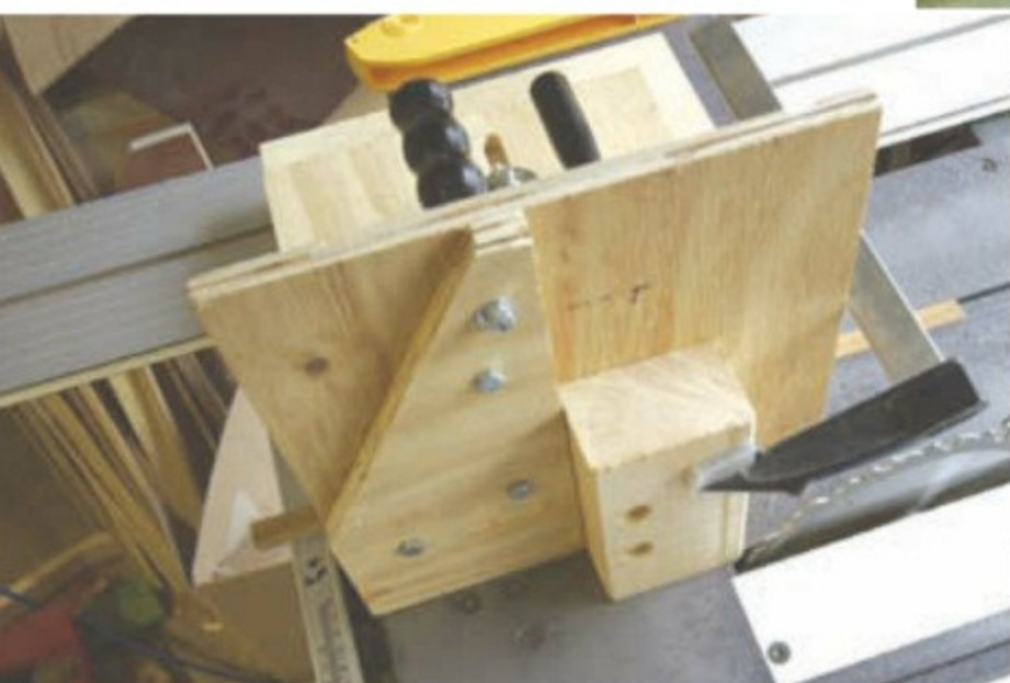
Adjustable jig Ernie Bowden's tenoning jig is adjustable in a couple of ways, and has handles for extra safety. Notice how the jig runs with a wooden bar in the mitre slot as a guide
