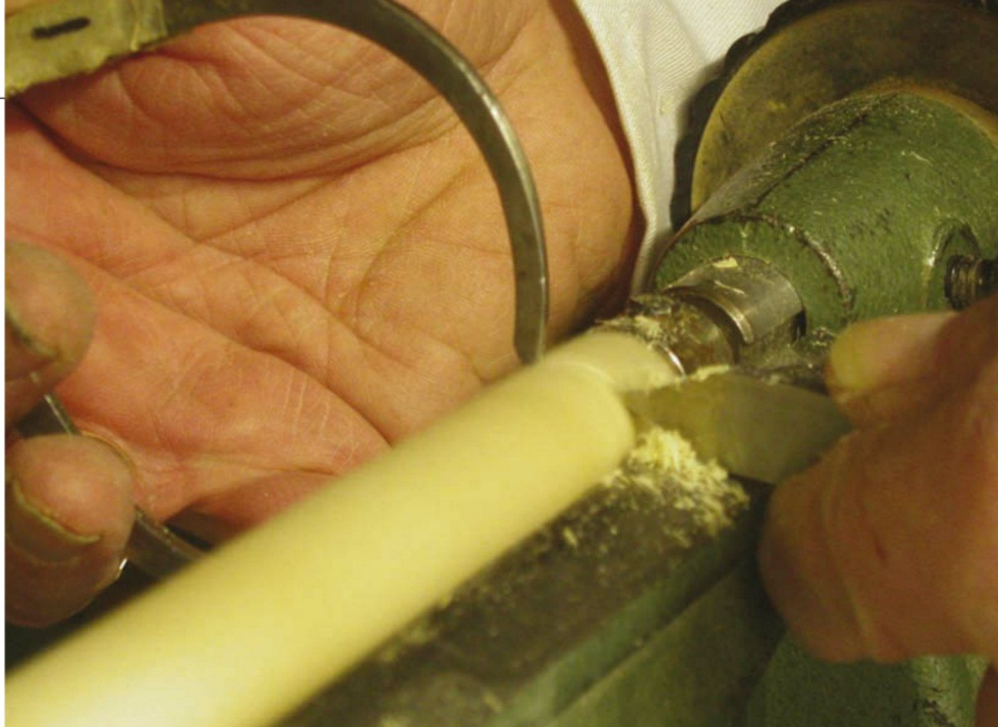
Pic.8 Use callipers to get the tenons on the end of the turned stretchers spot on
