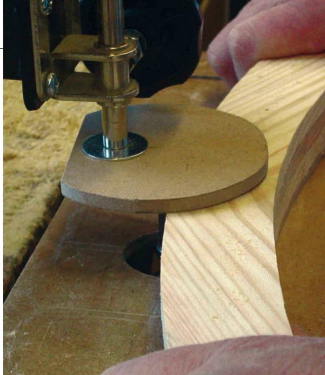
Pic.2 Initially a template fixed below the rails guides a cutter (above left), but you may well need to use the rail itself to finish the job because the cutter probably won't be long enough and you will need to raise it up. A guard (above right) offers protection and afterwards you can sand the leg smooth with a drum sander fitted in a pillar drill
