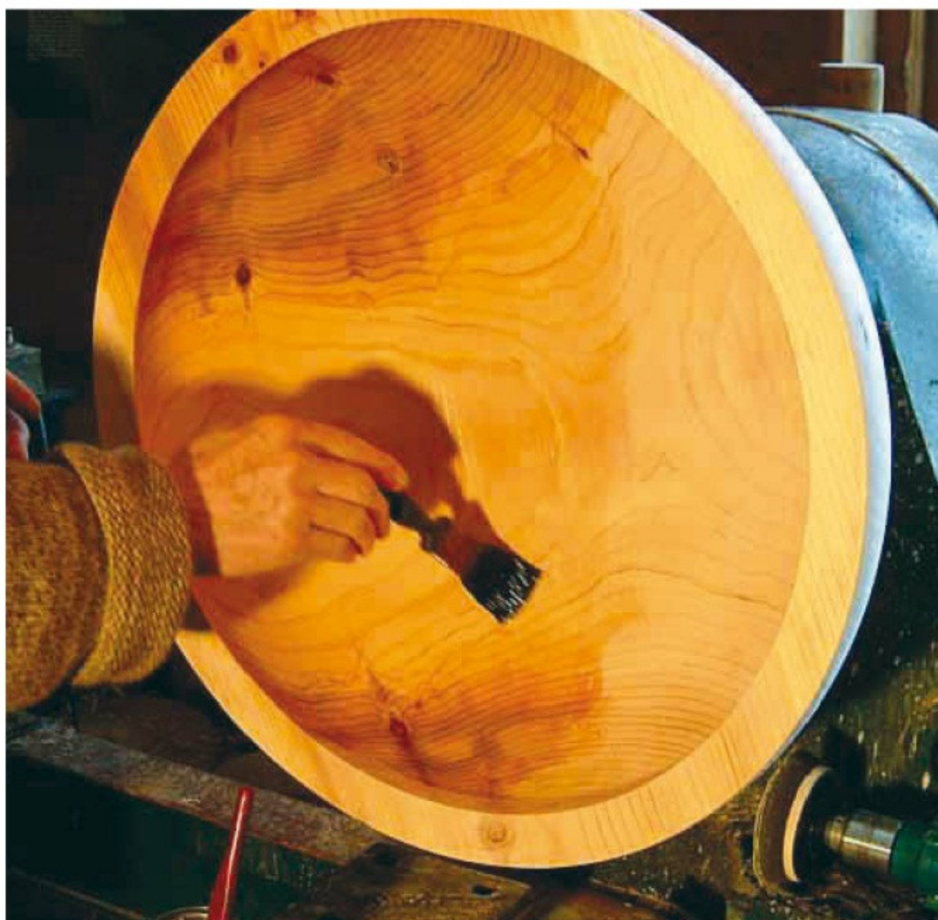
Pic.3 Cedar looks good with a very low shine. I chose to use sesame oil for the first coat and three coats of liquid paraffin later on
