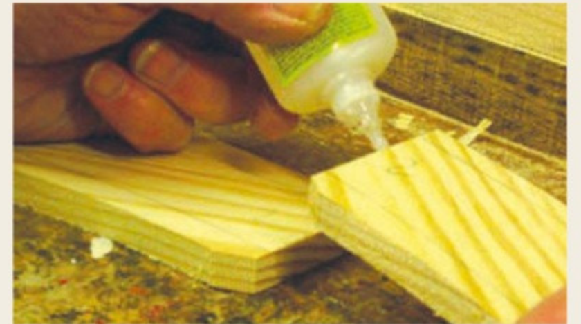
Pic.1 Using SloZap cyanoacrylate instant glue to fix laminates together temporarily before gluing up the sandwich (below)
