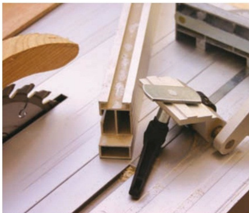
Pic.2 Extruded aluminium fences can be fine, but by replacing them with a wooden fence you have far greater flexibility
