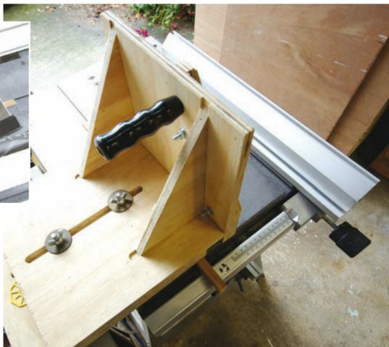
Adjustable jig Ernie Bowden's tenoning jig is adjustable in a couple of ways, and has handles for extra safety. Notice how the jig runs with a wooden bar in the mitre slot as a guide
