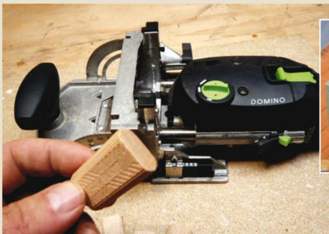
Pic.1 The Festool Domino System produces an elongated mortise to take a solid wood 'biscuit'. By increasing the 'waggle' of the cutter the mortise can be made into a longer slot for edge jointing
