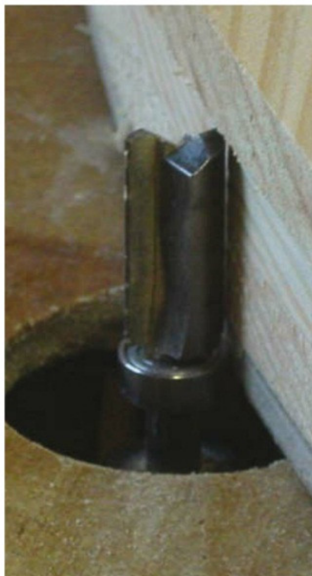
Pic.2 Initially a template fixed below the rails guides a cutter (above left), but you may well need to use the rail itself to finish the job because the cutter probably won't be long enough and you will need to raise it up. A guard (above right) offers protection and afterwards you can sand the leg smooth with a drum sander fitted in a pillar drill
