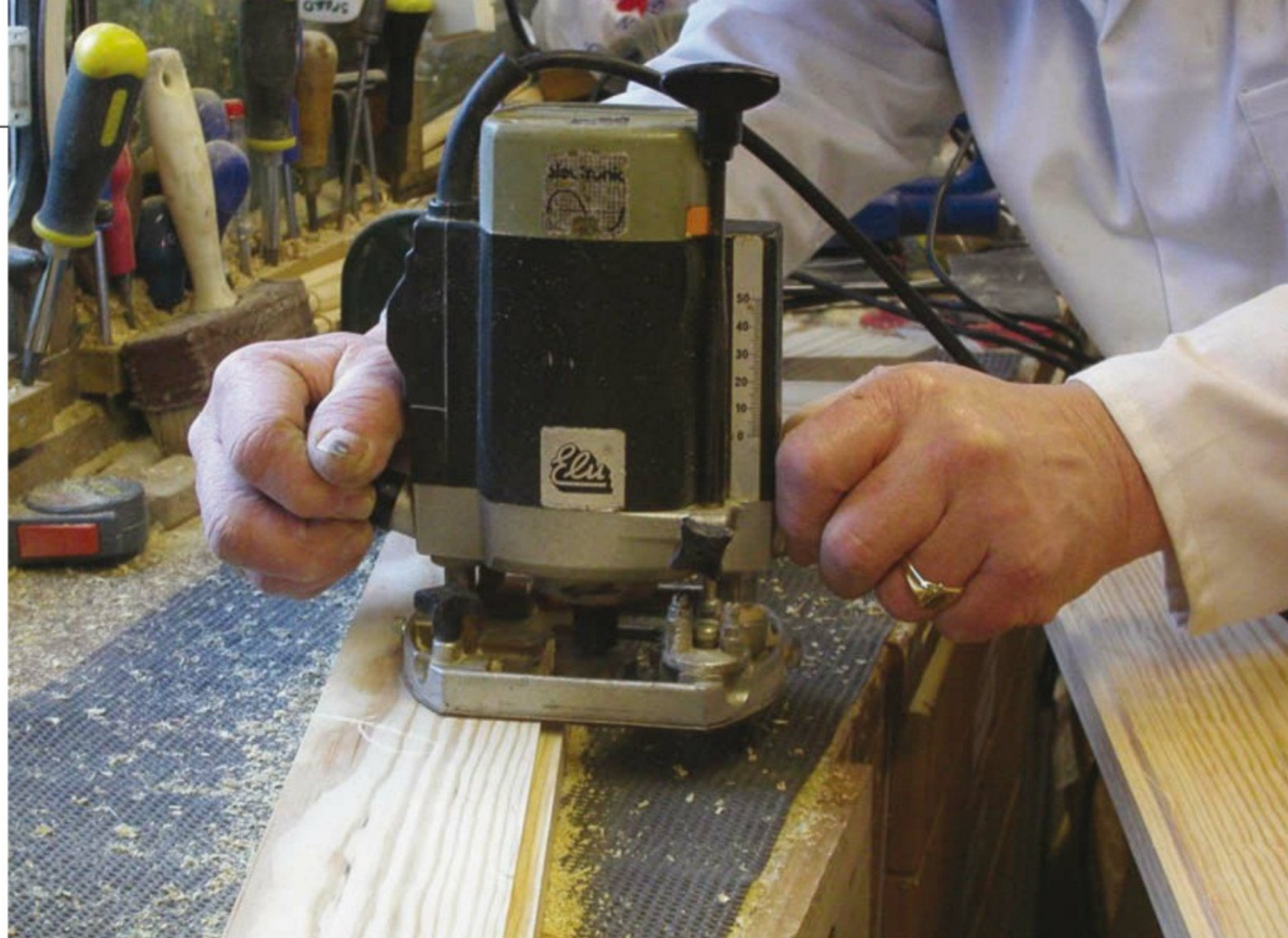
Pic.6 Rebating one of the components for the top for the glass
