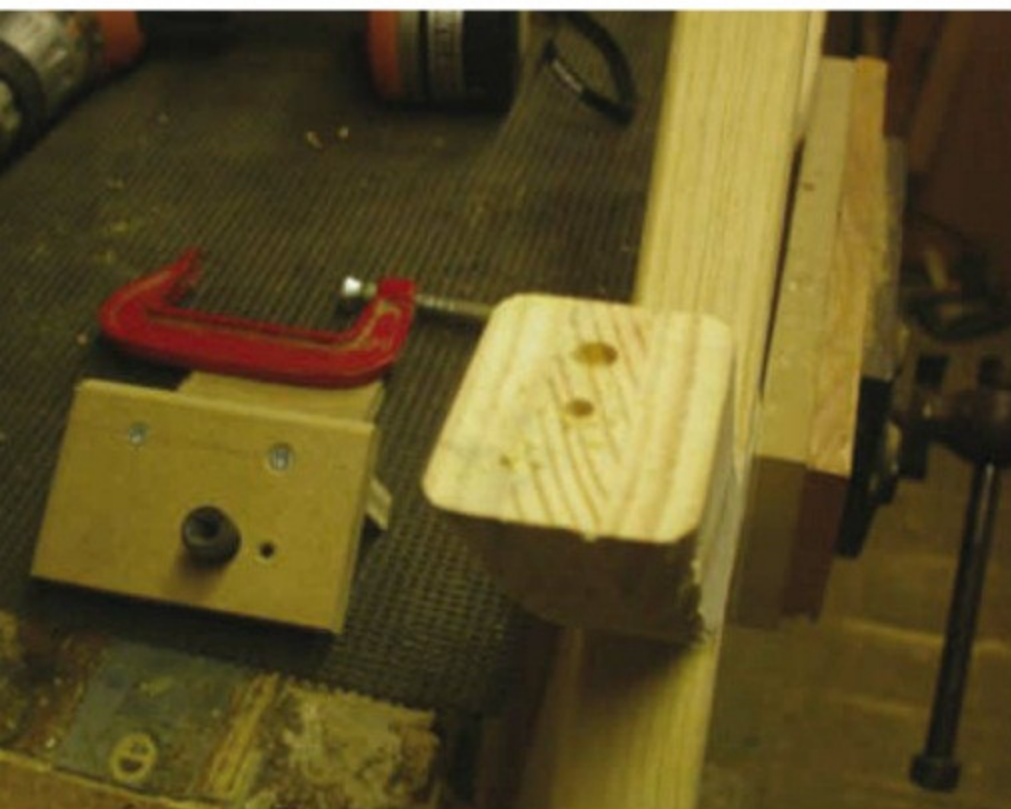
Pic.7 Bill uses a jig for drilling the holes for a screw and a dowel to attach the legs to the top of the table
