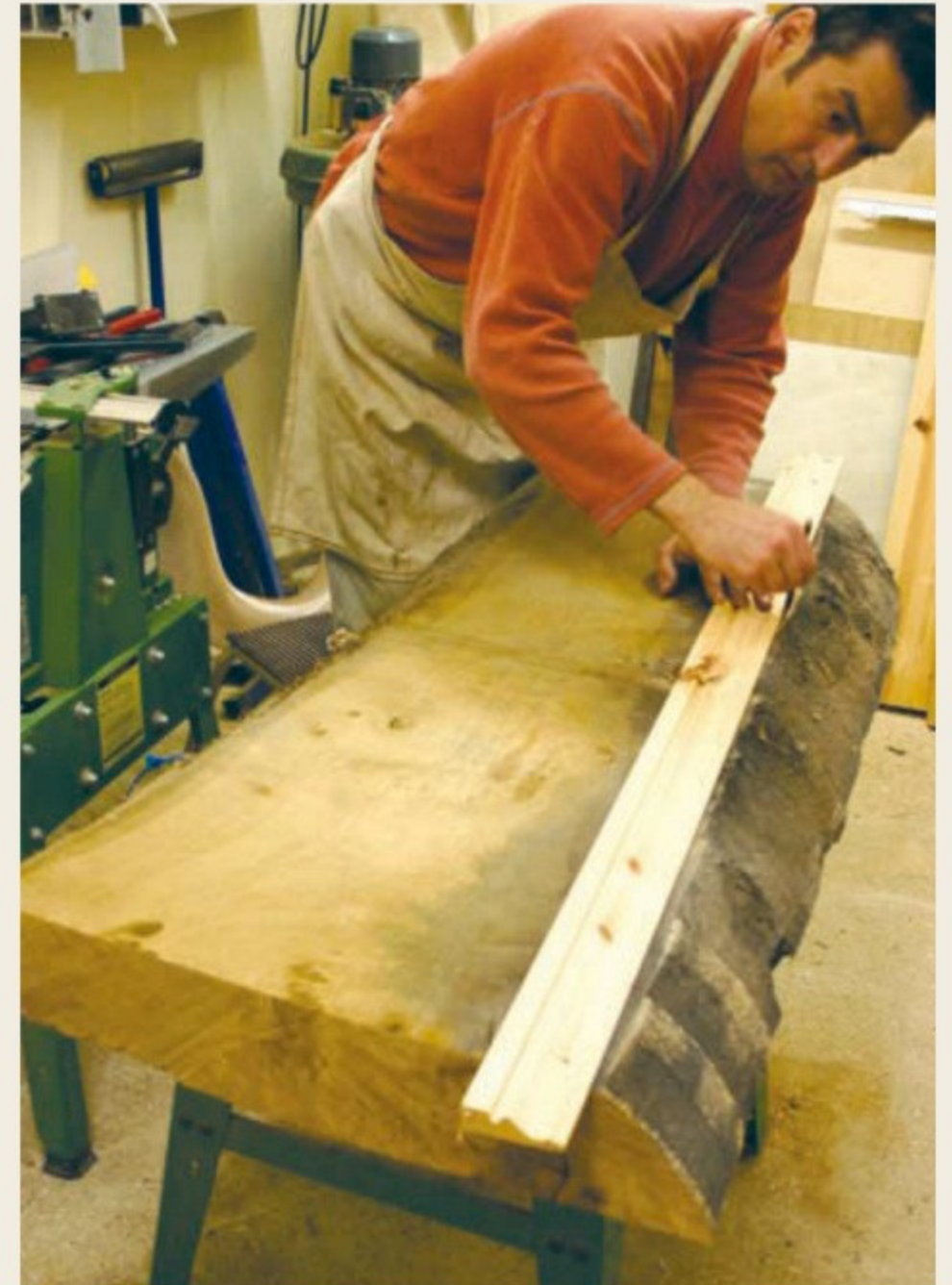
Straight edge Ideally start with the truest edge when it comes to removing the wane. You don't have to use a handsaw for this job!
