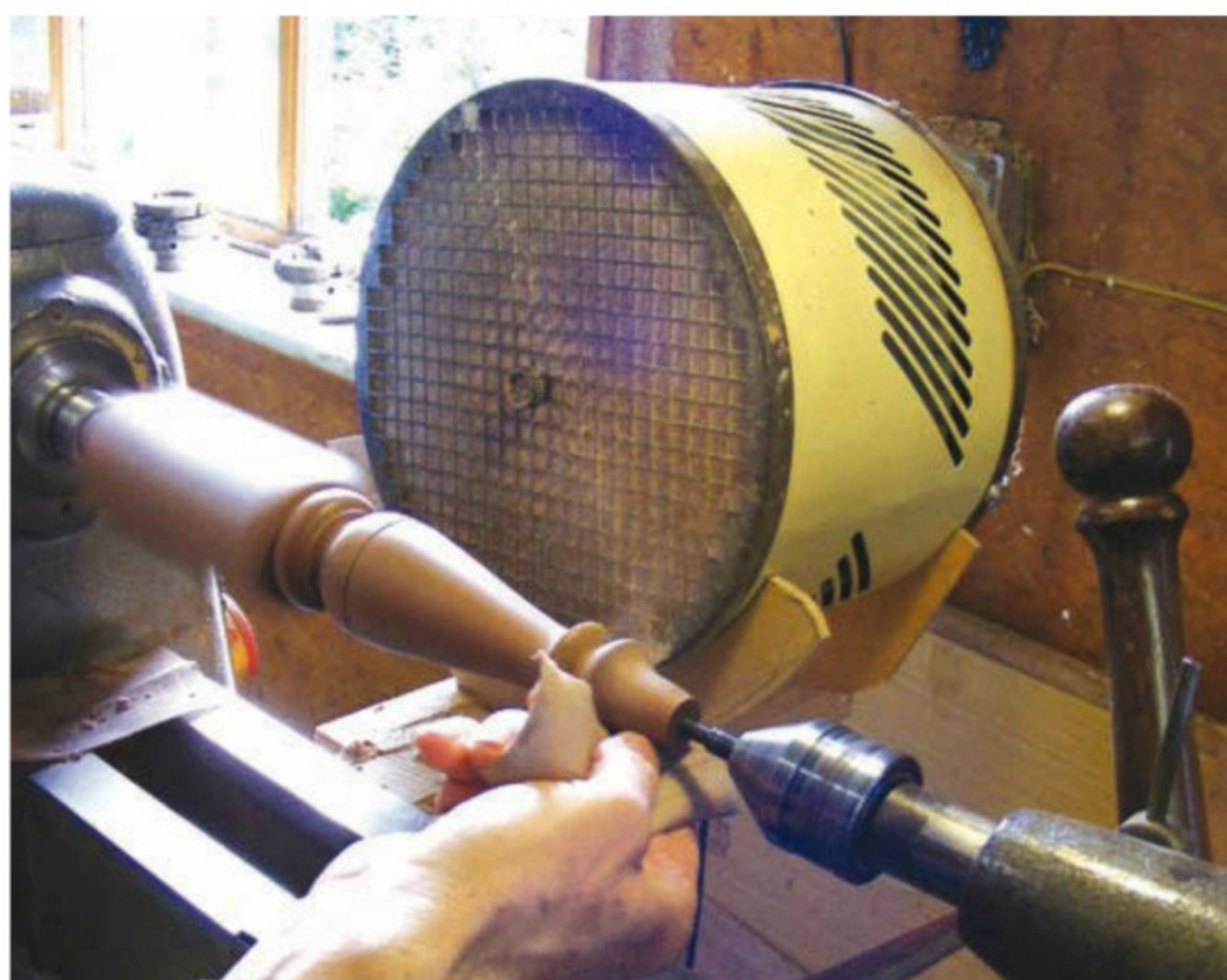
Pic.2 A fan-filter really helps to keep the dust down
