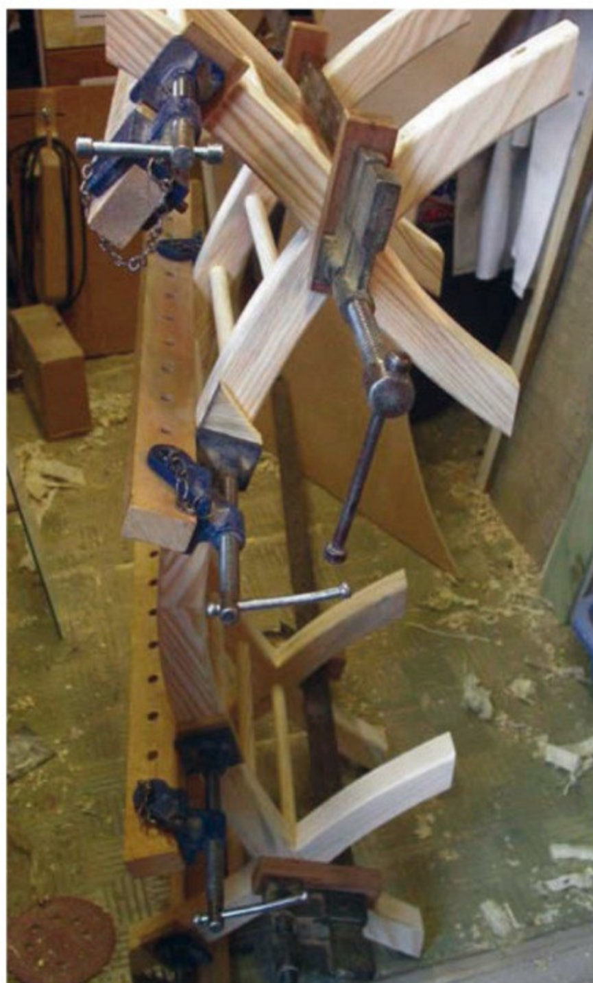
Pic.4 Joining the two frames with the turned stretchers is very fiddly. This attempt (left) failed and Bill had to fix the pieces to a board to keep it all true
