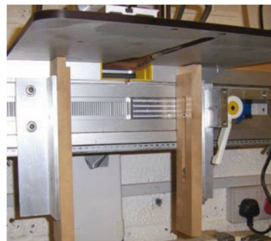
WoodRat mods Tony Sutton has added aluminium jaws to his WoodRat to make it stronger for cutting tenons. The MDF facings can be moved up and down
