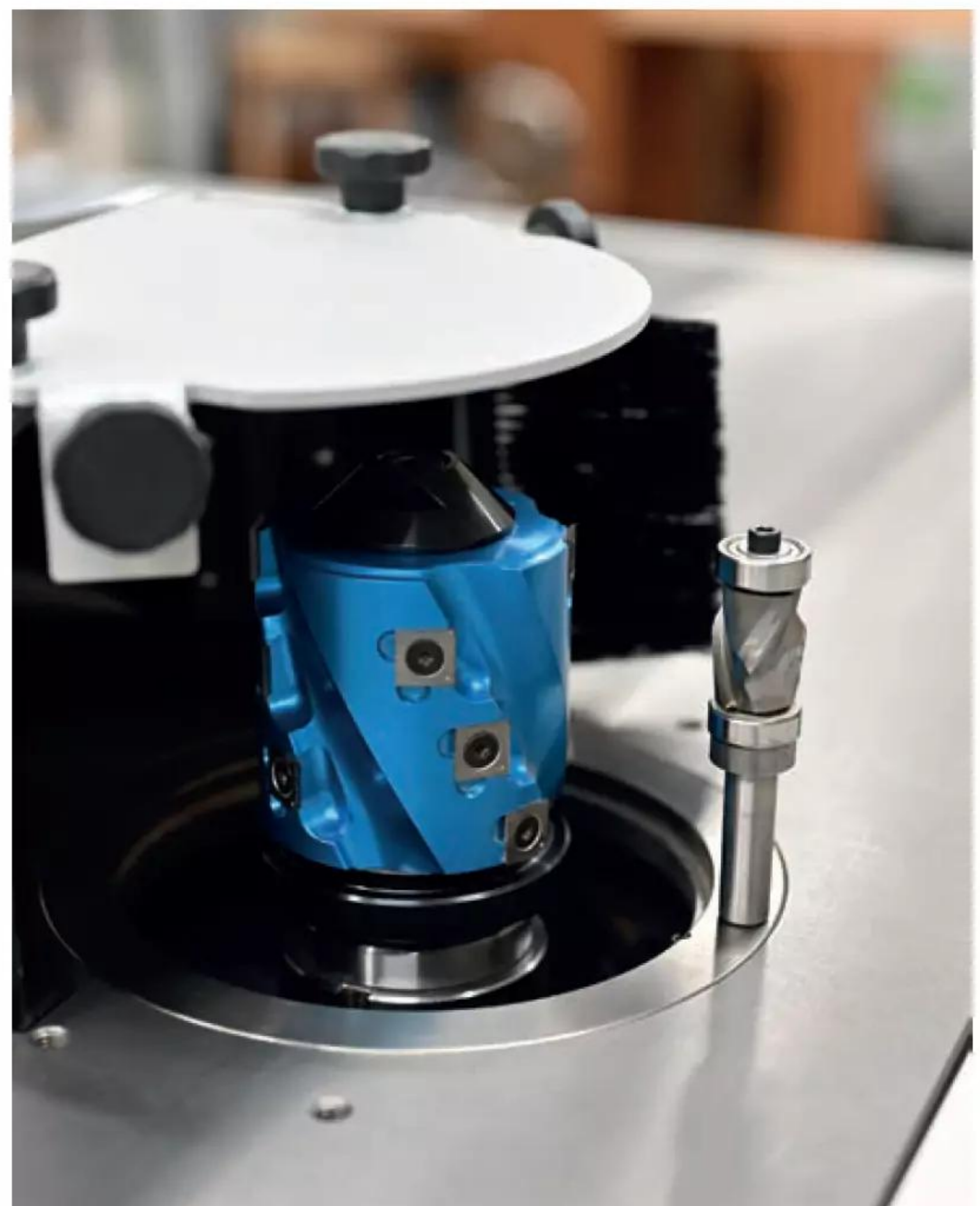
Above: An 80mm bearing guided spiral block vs 21mm spiral router bit – no contest.
