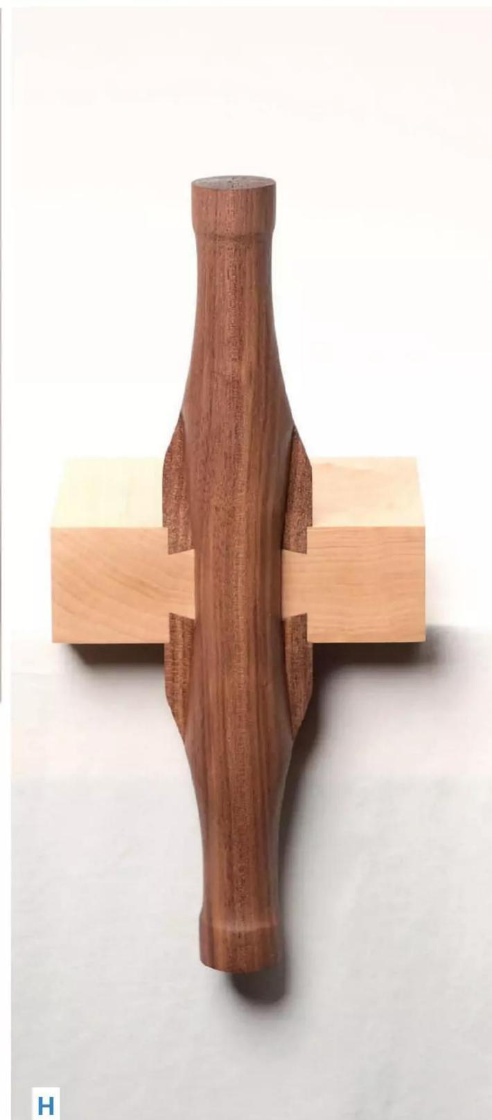
Now I need to cut a slot in the leg that's pretty close to my inner diameter. I do this on the lathe. The width of the slot for me is just wide enough to get my dovetail bit into the slot safely (B). I then take the leg back to the router table. I'll raise my dovetail bit incrementally to define my inner diameter. Then, using stop blocks again, I cut the dovetail angle in
