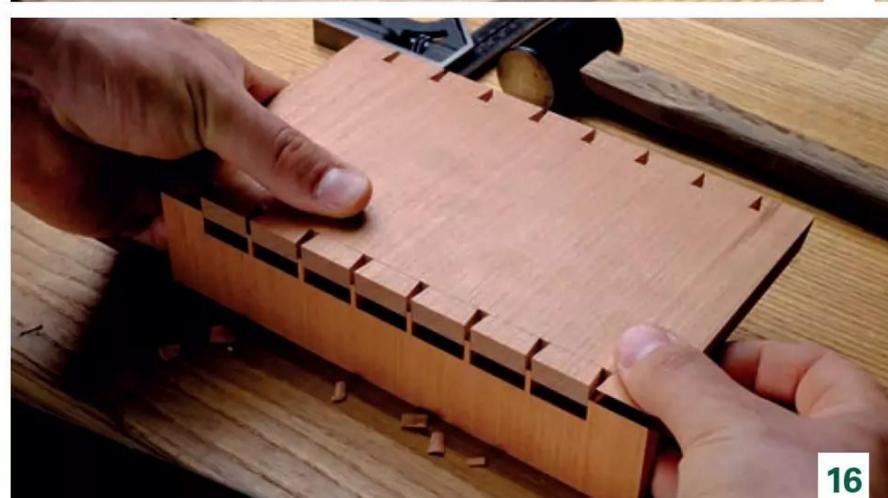
the row with half a tail. It's important to transfer the tails on the pin boards before any mitring occurs.
