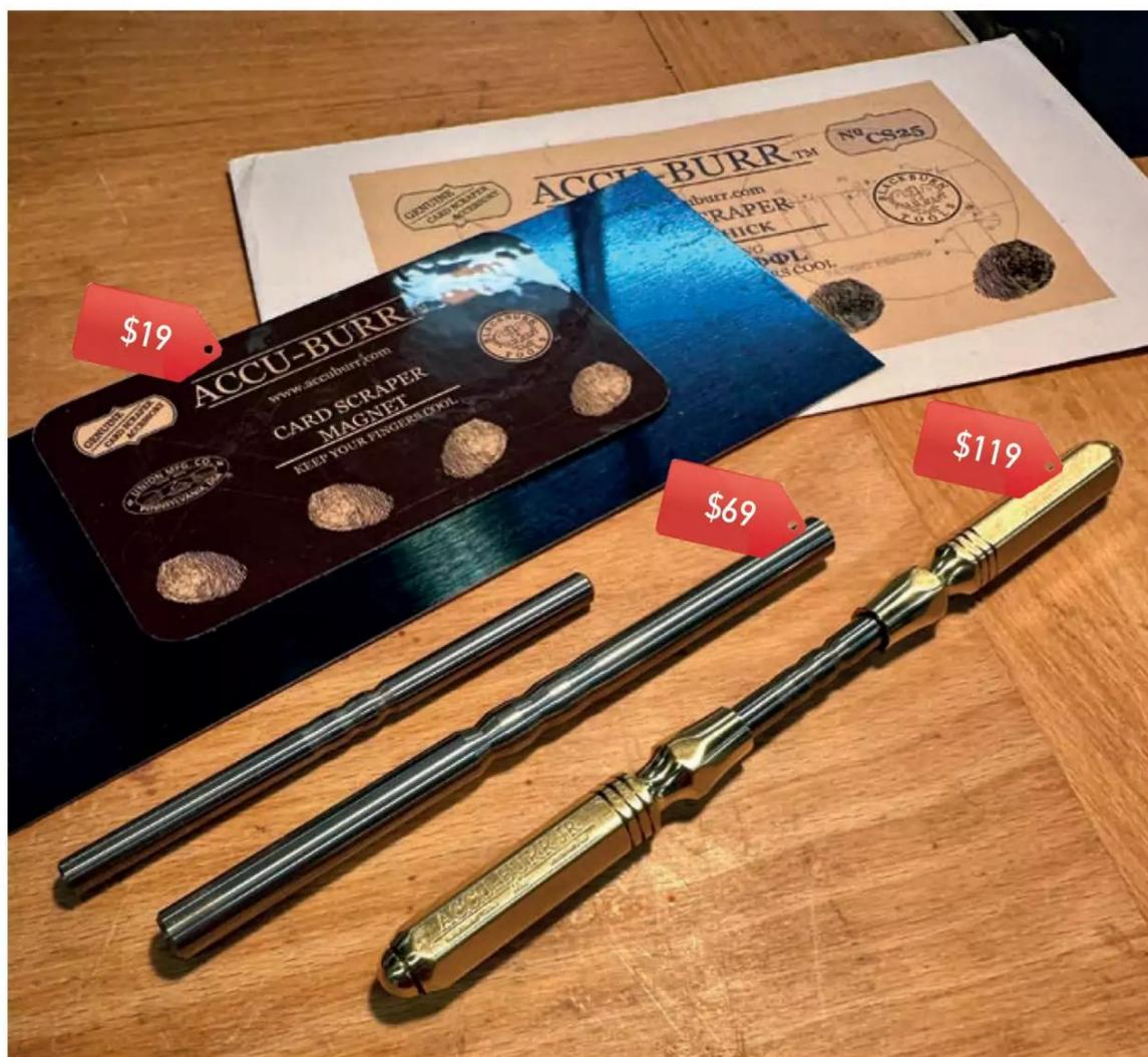
**Above:** Accu-Burr card scrapers come with a magnetic card which can be used to minimise heat transfer. The burnishing rods have three angled grooves and come with or without brass handles.
