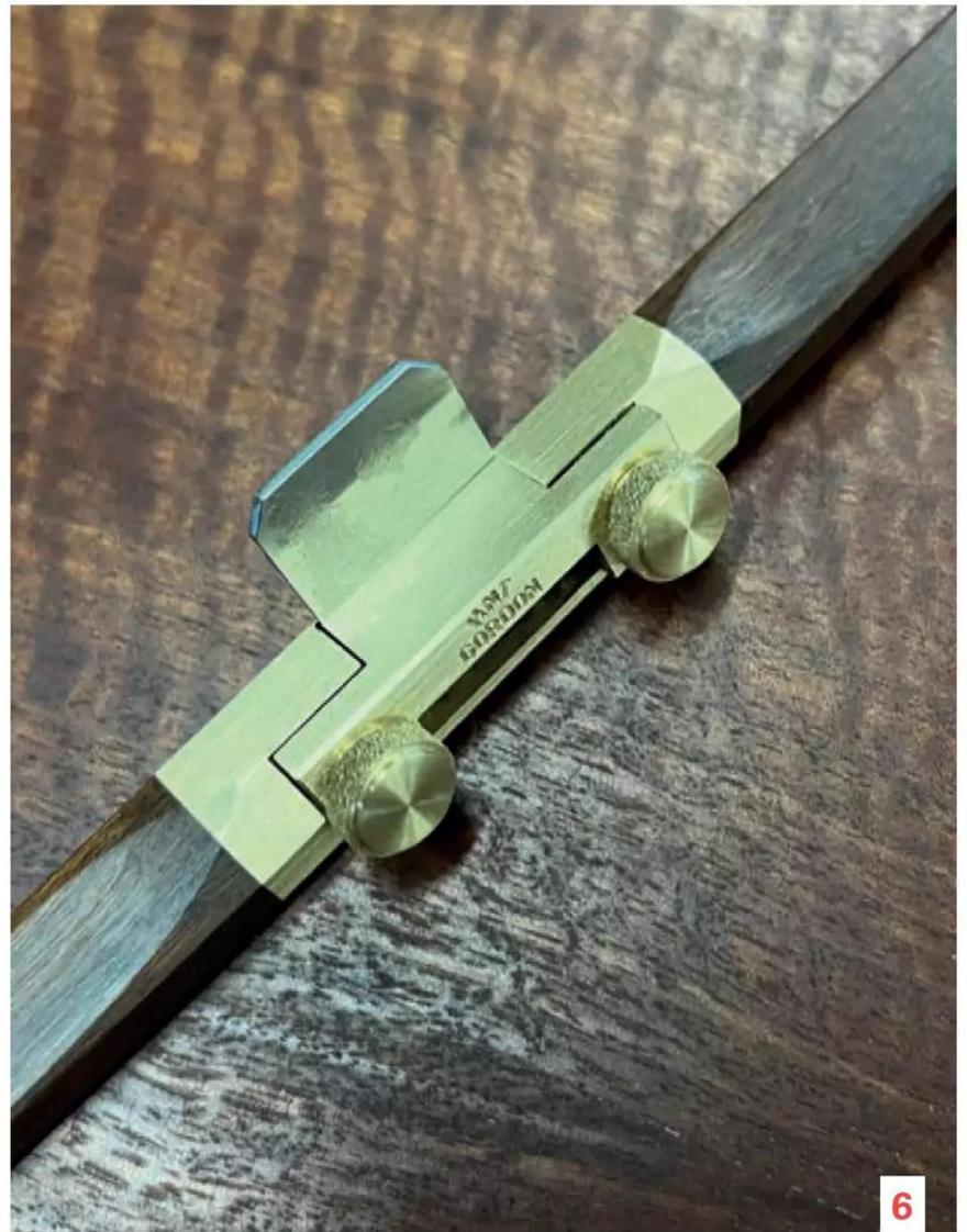
depth adjustment and the ability to skew the blade.
