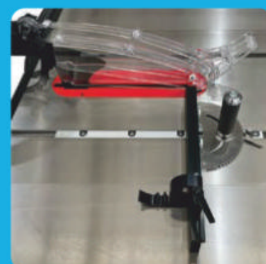
Clear blade guard with dust extraction channel
