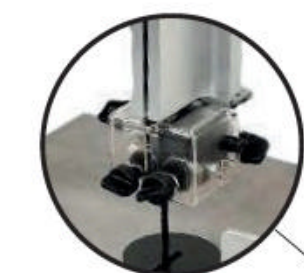
Tool-Less Spring-Loaded Blade Guides
