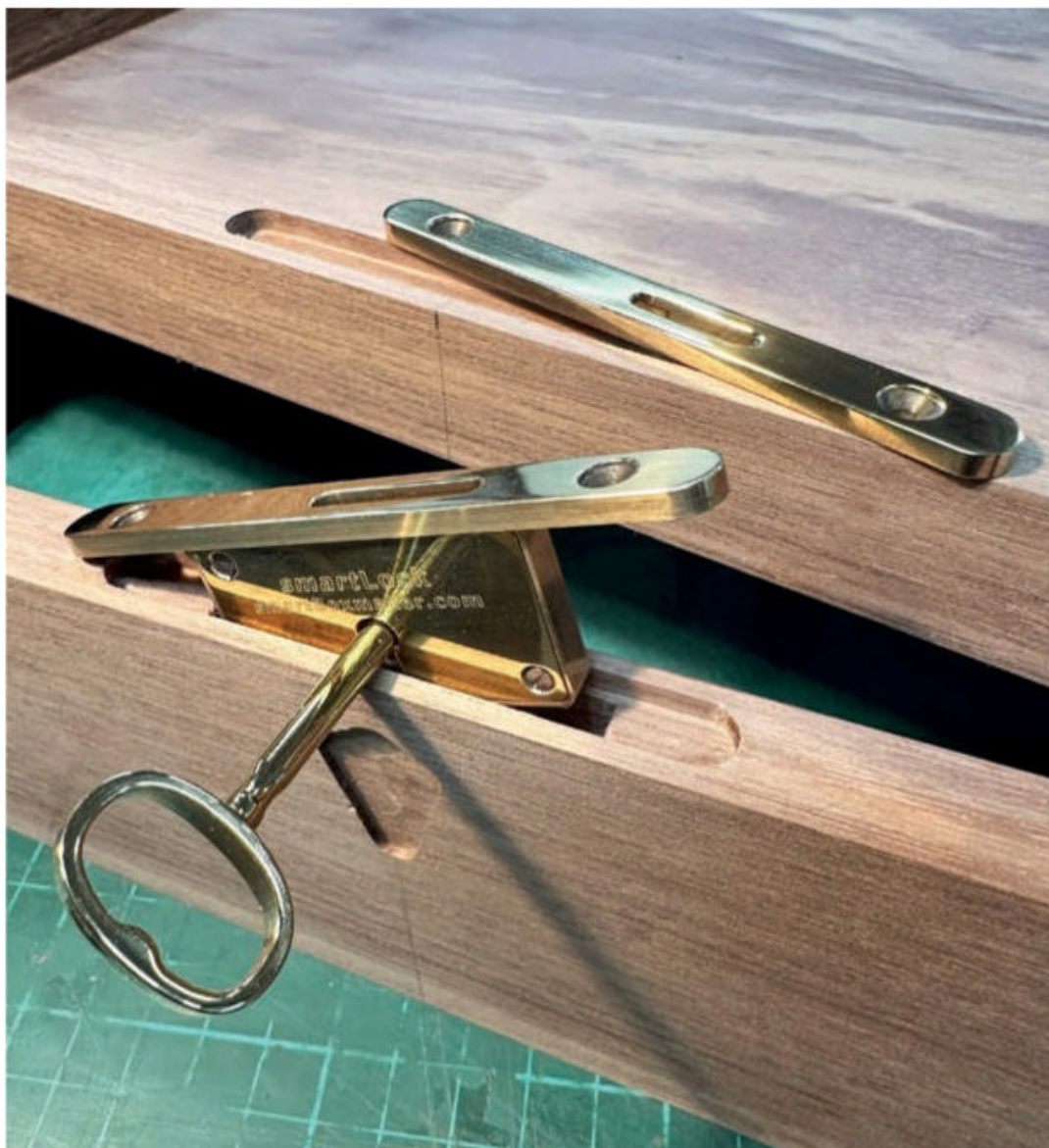
Above: The smartlock now locks and unlocks with a 90° turn of the key and performs flawlessly. Opposite: interior and outer views of installed smartButt and smartHinge hingeware.
