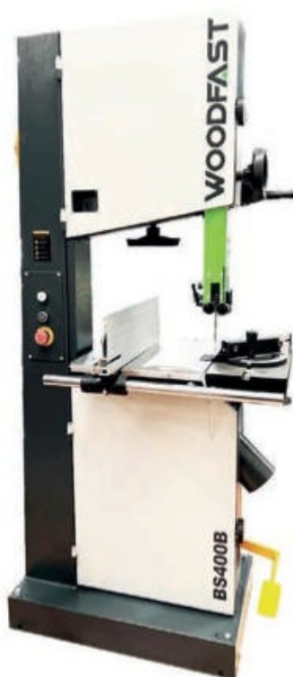
BS400B 400mm (16") Bandsaw Tilttable 2HP 240V
