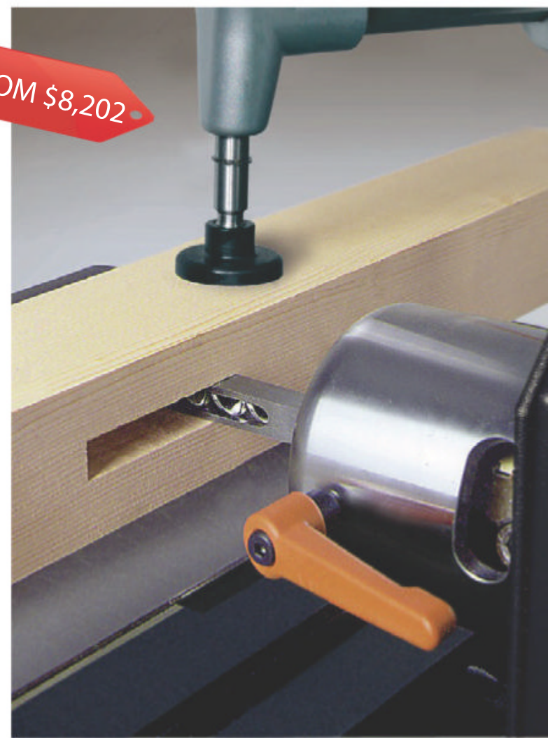
Above: Showing the FD250 mortiser in action. This is a versatile machine which can also be used for many drilling and boring processes.
