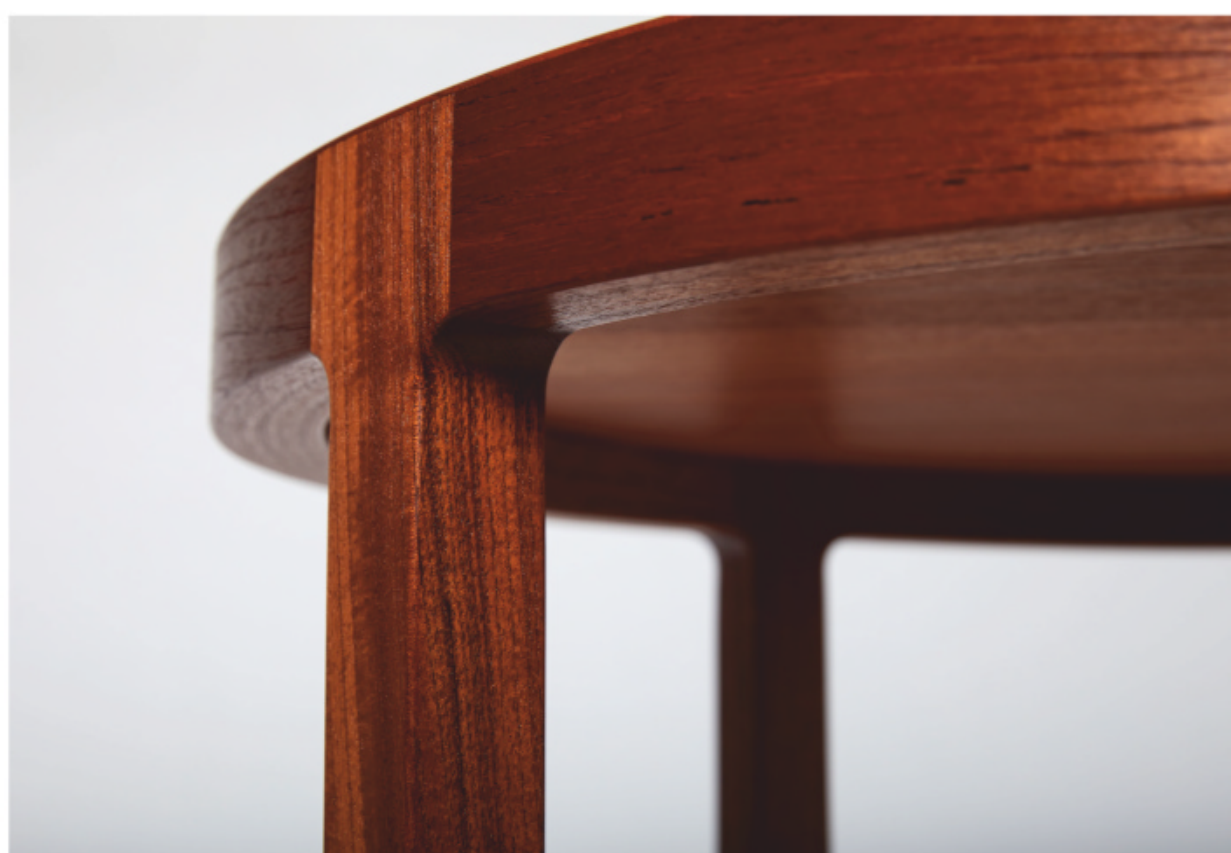
Left and below: Rolf Barfoed's Round Table in Australian red cedar features a resawn veneer top, a ring laminated rim and bridle joints.
