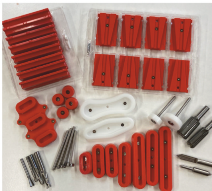
Left: The kit includes templates for box joints, dovetails, triple mortise and tenons, dowels, bowties and diamonds, 'monster' mortise and tenon guide bearings and bits as well as standard bits, guide bearings, mortise and tenon templates and centring jigs.
