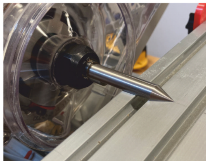
Below right: Close up to the split-shaft centring jig.
