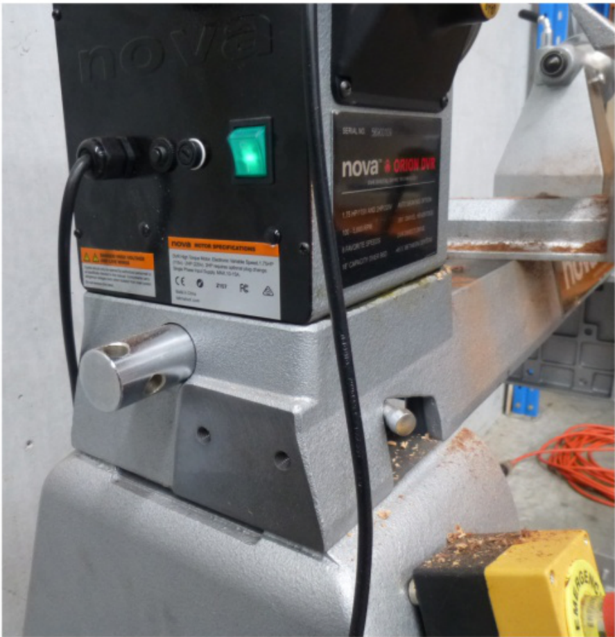
Above: Swivelling the headstock enables greater access for faceplate work and turning of larger pieces. The solid bed, saddle and toolrest provide plenty of support for outboard turning.
