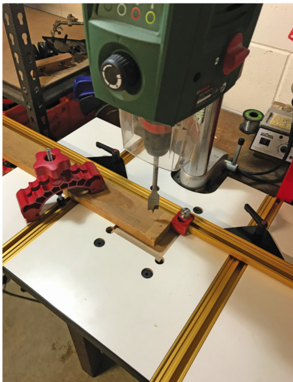
Above: The Prodrill Press Table kit comes with with fixings, clamps, flip stops and sacrificial inserts. The metric scales are not shown but fit over the T-tracks and fence.
