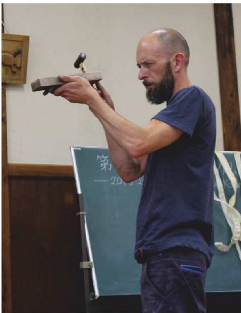
Top to bottom: Piotr Domanski sets the blade with a few hammer taps. Photo: Yuko Morita
