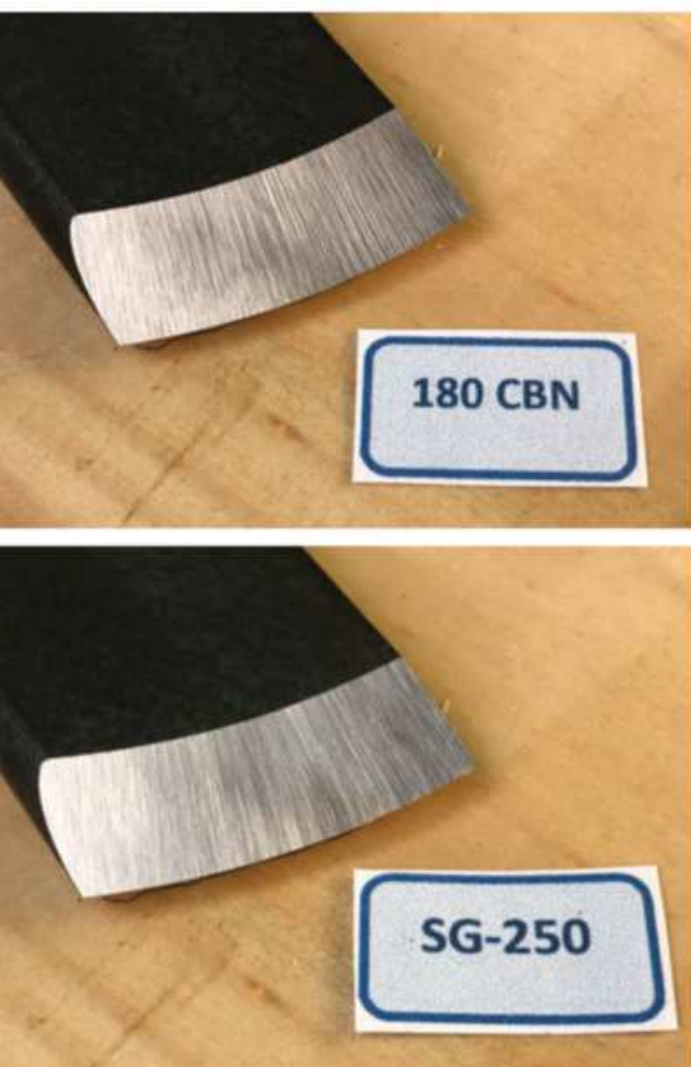
Above: Comparing grinds for the standard SG-250 and CBN wheels.
