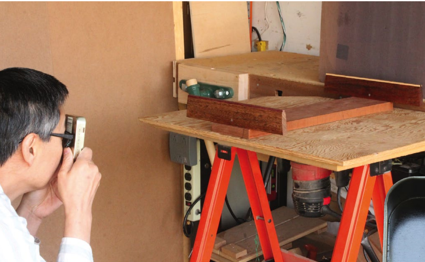
Left: Pick a contrasting background and sight at about an arm’s length from the rear stick.
