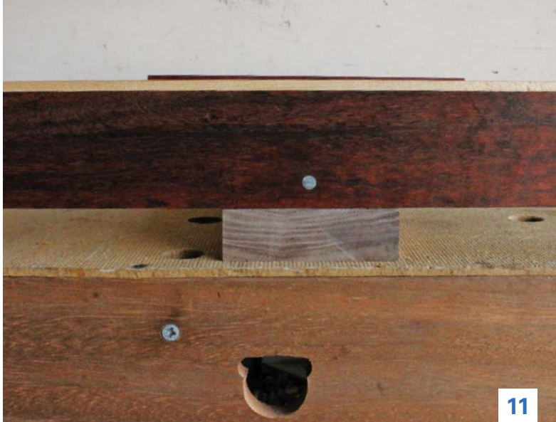
11. If the top edges of the sticks do not line up, the board is in wind.
