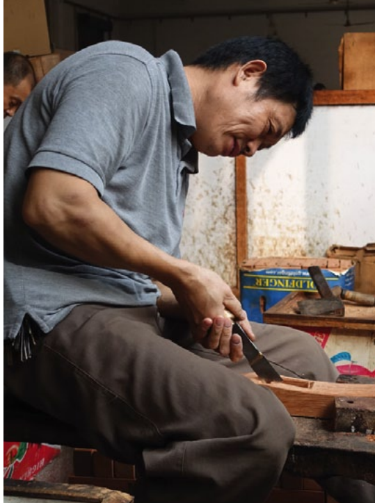
Clockwise from far left : Fitting brass wear strips into the plane bases is done by hand and by eye.
