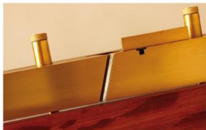
From top: HNT Gordon moving fillister plane in bull oak. The plane features beautifully machined brass fittings and fixtures. Detail of the mouth and blade.
