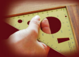
CHECK YOUR JOINTS ARE SQUARE
