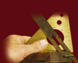
USE THE PROTRACTOR TO SET BEVELS
