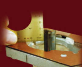
SET DEPTH OF ROUTER CUTTERS
