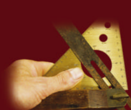
USE THE PROTRACTOR TO SET BEVELS
