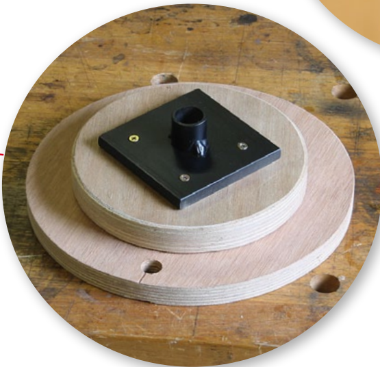
Pressure plates made from marine ply with flat steel / tube for locating rods
