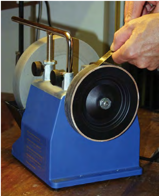
Left: The stone grader easily converts the grindstone from coarse 220 to fine 1000 grit. Above: Hand held stropping with the leather wheel leaves a razor sharp edge.
