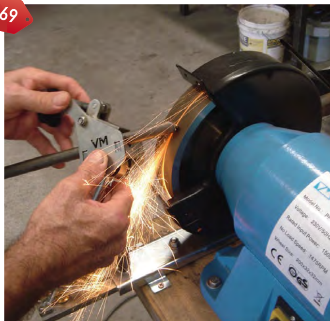
Above: Vicmarc grinding system. Shaping the tool on the coarse wheel.
