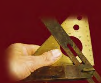
USE THE PROTRACTOR TO SET BEVELS
