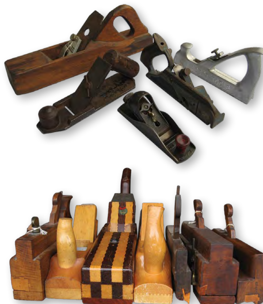
Bottom: Showing the interesting variations of boxwood inserts attached to some plane soles.
