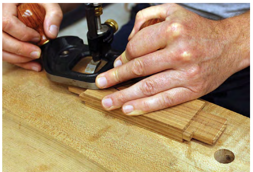
Above: Using a router plane to trim the tenon cheeks.
