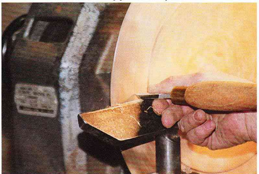
2. (above) Starting to cut the dovetailed spigot. 4: (below) Cutting grooves on a platter rim.
