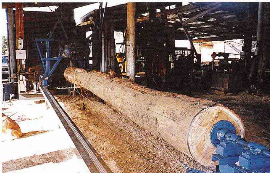
Silvertop ash set in the "dog" used to hold the log
