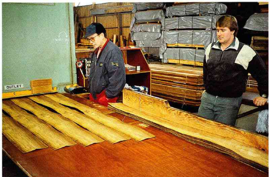
Top and above Slicing and drying veneer at Britton Bros in Smithton, Tasmania.
