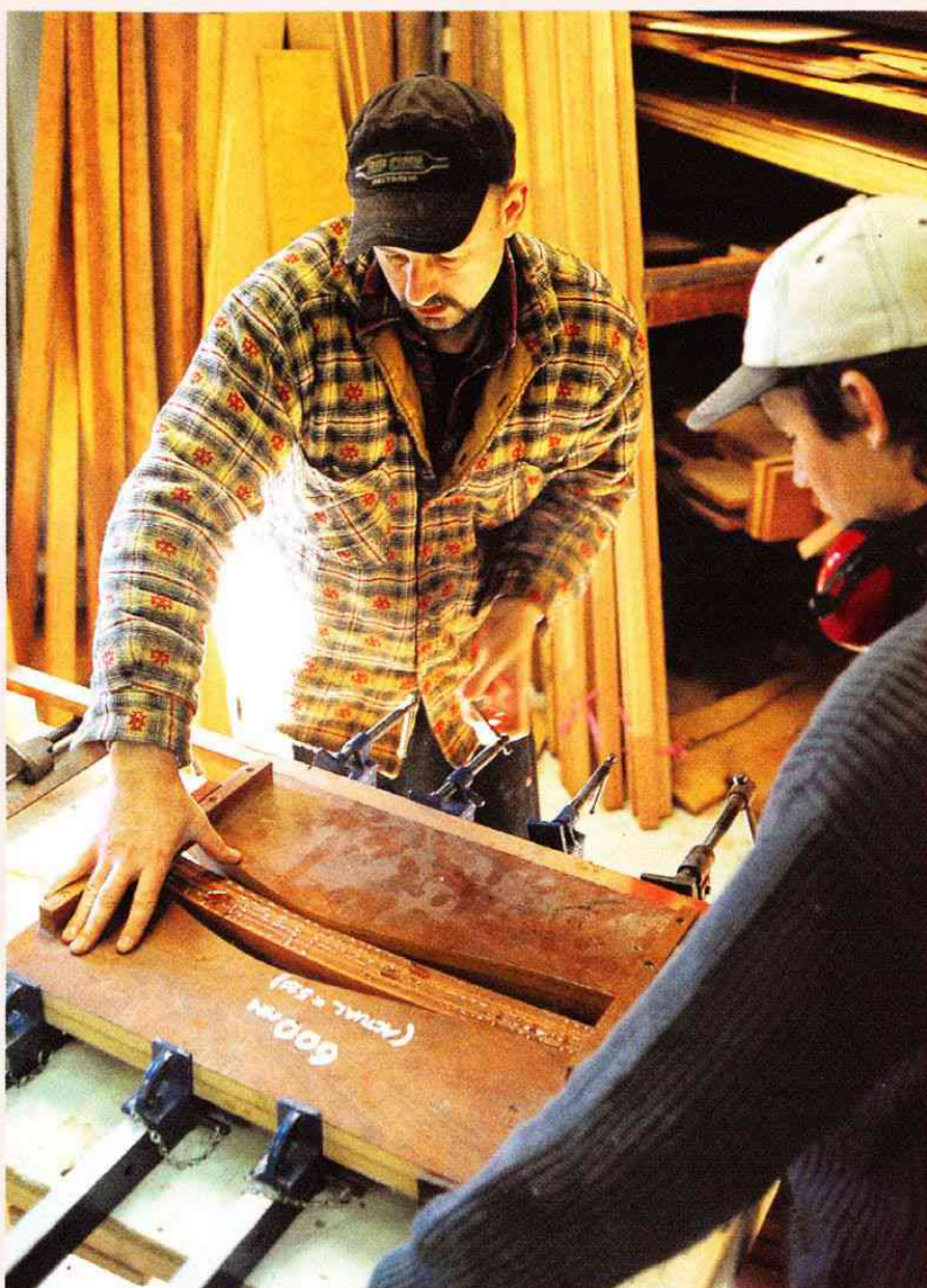
Top: Each splat is made up of two strips of wood which are glued together. Above: Sets of splats are clamped between the shaped blocks.
