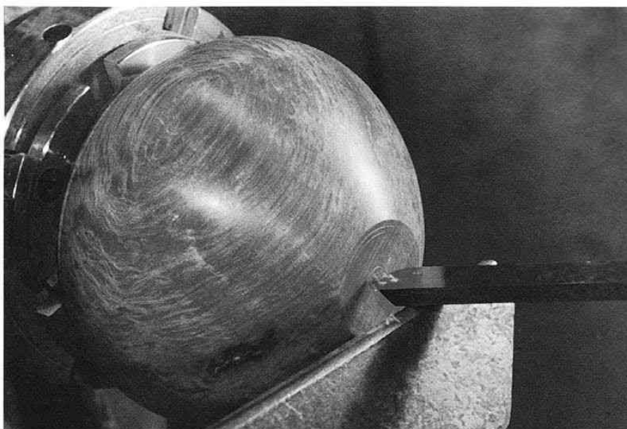
8. Cutting fine grooves in the foot.
