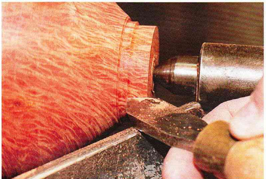
2. (above) Starting to cut the dovetailed spigot. 4: (below) Cutting grooves on a platter rim.
