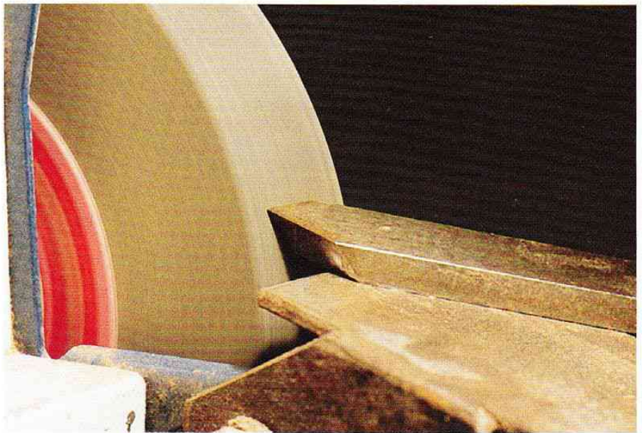
1. Grinding the diamond-point scraper on the flat tool rest.
