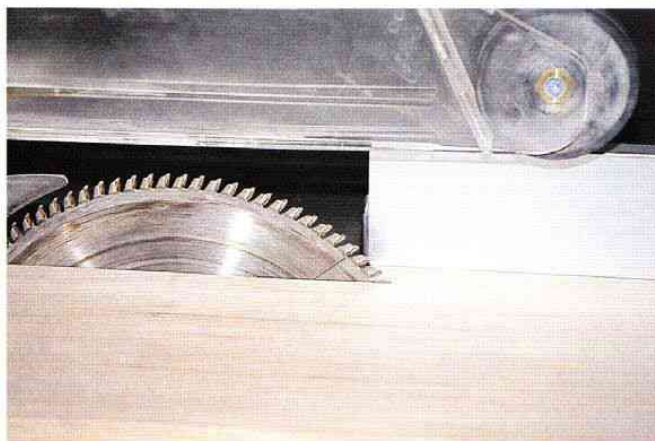
Setting the rip fence to the saw gullet for solid timber cutting.
