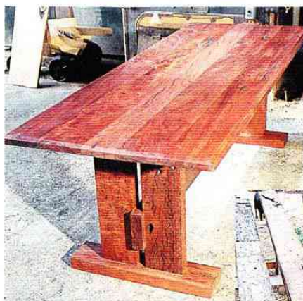
The redgum table above was made from the beams shown right by A.Y. Woodworks in Victoria. Apart from all the tar, bolt and nail holes, the volume of usable timber was greatly reduced by the amount of gum vein and feature present.
