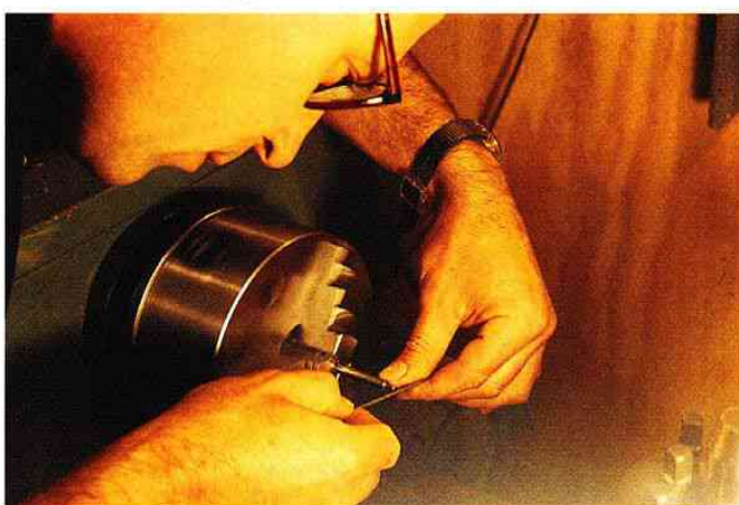
Left: Polishing the pivots. Pivots are made from hardened steel and polished to a mirror finish to minimise friction. Right: Drilling and boring the centre hole of a completed wheel. My woodturning chuck (Vicmarc 140) has been adapted for use on my metal lathe. The chuck has been fitted with MDF 'soft jaws' which have been turned with a rebate to suit the wheel diameter. The wheel can now be accurately centred and drilled.
