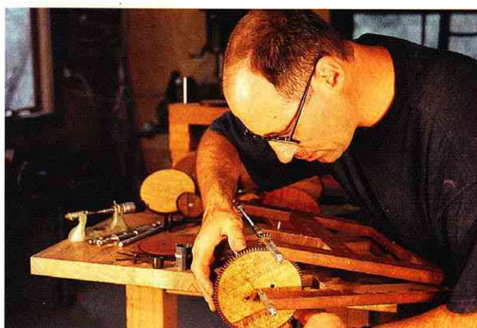
Left: Machining a batch of wheel blanks on the milling machine. The compound table traverses the rotating cutter from left to right. The rotary table with the indexing plate is rotated a tooth width before commencing the next cut. Right: Checking the mesh of a wheel and pinion on a homemade depthing tool. The depth of mesh is critical and ensures the smooth running of the wheel train. The distance between centres is then directly transferred to the clock plates.
