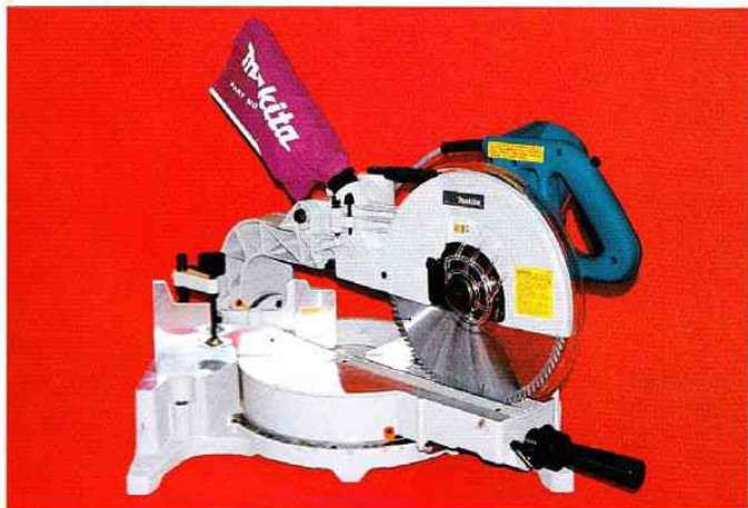
Makita LS1212, 305mm 100-tooth sawblade, made in Japan, $1385, 1650 watt, compounds left and right, dust bag, crosscut capacity at 90°: 310mm x 98mm, at 45°: 220mm x 98mm.
