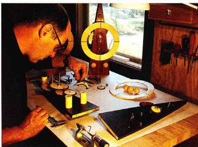
Left: The completed wheel assemblies are assembled on the clock plates. Right: The top clockplate and dial are fitted.
