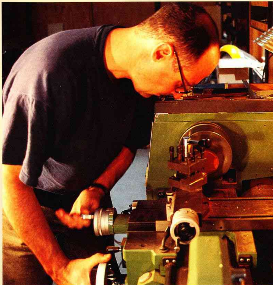
Truing up some wheel blanks on the lathe.
