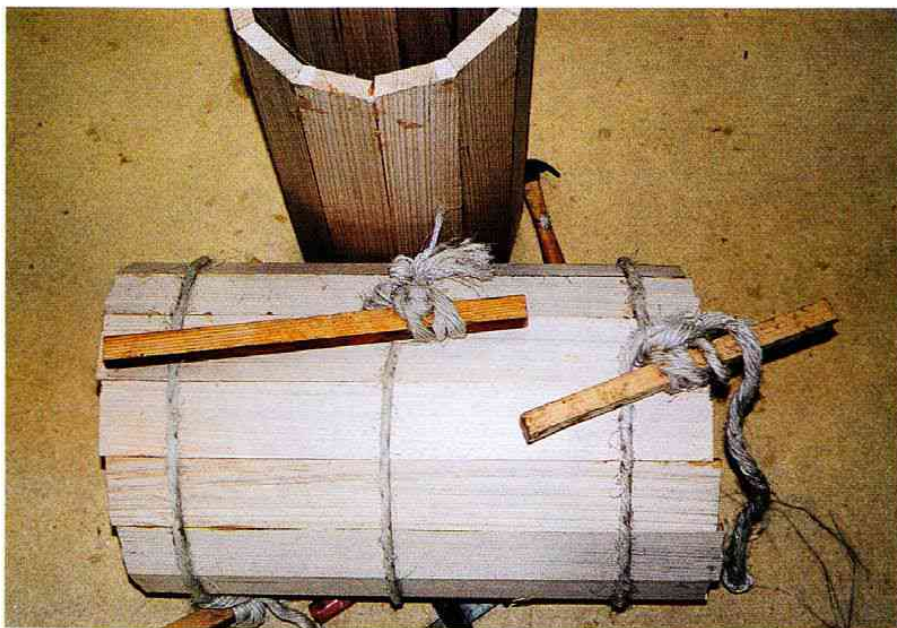
Commercial belt clamps are available, however twisting rope around with the aid of small sections of timber worked effectively.
