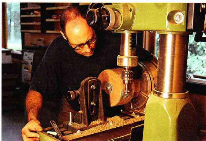
Left: Machining a batch of wheel blanks on the milling machine. The compound table traverses the rotating cutter from left to right. The rotary table with the indexing plate is rotated a tooth width before commencing the next cut. Right: Checking the mesh of a wheel and pinion on a homemade depthing tool. The depth of mesh is critical and ensures the smooth running of the wheel train. The distance between centres is then directly transferred to the clock plates.
