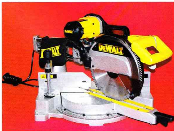
DeWalt DW708, 305mm 60-tooth blade, made in USA, $1349, 1500 watt, compounds left and right, dust bag, crosscut capacity at 90°: 305mm x 114mm, at 45°: 218mm x 114mm.
