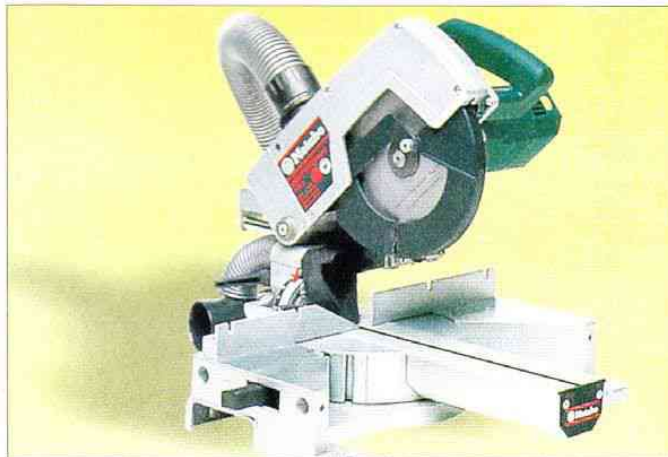
Metabo, KGS E1670, 210mm blade, made in Germany, $1136, 1600watt, compounds one way only, dust outlets, crosscut capacity at 90°: 270mm x 52mm, at 45°: 184mm x 52mm, belt drive.
