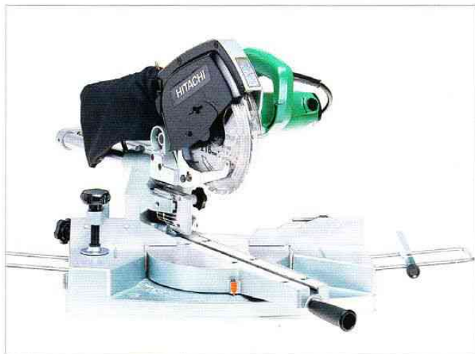
Hitachi C8FB2, 216mm 60-tooth blade, made in Japan, $859, 1370 watt, compounds left and right, dust bag, crosscut capacity at 90°: 305mm x 75mm, at 45°: 220mm x 75mm.
