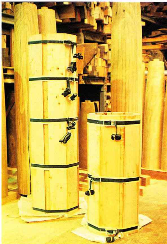
Left: Laminated drums for a pattern for columns to be cast in imitation sandstone by Haddonstone Australia Pty Ltd. Right: A 7-metre-long central column for a pole house being turned to the client's design.
