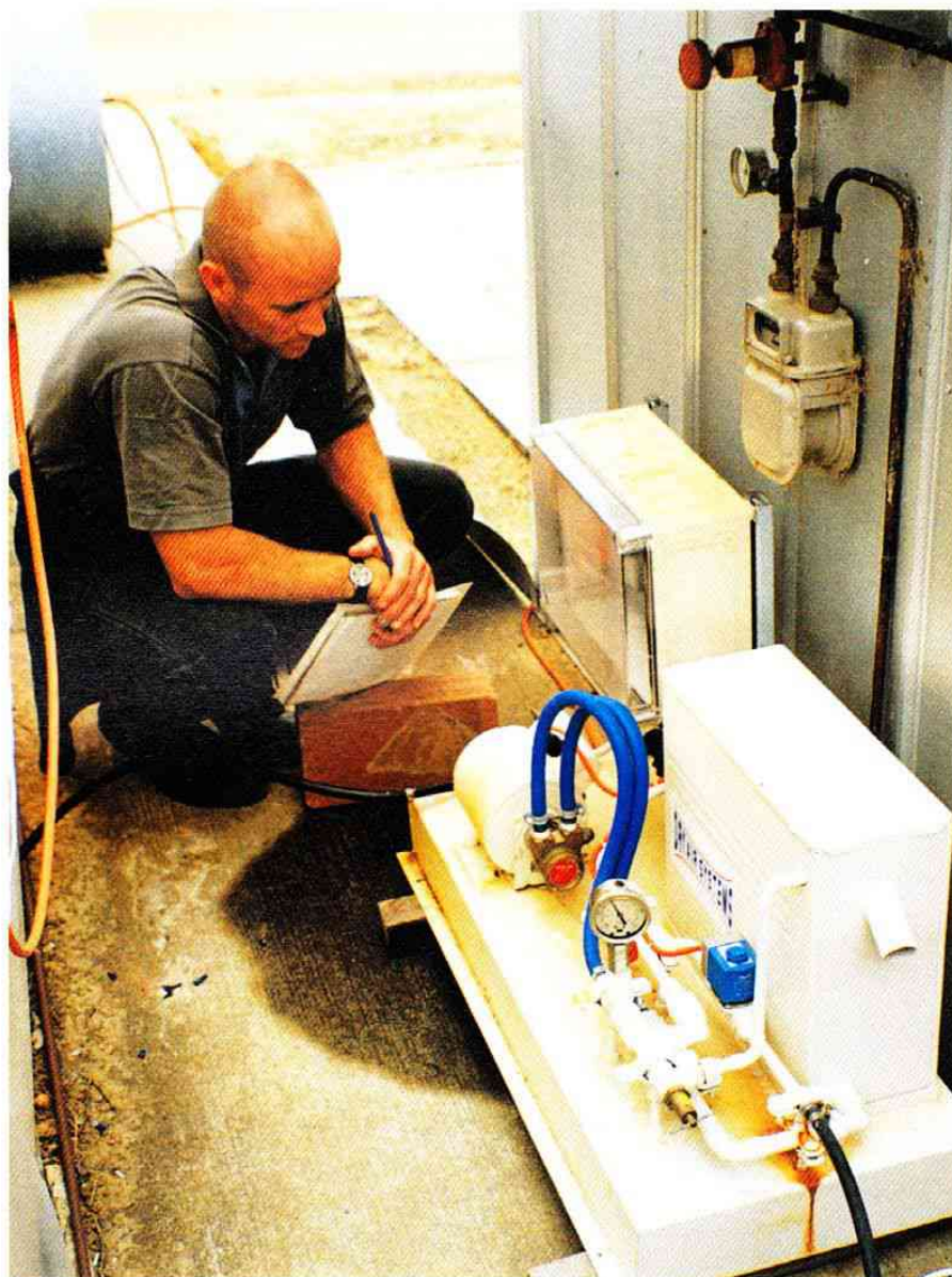
Technical officer Peter Hill with experimental unit for controlling switching and water pressure for foggers (humidifiers) on one of the solar kilns.
