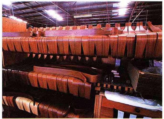
After baking, the laminated plyformed shells are cut and shaped into the required components.
