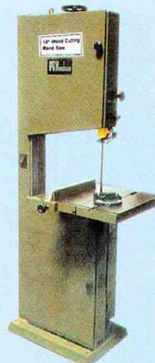
Woodman BA218W bandsaw. Features 1.5hp motor, 458 x 483mm tilting table (45°), mitre fence, rack & pinion top guide assembly, cut height 11".
