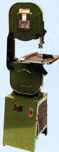
The Haeco range have tables 14", 16" and 18" square and 22.5x28.5", 24" x 28.5". Cutting height capacity from 5.5" up to 12".
