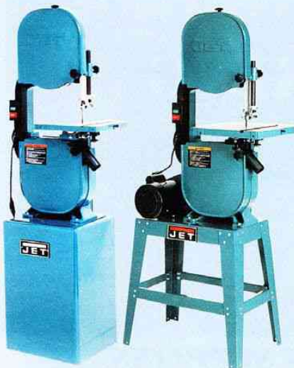
Jet bandsaws JWBS14CS (1hp) and JWBS140S (0.75hp). 15" square tables, 45° x 10° tilt, 6" cut height, heavy duty cast alloy wheels, 2 year warranty.
