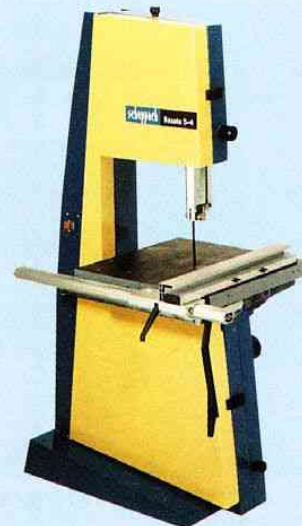
Scheppach, table size 640 x 640mm, four speeds, cut height max. 300mm, tilt -20°—+45°, overall height 1850, width of cut max. 440mm.
