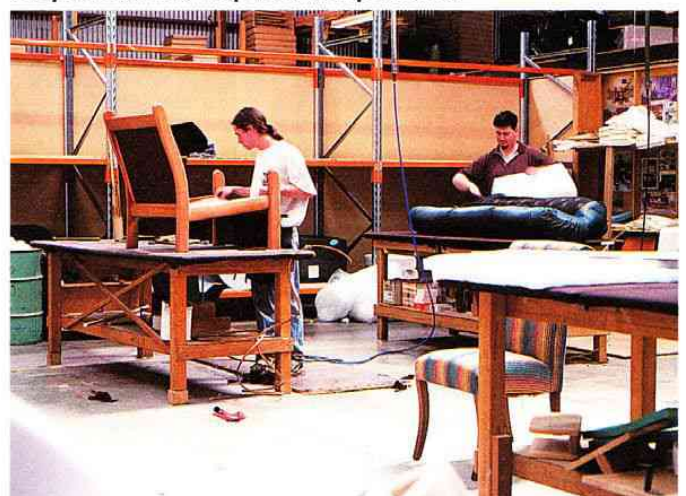
Webbing and padding is stapled to the assembled and polished chair and lounge frames.
