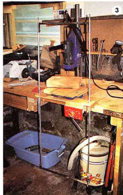
A foot extension on the drill press frees the hands.
