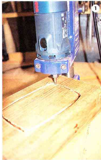
Hollowing out the interior of the box.
