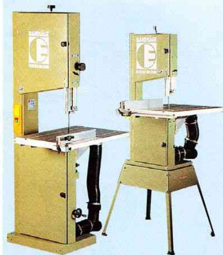
Elektra Beckum BAS 350 has 688 x 550mm table and 170mm cut height. BAS 500 table is 772 x 550mm, cut height 300mm. 45° tilt on both.
