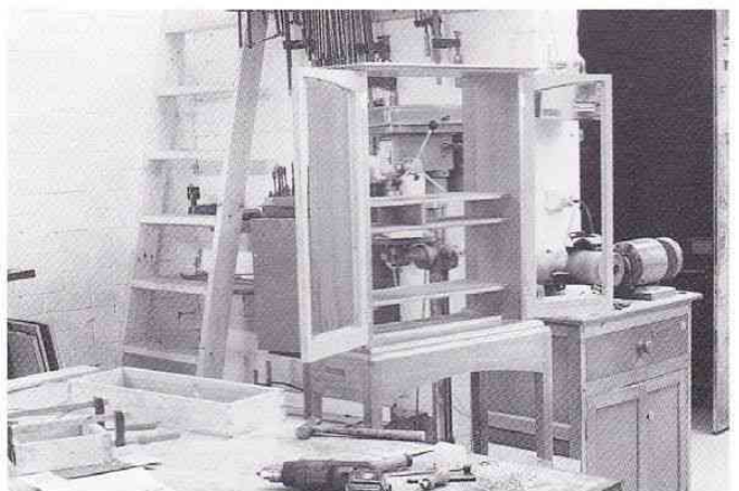
Hanging the doors on the near-completed carcass and base.
