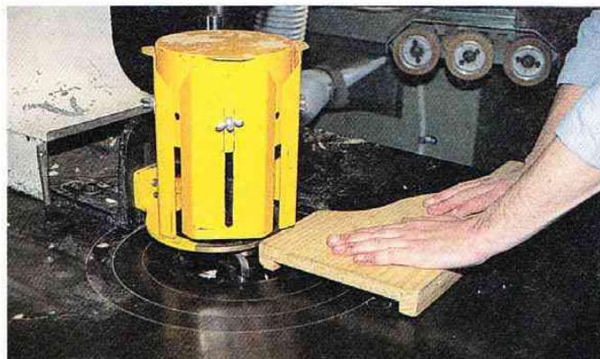
A ring fence operation using a jig, which is always preferable.
