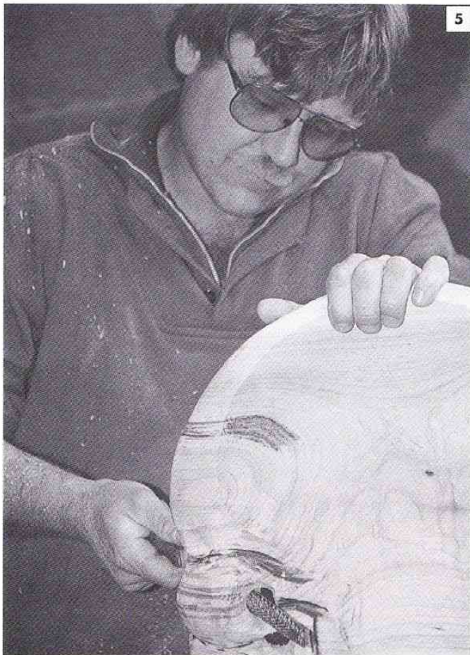
Smoothing the holes with a rasp.
