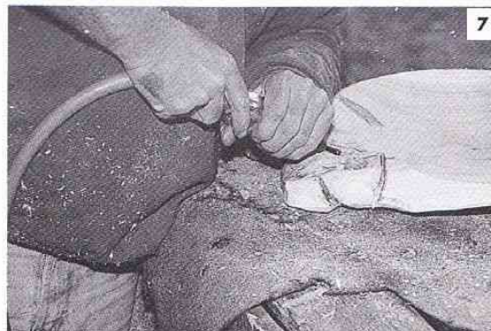
Refining the design with a burr in an air-powered die grinder.
