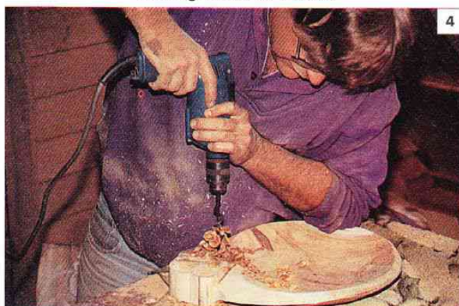
Drilling out the waste.
