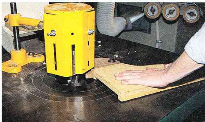
Starting a ball race operation. The work is held in a jig which fits over the workpiece. The part is first supported by the 'lead-in' piece seen bolted to the table. A bonnet guard must be used and, as usual, the hands held flat.
