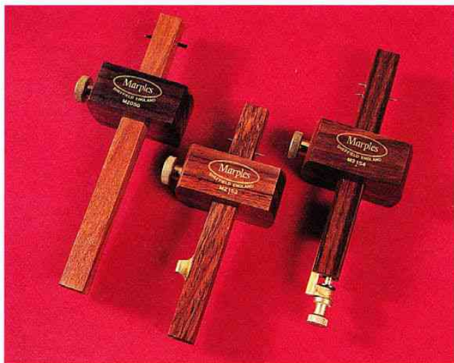
Marples M2050, $33, polished hardwood, steel pin sharp, end of beam a bit rough, brass screw, brass wear plates on stock neatly fitted but pins slightly proud, beam and stock fit OK, can be squared.
