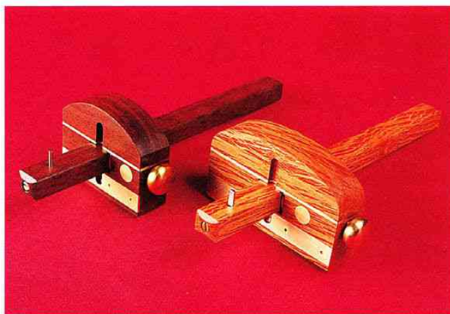
Left above: Colen Clenton marking gauge, $98, polished hardwood, hand made and detailed, HSS pin sharp, all edges fine sanded, brass screw would be better knurled, brass wear plates neatly fitted, fit of beam and stock good, not square. Right: Colen Clenton cutting gauge, $132, polished hardwood, hand made and detailed, HSS steel cutter sharp, all edges fine sanded, brass screw would be better knurled, brass wear plates neatly fitted, fit of beam and stock OK, not square.
