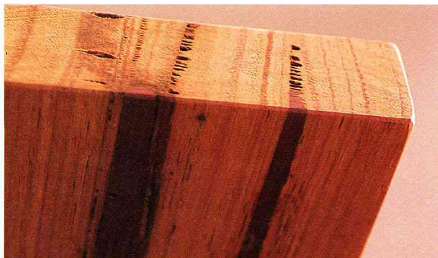
Gum vein over 3mm exposed in the ends of boards should be avoided as resulting movement can loosen fillers.
