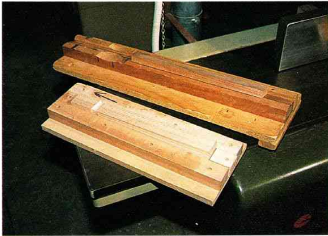
Left: Jig samples, at the front a 'box' type jig for machining a tapered leg. Direction of feed is indicated. At the rear a jig for machining bevels (bevelled beads). Note the stop at the right of the jig to stop it being fed through the machine. Wax prevents friction. Right: Use push blocks where possible—they are safer, keep you cleaner and prevent you getting splinters.
