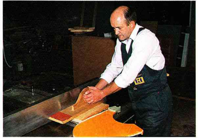
Left: Jig samples, at the front a 'box' type jig for machining a tapered leg. Direction of feed is indicated. At the rear a jig for machining bevels (bevelled beads). Note the stop at the right of the jig to stop it being fed through the machine. Wax prevents friction. Right: Use push blocks where possible—they are safer, keep you cleaner and prevent you getting splinters.
