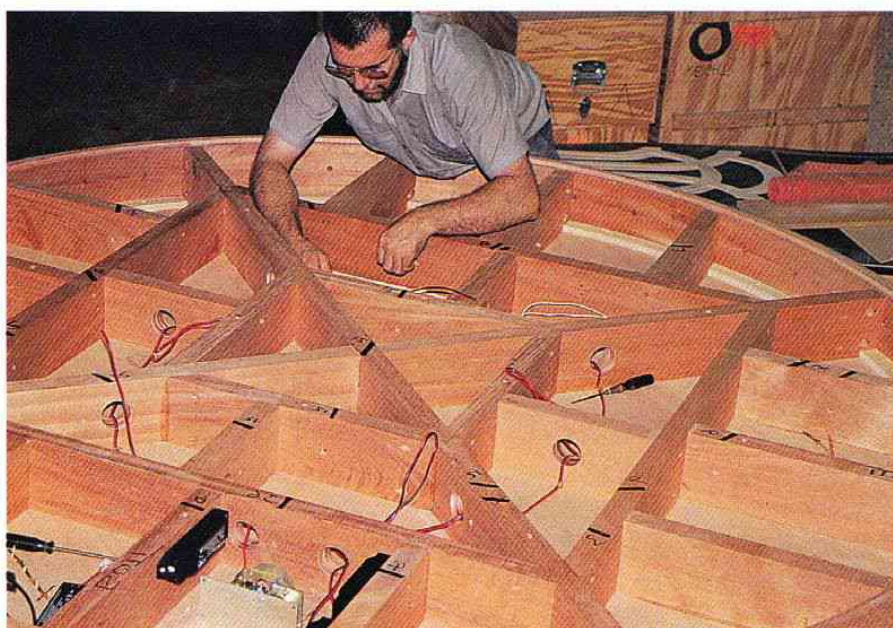
Workshop manager Nick Edgar engineers fibre optical lighting in a torsion box of labyrinthine construction.
