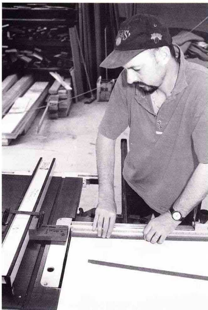
To make the 8 x 8mm tenons for the kumiko the fence of the table sawblade is set to 90°, coinciding with the top dead centre of the blade and with a stop on the other side. The workpiece is pushed into the side of the blade.
