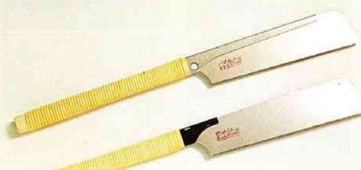
These Japanese Z-saws are a delight to use, one is a fine crosscut and the other is a super fine dovetail saw.
