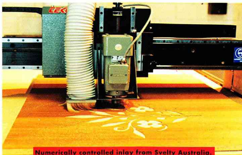
Numerically controlled inlay from Svelty Australia.
