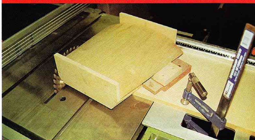
Jig for cutting chair backs: In production situations a series of complex jigs may be devised to cut irregularly shaped components such as curved chair backs. I have made two such jigs for the cutting of chair backs in a production chair that I make. First the pre-laminated backs are held and passed through the panel saw upside down in a box-like jig clamped to the sliding table, as shown here. The blade is tilted to produce a compound angle on a curved component with great accuracy. Another jig trims the top of the chair back to the correct angle, once again with the aid of a purpose-built jig clamped to the sliding table, see photo p.35.
