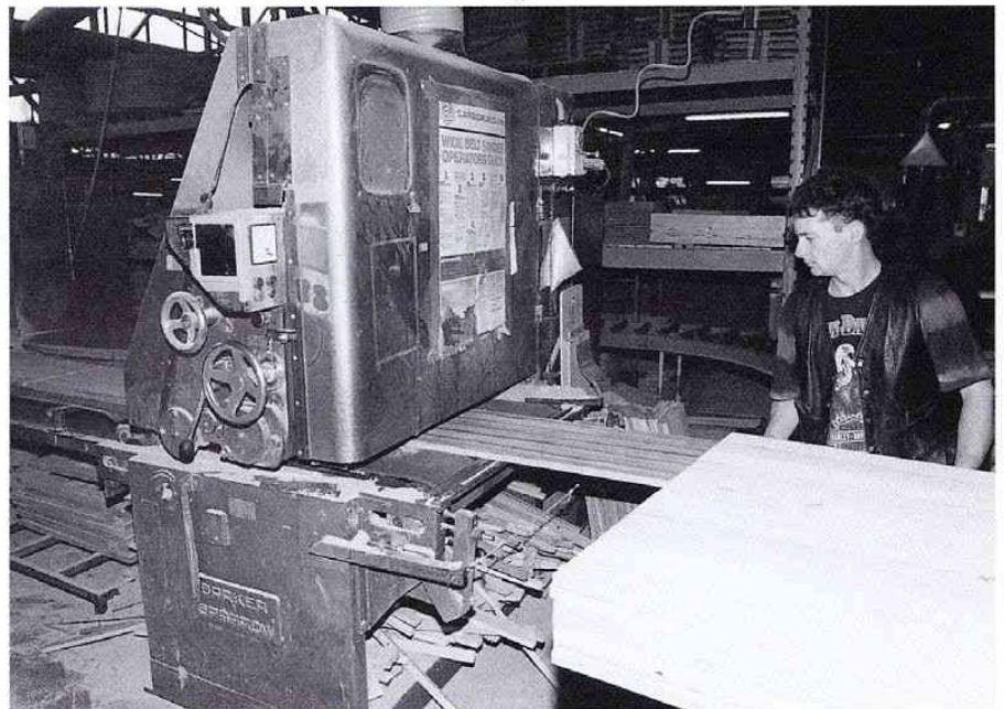
The Barker & Sparrow wide belt sander handles the abrasive native timbers.
