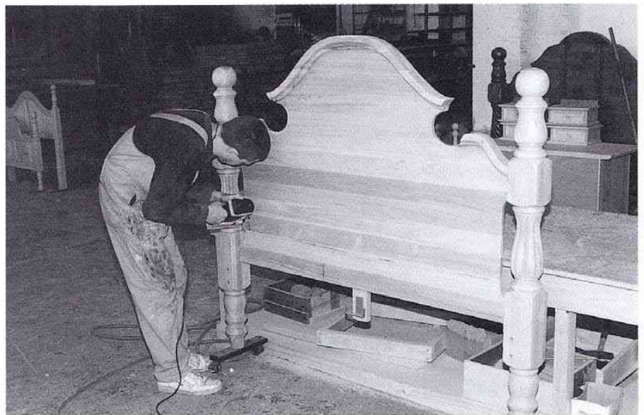
Finish sanding bedheads.
