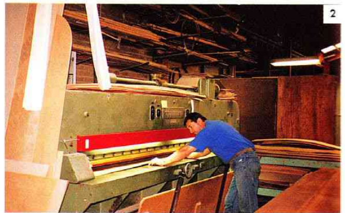
2 The guillotine cuts the whole bundle to 205mm width at once to ensure perfect joints.
