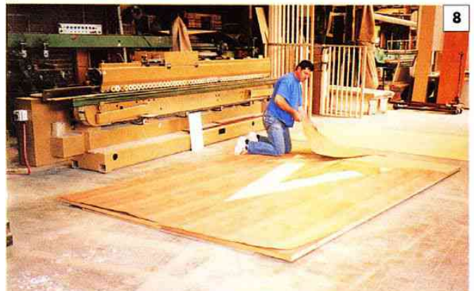
8 The sections of mahogany veneer where the star sits are cut out to be replaced with the blackbean and ash segments.
