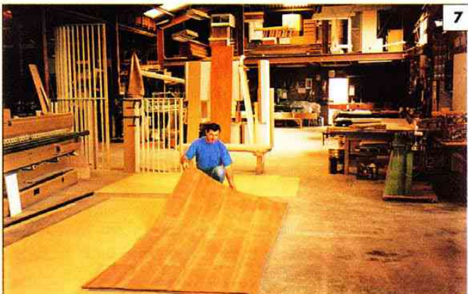
7 The table is too big to put on a workbench! After making a suitable platform the veneer is layed up on the floor.
