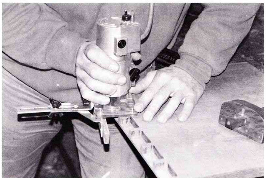
Top: Setting depth and width of cut for a butt hinge.
