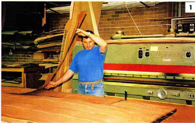
1 Checking quality and grain marking of each veneer leaf before cutting. One faulty leaf can ruin the whole layup.
