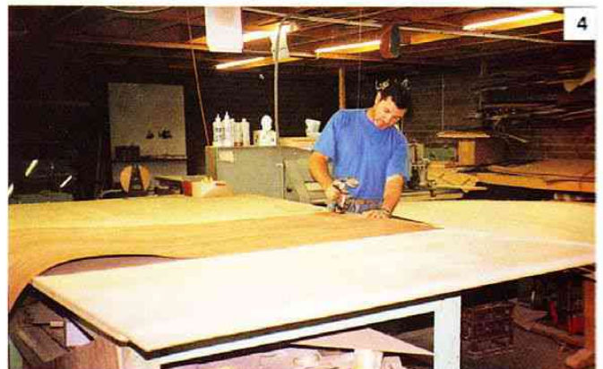
4 Veneer ends are glued across the grain to prevent splitting in the press. A small, hand-held joining machine operates on the same principle as its larger brother in photo 3.
