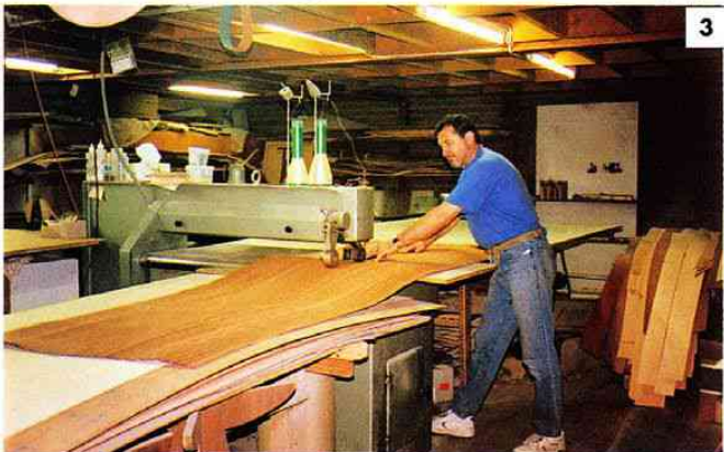
3 Our joining machine uses plastic heated thread to glue together the individual leaves perfectly.
