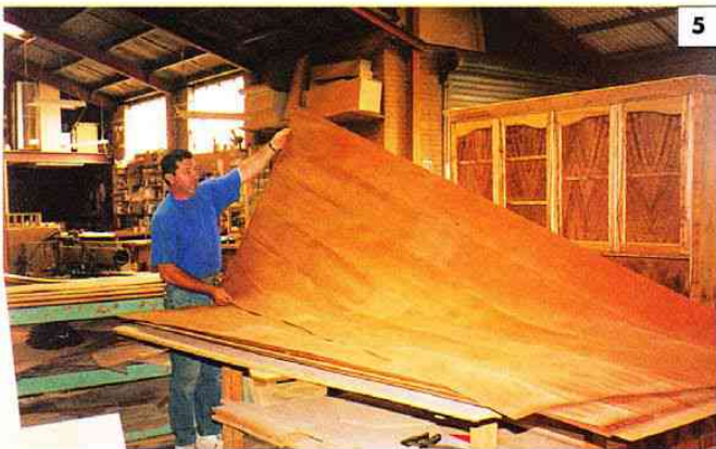
5 Veneer lay ups for the four quarters have been cut and joined. A final inspection of the quarter bookmatch joint.
