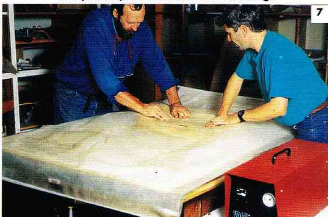
7 Morris and Mclean hold the laminates in place as the vacuum pump is turned on and the bag collapses.
