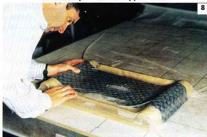
8 The former and laminates are checked finally before being left to harden. The scrap of carpet acting as a caul helps even the pressure on the glued veneers.
