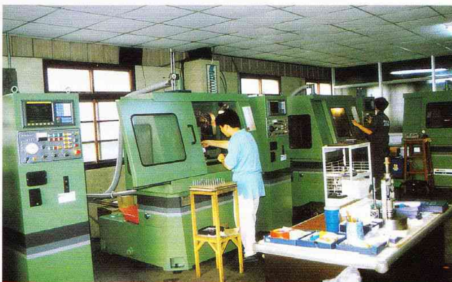
Top: A technician precision grinds solid carbide router cutters at Carb-I-Tool. Centre: Brazing carbide tips onto the router body. Photos: Debbie Butler. Above: Grinding tungsten carbide tips on a CNC machine in a router manufacturing plant in Taiwan. Photo courtesy Carba-Tec.
