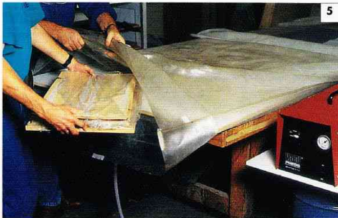
5 The former and laminates are covered with plastic wrap and placed in the vacuum bag.
