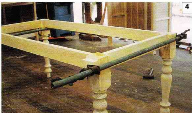
Short rails being glued in. Use two cramps for each rail to spread the pressure more evenly.
