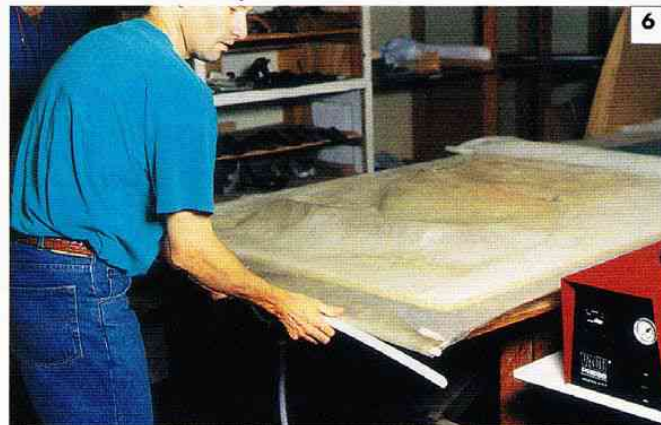
6 A plastic tube seals the bag which is wrapped around. Another split tube is clipped over.
