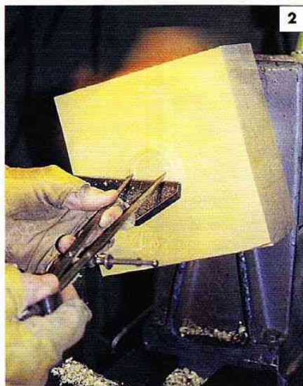
Marking the spigot diameter.
