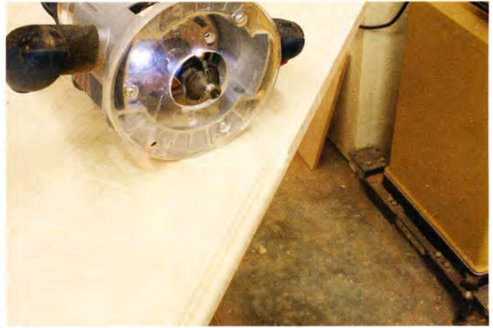
23 The bottom molding and the top have the same cove-and-bead profile. The bottom edges are rounded with a \frac{3}{16} " roundover bit.
