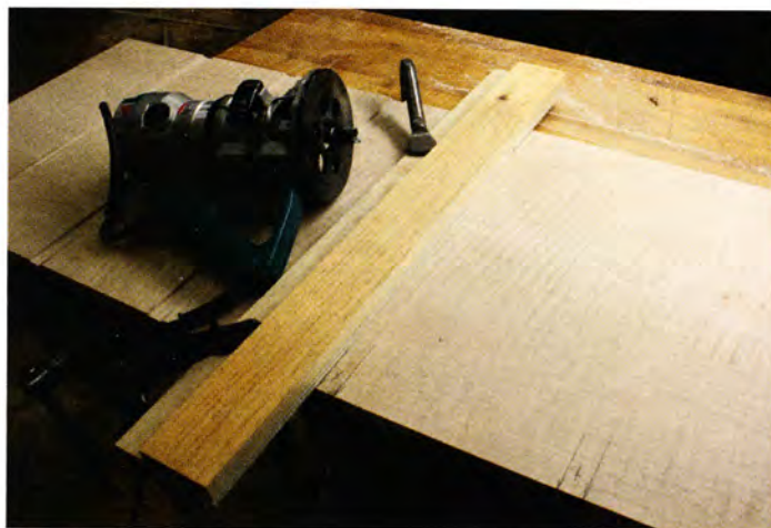
5 A piece of plywood with a narrow second piece stacked and attached on top makes a great fence to guide my router and top-mounted pattern bit when cutting the dados.
