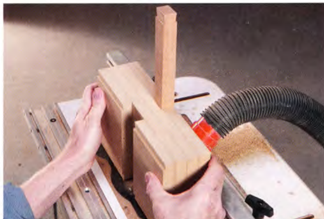
2 Rout both sides of each rail using a vertical jig.
