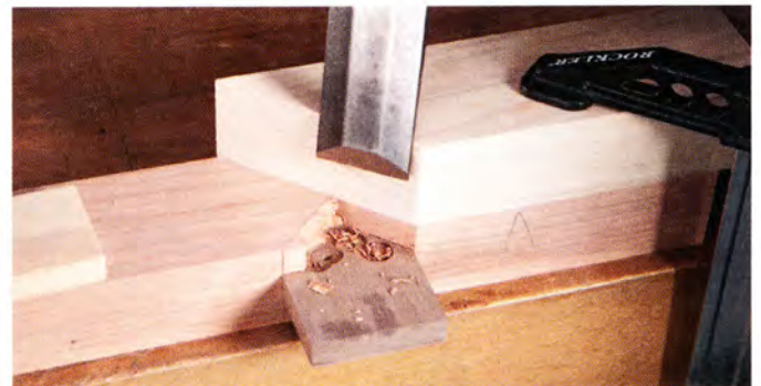
7 Use a guide to pare miters next to a mortise.
