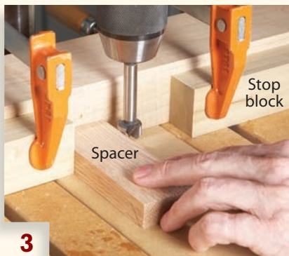
3 Use the spacer to set up two stop blocks on either side of a Forstner bit.
