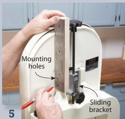
5 Fasten the plates to the riser blocks, then mark the location of the mounting holes on the saw.
