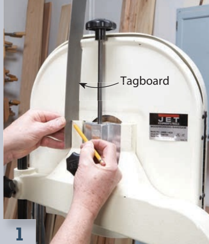
1 Trace around the contours of your saw to make a pattern.
