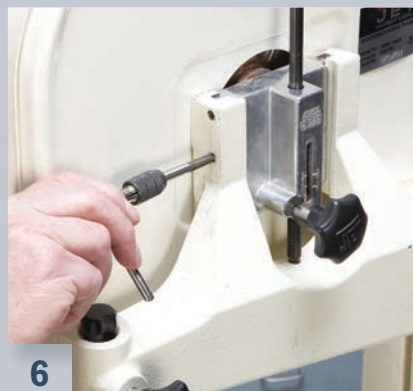
6 Drill and tap the mounting holes.
