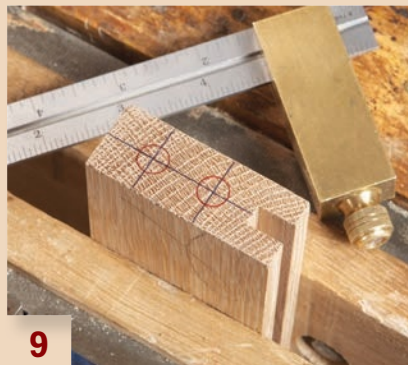
9 Lay out the dowel holes. They can be spaced any way you wish.
