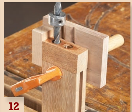
12 Drill the rails. Again, butt the jig against the outer edge of the rail.
