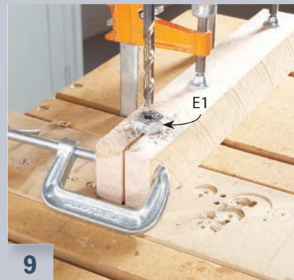
9 Drill a hole in the head of a short bolt (E1). This "adapter bolt" will connect the piston to a long all-thread rod.
