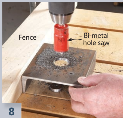
8 Drill a large hole through the mounting plate to accommodate the air cylinder's piston. Fasten the cylinder to the plate.
