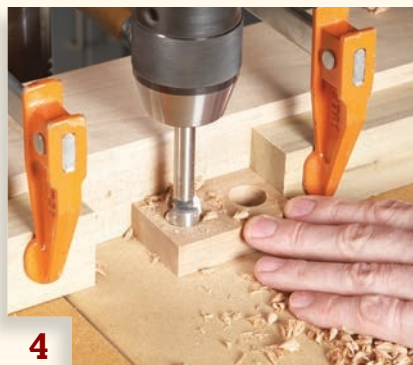
4 Drill holes for the doweling jig's flanged sleeve bearings.
