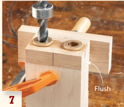
7 Flush Clamp the jig flush with each side of a rail.
