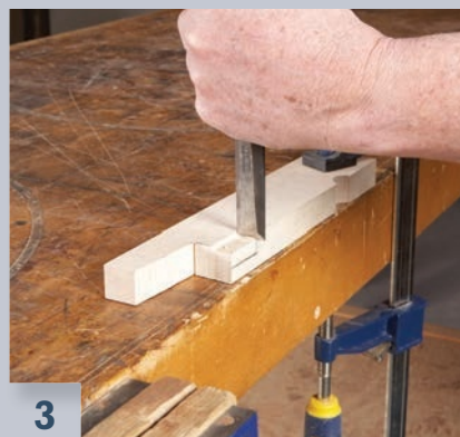
3 Chop a recess for the bandsaw's sliding bracket (see photo 5). The bracket will rise into this recess as the blade is tensioned.
