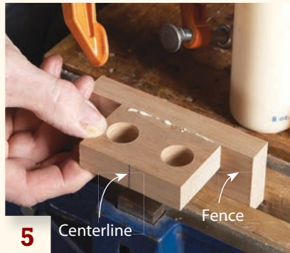
5 Centerline Fence Glue the block to a fence. Mark a centerline on the block.
