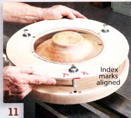
11 Install the ring and use it to clamp the bowl to the plywood base using bolts, washers and wing nuts.
