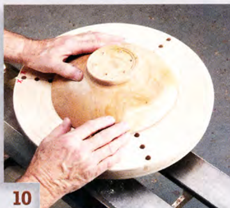
10 To use the chuck, start by roughly centering a bowl on the appropriate groove cut in the base.
