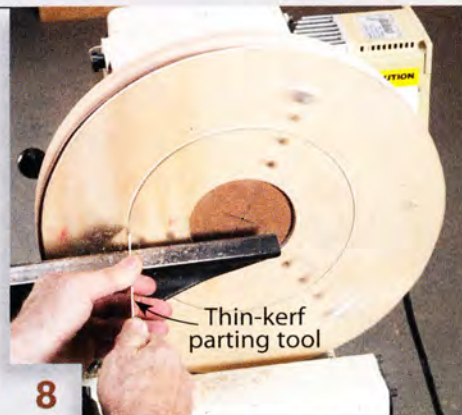
8 Cut through the disc to create the rings. Cut out the waste at the center. Then cut the small ring to create the large ring.
