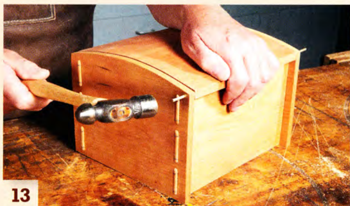
13 Install the lid by tapping home the hinge pins.
