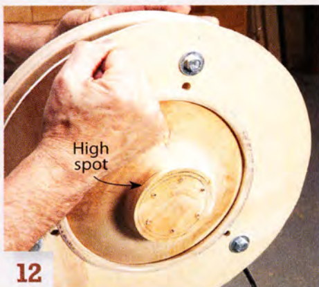
12 Center the bowl with the chuck mounted. Mark the high spot. Gently tap it as necessary and then tighten the wing nuts.
