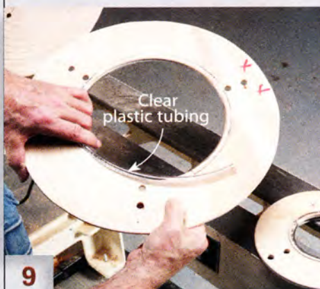
9 Line each plywood ring with clear plastic tubing that's been split with a utility knife.
