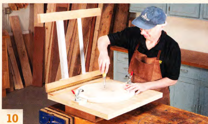
10 Fasten the workpiece to the turntable. The center of this pattern will be cut out later, so it's OK to put the screws there.
