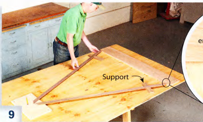
9 Locate the center of the arc. First, place the radius sticks on the endpoints of the arc (see inset). Support each stick with a block that's the same thickness as the workpiece.
