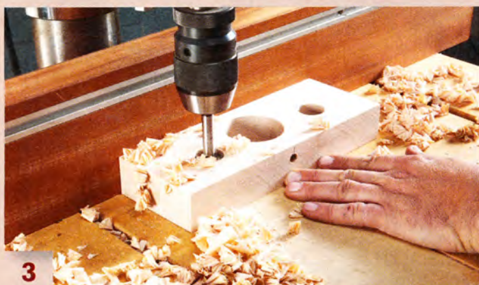
3 Drill the two smaller holes that define the insides of the handles, also using a Forstner bit.
