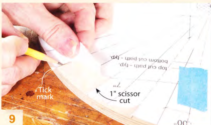
9 Mark the center of each V-groove by drawing a series of tick marks on the perimeter of the workpiece. Cut the pattern to guide your pencil.
