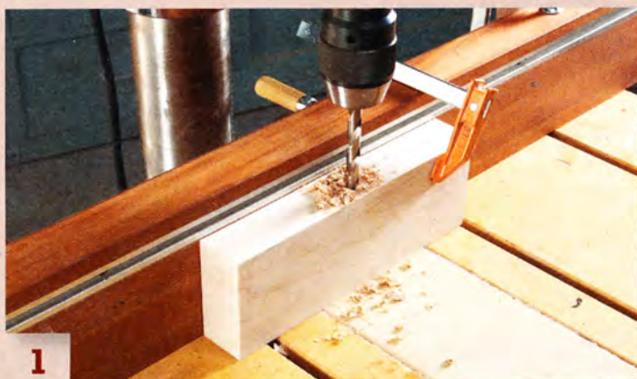
1 Drill a hole on the back edge of the plane body's blank for the cutter holder, which is made from a large thumbscrew.
