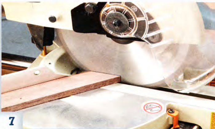
7 Cut two sticks that are the exact length of your arc's radius. For precise measurements later on, miter their ends.
