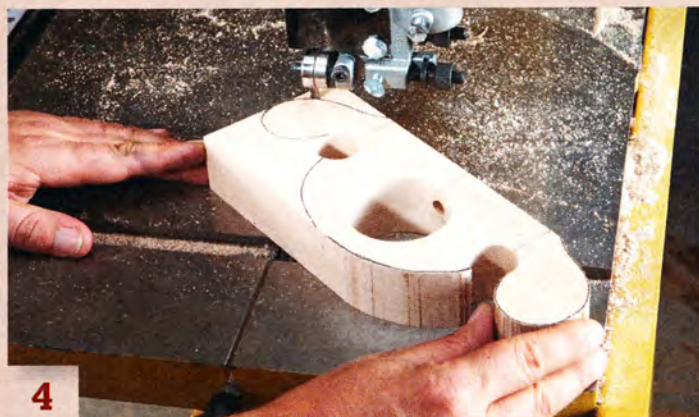
4 Bandsaw the body's shape. A jigsaw or coping saw would also work for this.
