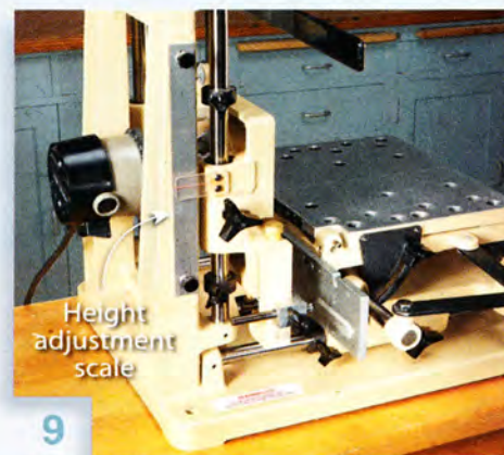
9 The height adjustment scale, primarily used to position the stylus, is very accurate. I often line up offset loose tenon mortises by sighting the scale.
