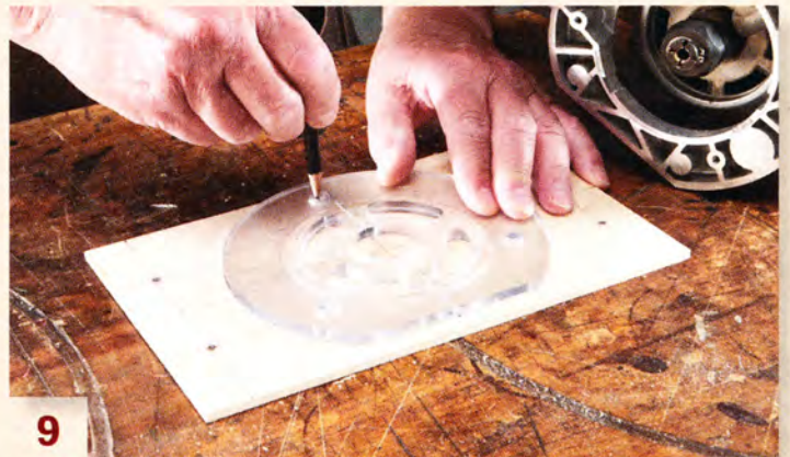
9 Make two platforms for the arm. This one will be drilled to fit a router; the other one is for use with a pencil.
