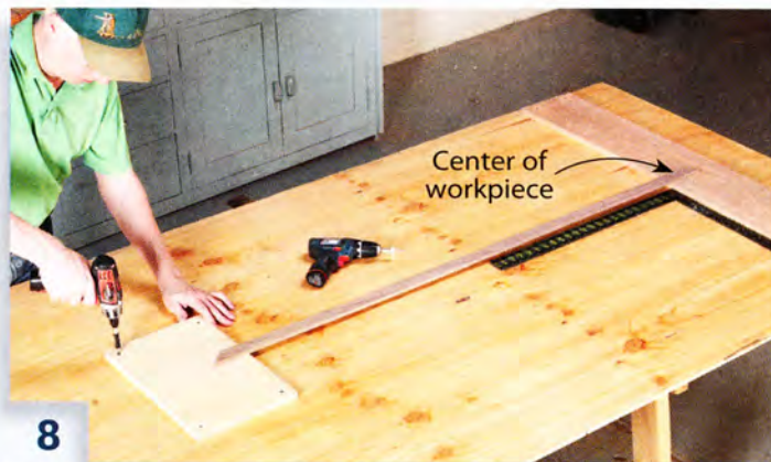
8 Fasten a block to the plywood to serve as a pivot point for routing the arc. Use one of the radius sticks to position the block—close is good enough.
