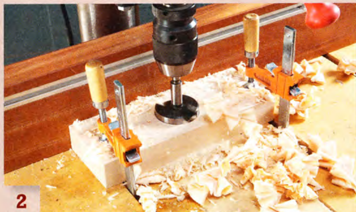
2 Drill the plane's large throat opening using a Forstner bit. Make sure your bit is sharp, so it doesn't burn the inside of the throat.
