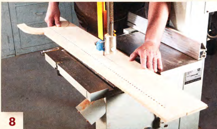
8 Make the jig's arm. Drill holes spaced 1/2" apart down the length of the arm, then cut out the arm's shape.
