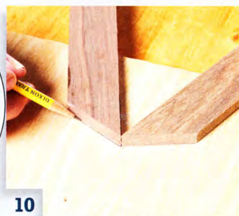
10 Position the other ends of the sticks so that their points meet. Trace around the miters.
