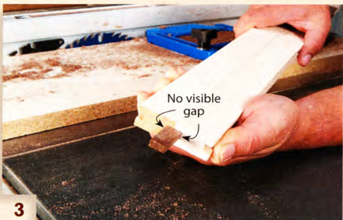
3 Check the splines' width using two grooved boards. There should be no visible gap at the spline's edges.
