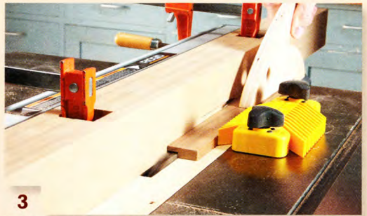
3 Rabbet the inside faces of the rails using a subfence.
