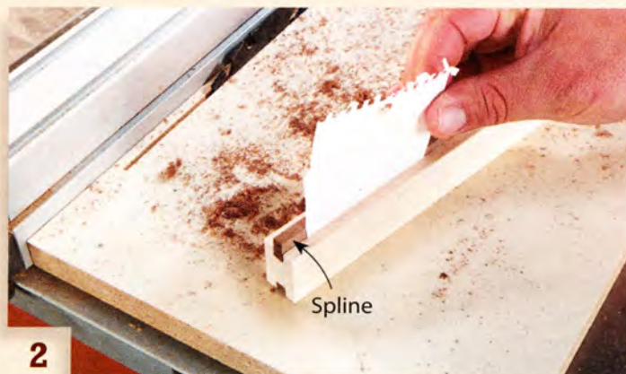
2 Cut walnut splines and test their fit. The splines should fit snugly alongside two pieces of paper placed in a groove.
