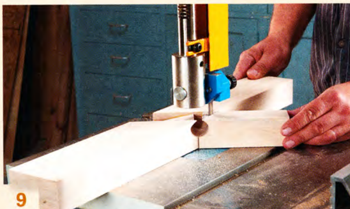
9 Bandsaw the frog's ends flush with the infeed and outfeed.
