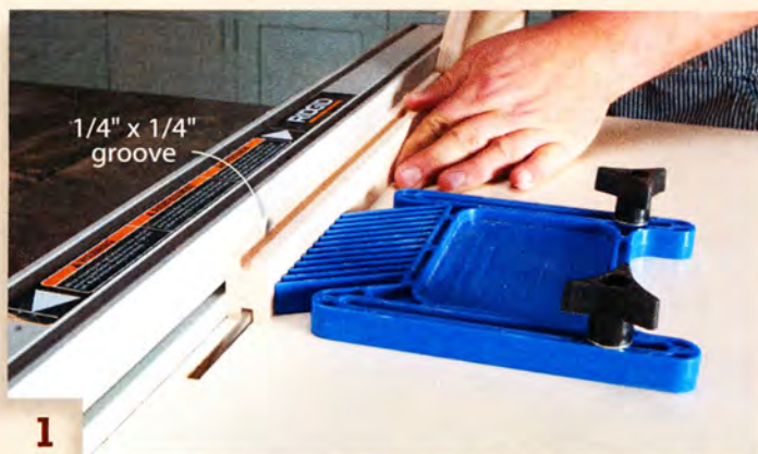
1 Cut grooves on both edges of a number of maple boards. Riding the boards on piece of melamine ensures an even cut.
