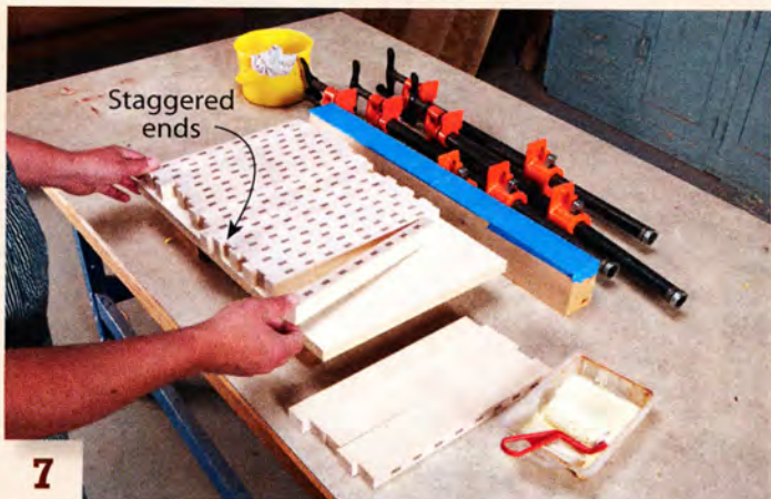
7 Glue the strips together on a sheet of melamine, staggering their ends. Use cauls again to keep the cutting board flat.
