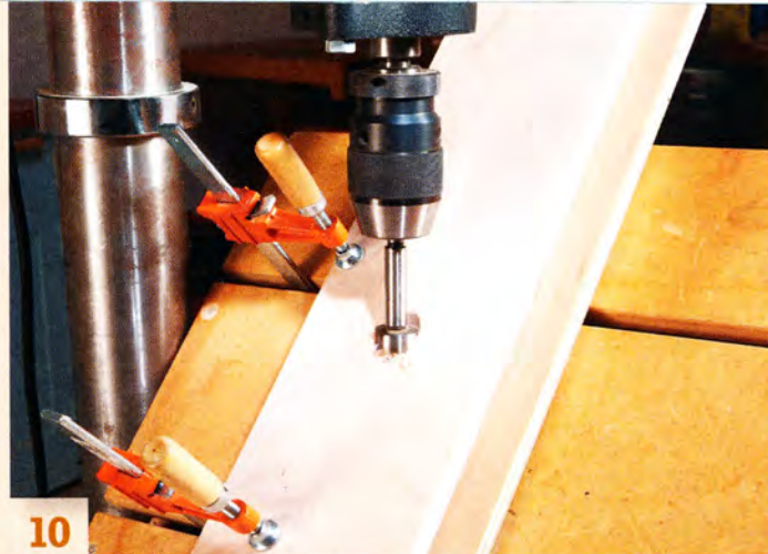
10 Tilt the table of your drill press to make an angled escapement hole in the plane's fence. Glue the fence to the plane's body.
