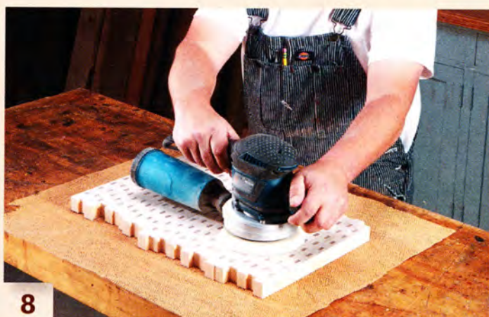
8 Sand with coarse paper until the surfaces are even, then finish-sand. Trim the sides to make a cutting board any shape you wish.
