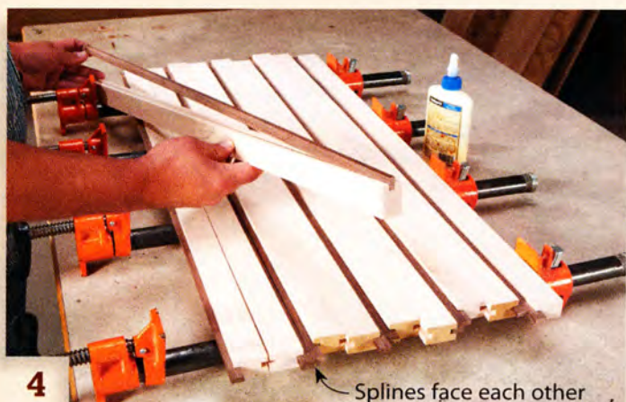
4 Glue each spline in only one grooved board. Clamp the boards with the splines facing each other to press them into place.
