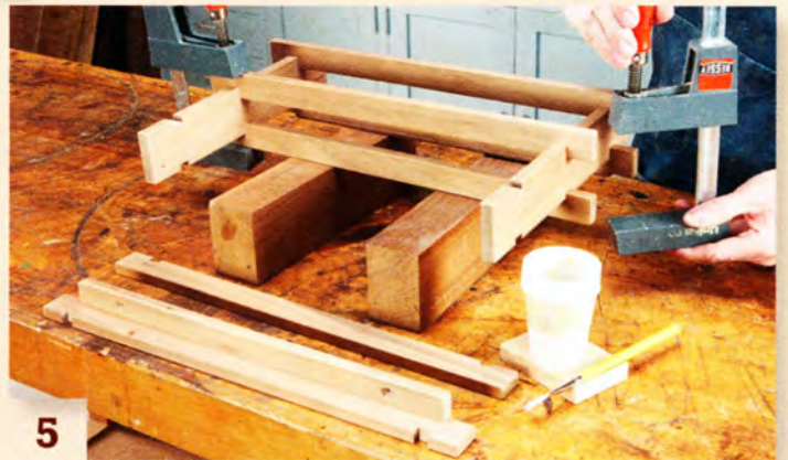
5 Glue all of the shelf pieces to the ends of the wine rack. It's very easy to clean up glue that squeezes out of the joints—it will pop right off the finish.
