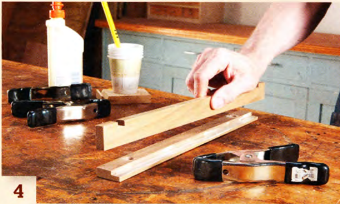
4 Glue the two shelf pieces to the rails. Of course, you have to remove the tape from the shelf pieces first!
