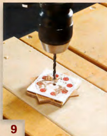
9 Enlarge the center hole to 3/16"—the size of the gear's axle.
