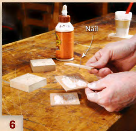
6 Insert a 3d nail through the top piece. Apply glue and rotate each piece 45°.
