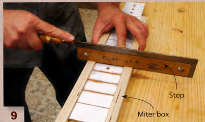
9 Cut slots in the fretboard for the faux frets using a shop-made miter box. Attach a stop to the saw in order to cut the kerfs to a consistent depth.
