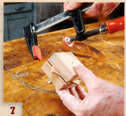
7 Clamp the stack between cauls. The nail keeps each piece centered.
