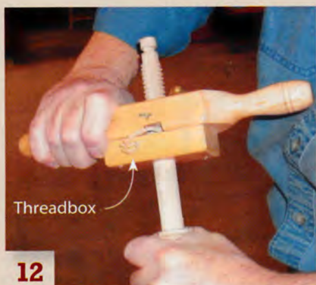
12 Use a threadbox to cut the threads on the screw's shaft. Work back and forth as necessary to clear the waste.
