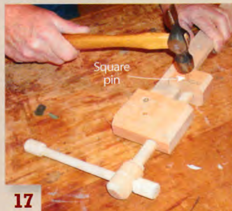
17 Capture the screw by driving square pins into the holes, so they track inside the groove in the screw's tenon.
