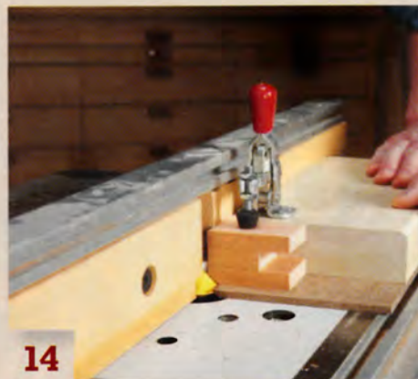
14 Use a sled to chamfer the sliding jaw. Make the sled by gluing a squared block onto 1/4" hardboard and attaching a toggle clamp.
