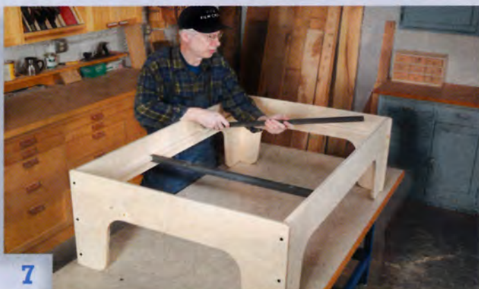
7 Install steel angle iron in the gaps between the ledger pieces. The rigidity of the angle iron prevents the platform from sagging.
