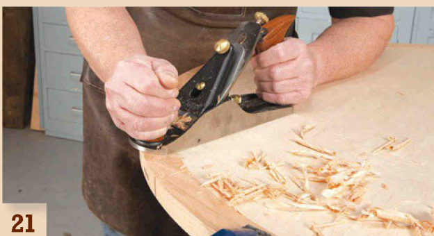
21 Plane the rim almost flush to the plywood, then scrape or sand the rim even with the plywood.
