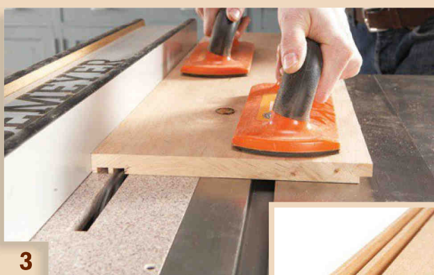
3 Cut grooves for the sliding doors in the top and bottom shelves. The grooves in the top shelf are deeper (right).
