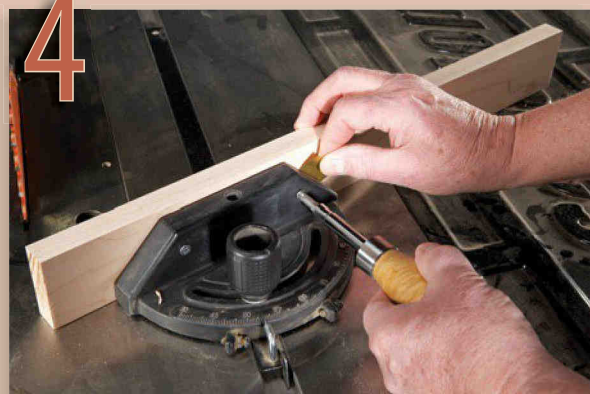
Set your saw's miter gauge using the triangle. Saw a test set of eight pieces.
