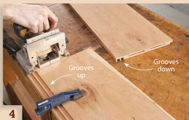
4 Cut slots in the top and bottom shelves on a flat surface, with the biscuit joiner held horizontally. Clamp the bottom shelf grooves up and the top shelf grooves down.
