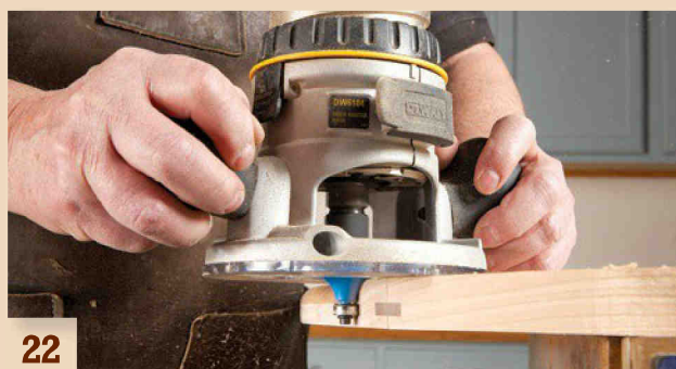
22 Rout a roundover or other profile around the tabletop. Be sure that the routing doesn't cut into the splines—after all this hard work, that just wouldn't look right!
