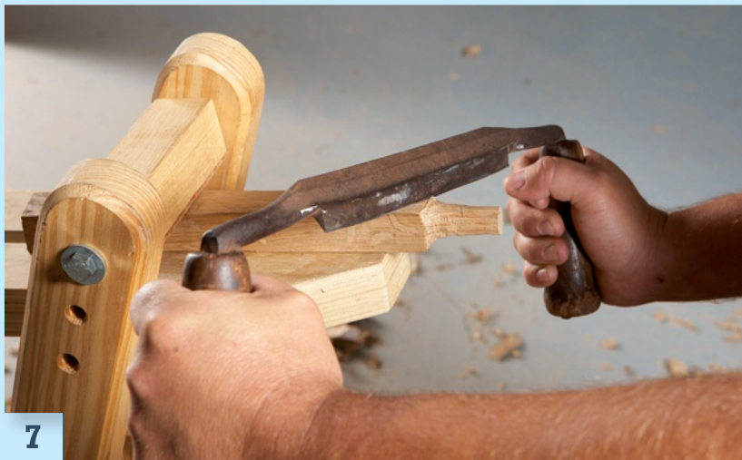
Form round tenons on the ends of the sled's posts using a drawknife. A shaving horse is ideal for this kind of job—it gives you plenty of room to maneuver the drawknife.
