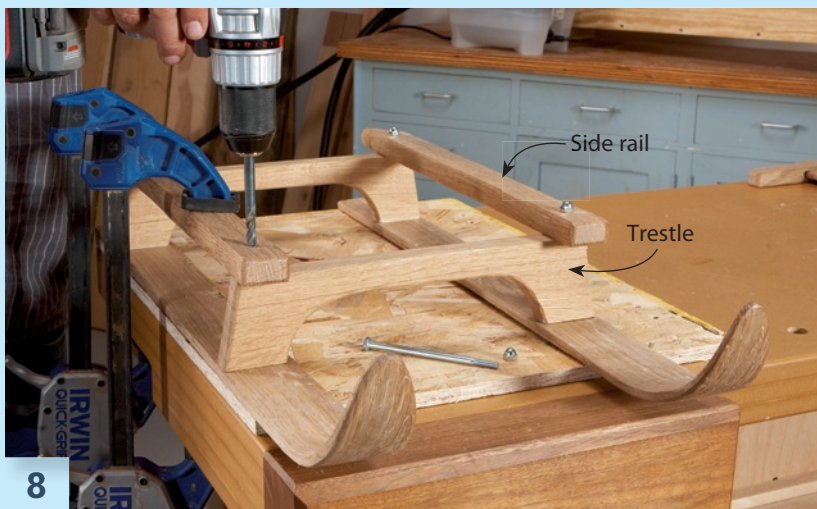
Drill through the side rails, trestles and runners using an extra-long bit. Clamp the parts to your bench to keep them aligned. Assemble the parts using a bolt and acorn nut.
