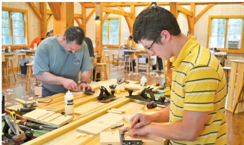
The New Legacy School's three-part foundation course teaches basic hand woodworking skills. In each part, students learn to use the necessary tools to build a project designed around one or more essential joints.
