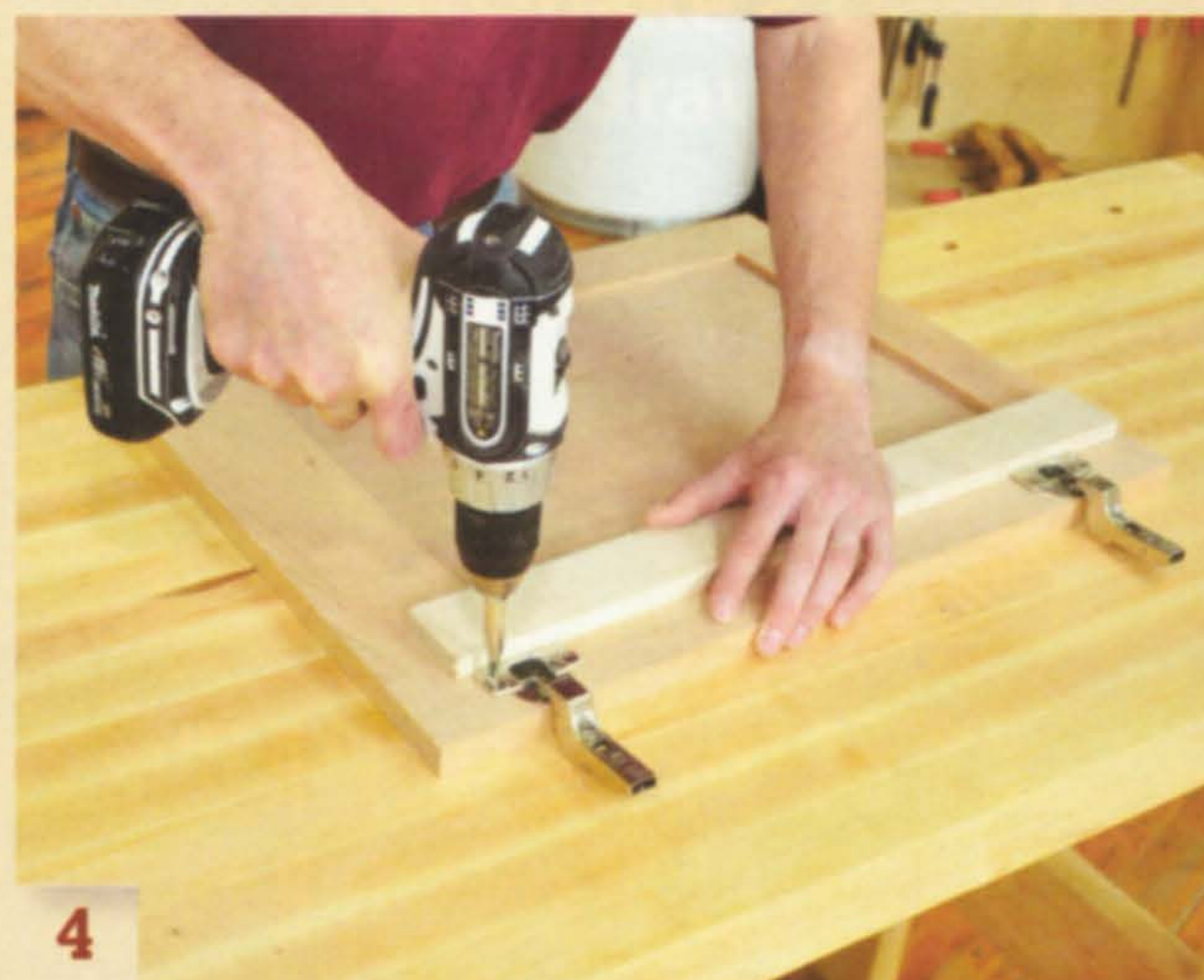
Install the hinges. Insert each hinge cup in its hole. Then use a scrap board with a straight edge to align the hinges parallel with the edge of the door.
