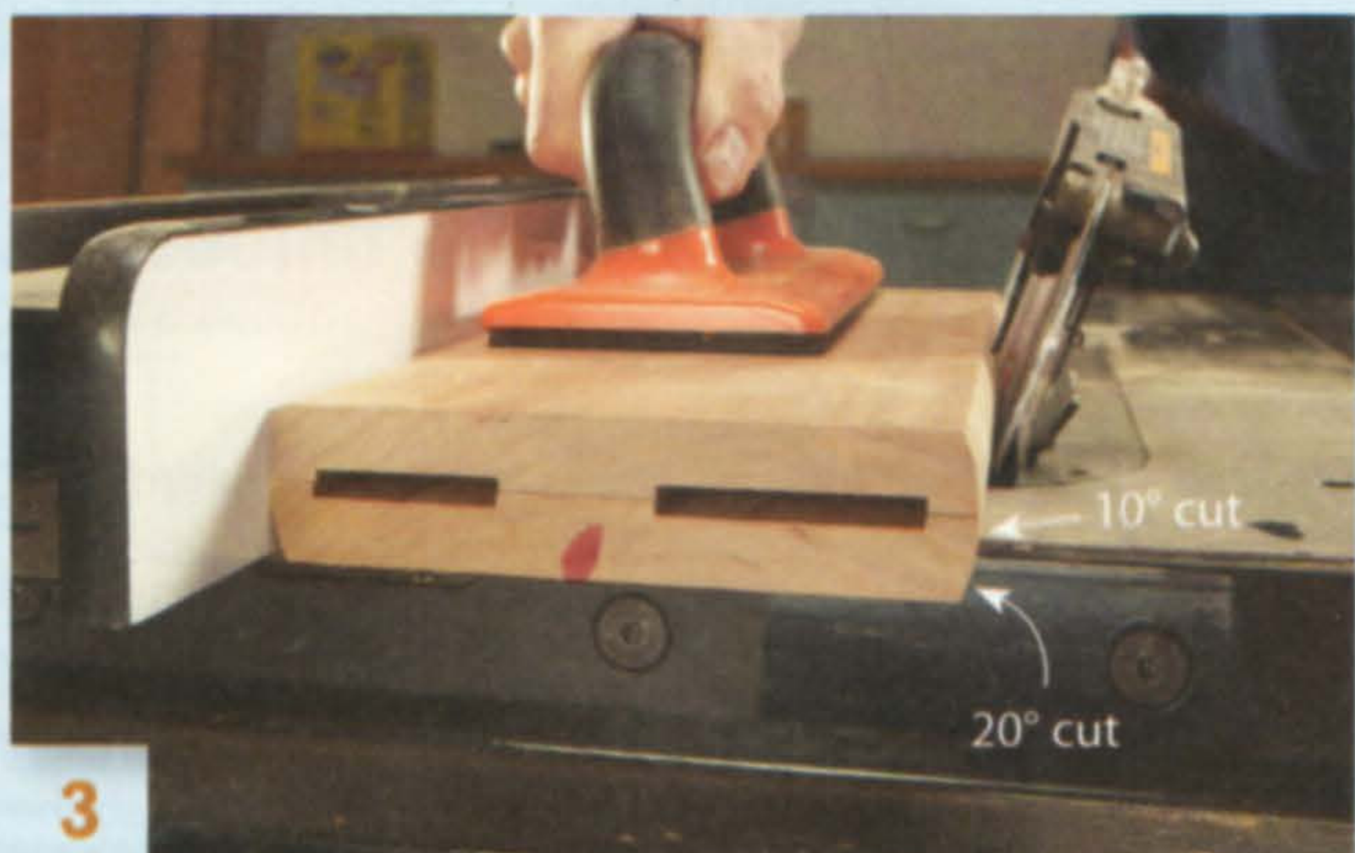
3 Saw the sides of the blocks at two different angles to begin forming a curved edge.
