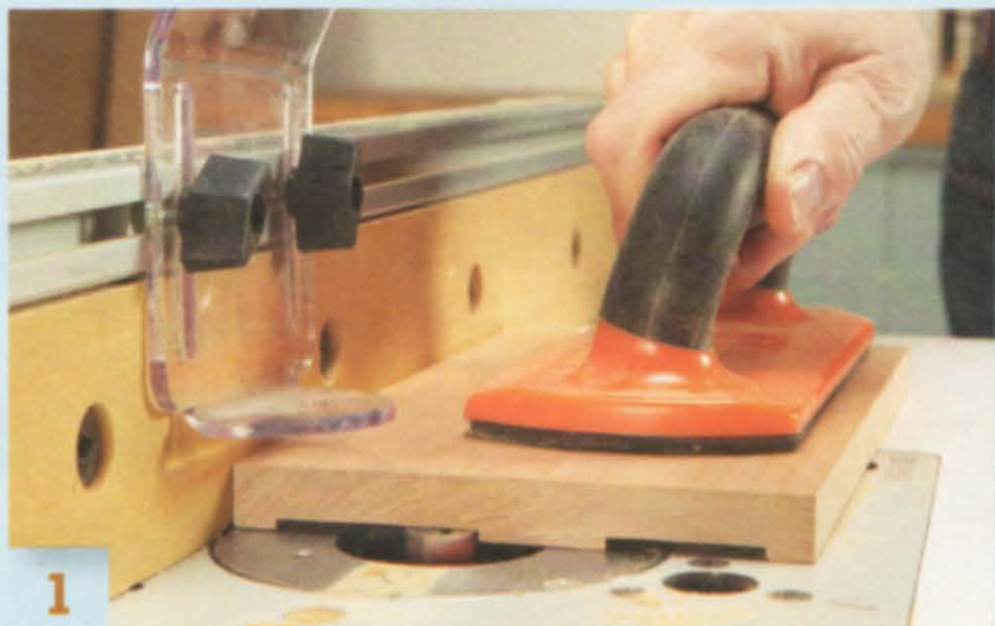
1 Each section of the knife block is made from two pieces of wood. Rout shallow grooves in each one.
