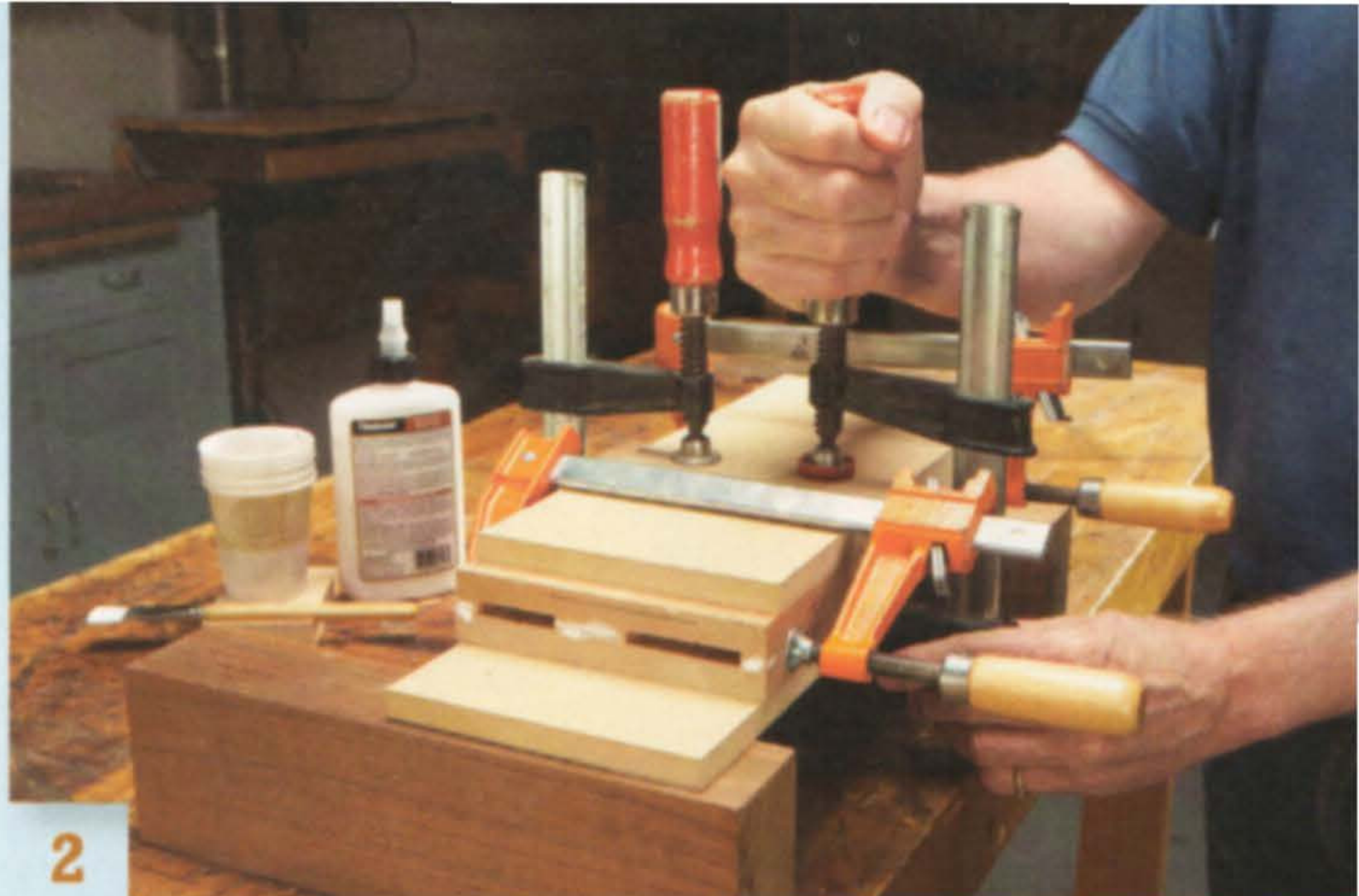
2 Glue the pieces together. Note that the end grain should curve in the same direction on both pieces. This helps create the illusion that the glued-up pieces are a single block of wood.
