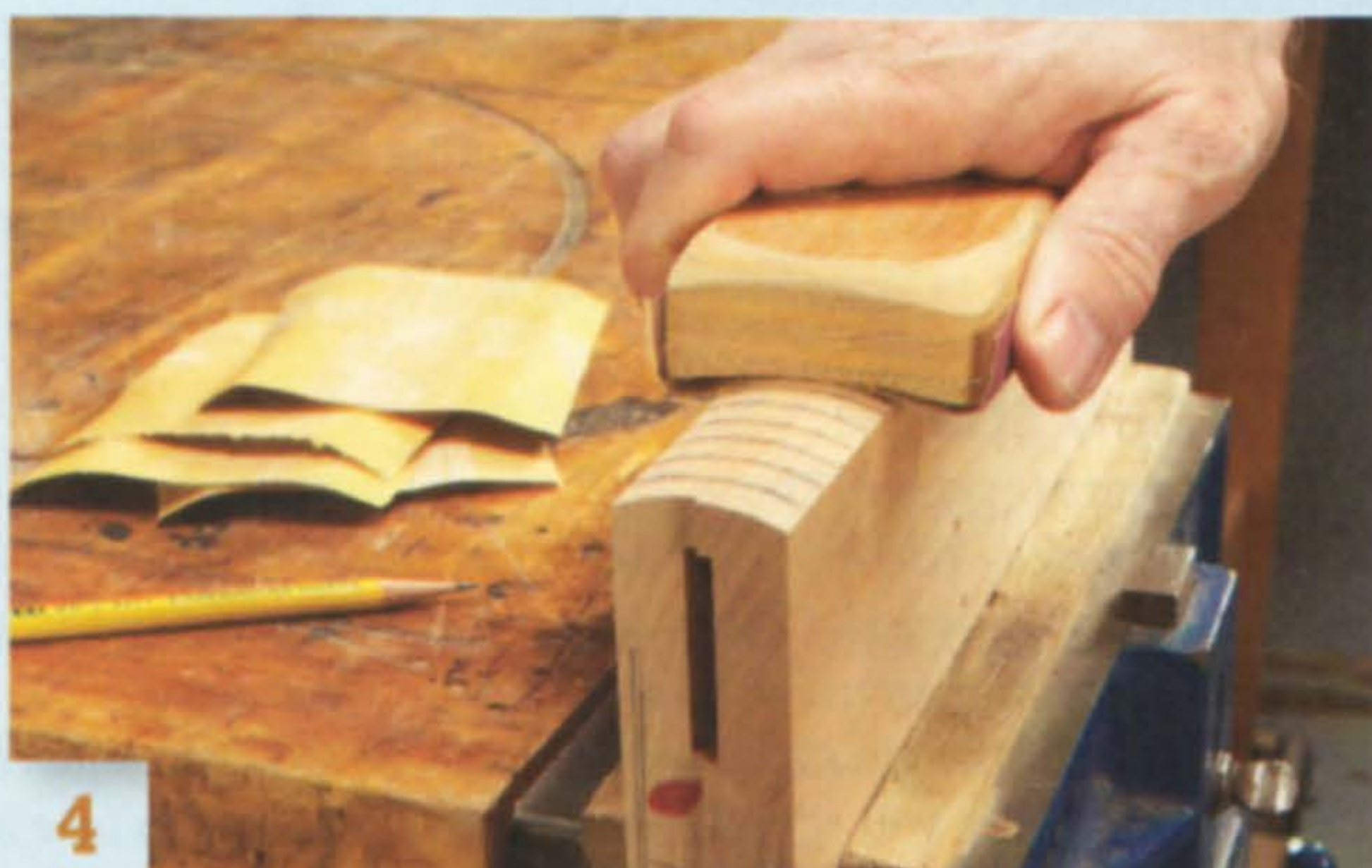
4 Sand each side with a curved sanding block. Keep sanding until all the pencil marks are gone—this indicates that all the flat areas are now curved.
