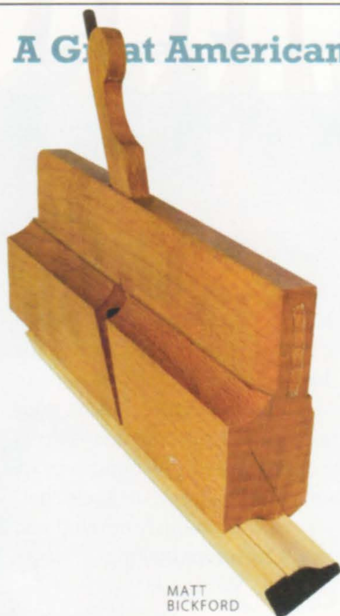
Dedicated molding planes allow cutting a specific profile with a single plane. This plane cuts a 3/4" ogee with a fillet.
