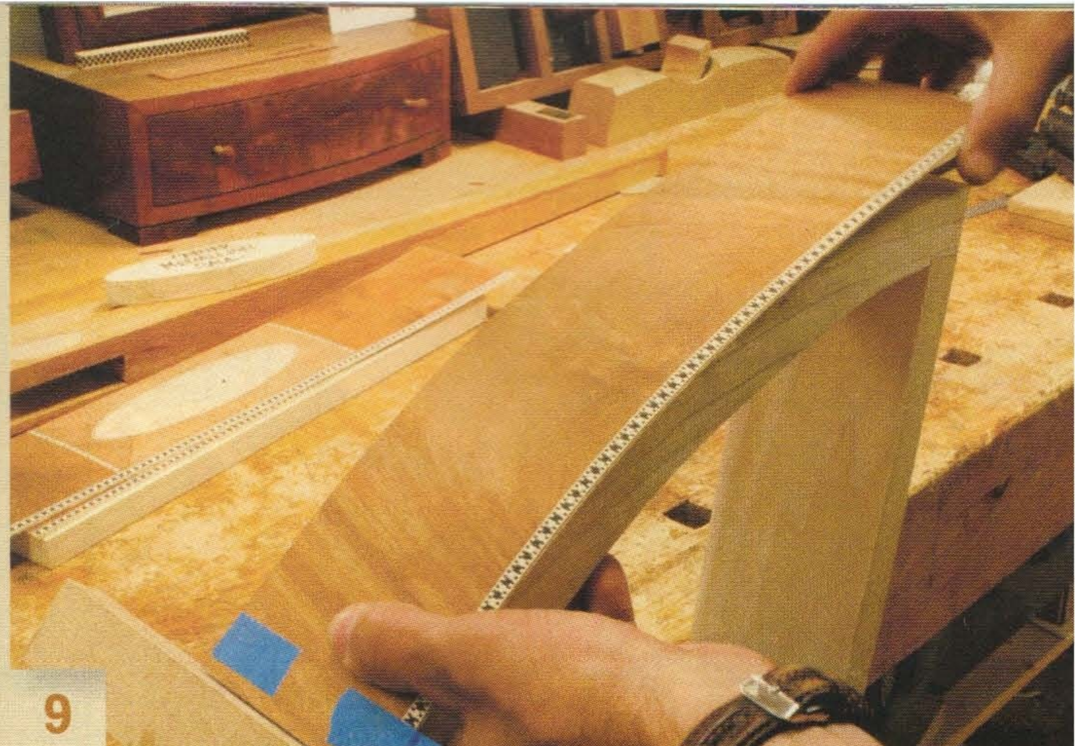
9 Prepare extra-thick veneer for the apron. I make it myself by gluing standard-thickness veneer (and banding) to a flat board first. Resawing this board yields extra-thick stock.
