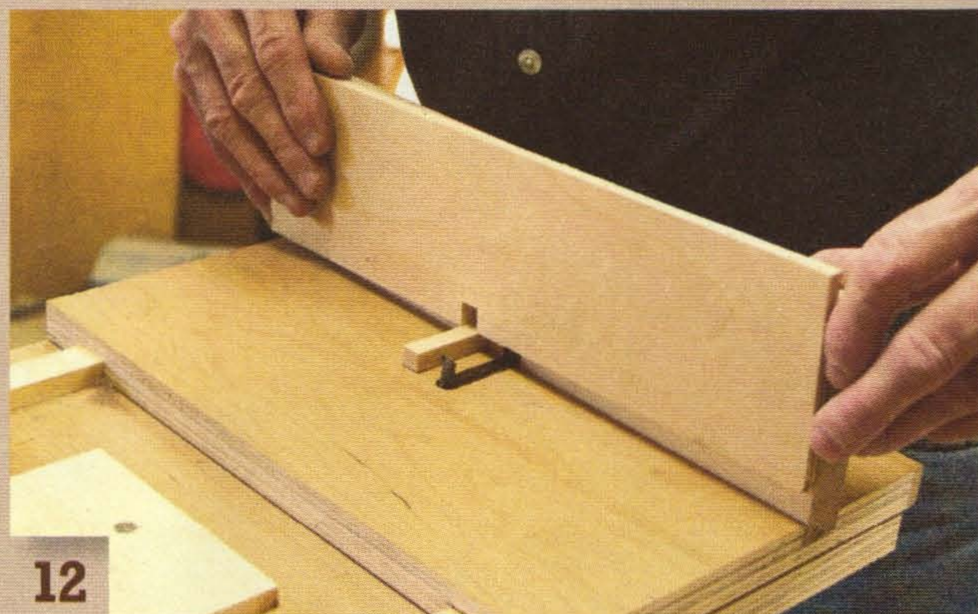
12 Make an auxiliary fence to eliminate tearout when you rout joints in thinner stock. Set the bit's height for the thinner stock, use the key to index the fence and rout a new, shorter slot.
