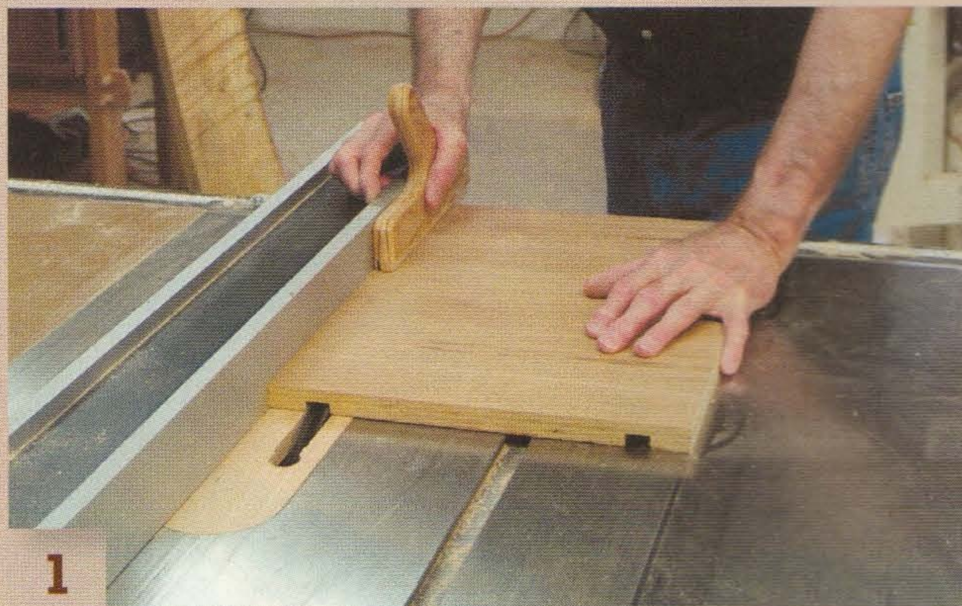
1 Create the jig's base and sled from a single blank. Cut dados for the runners, then rip the blank into the two parts. This method ensures the slots will align.
