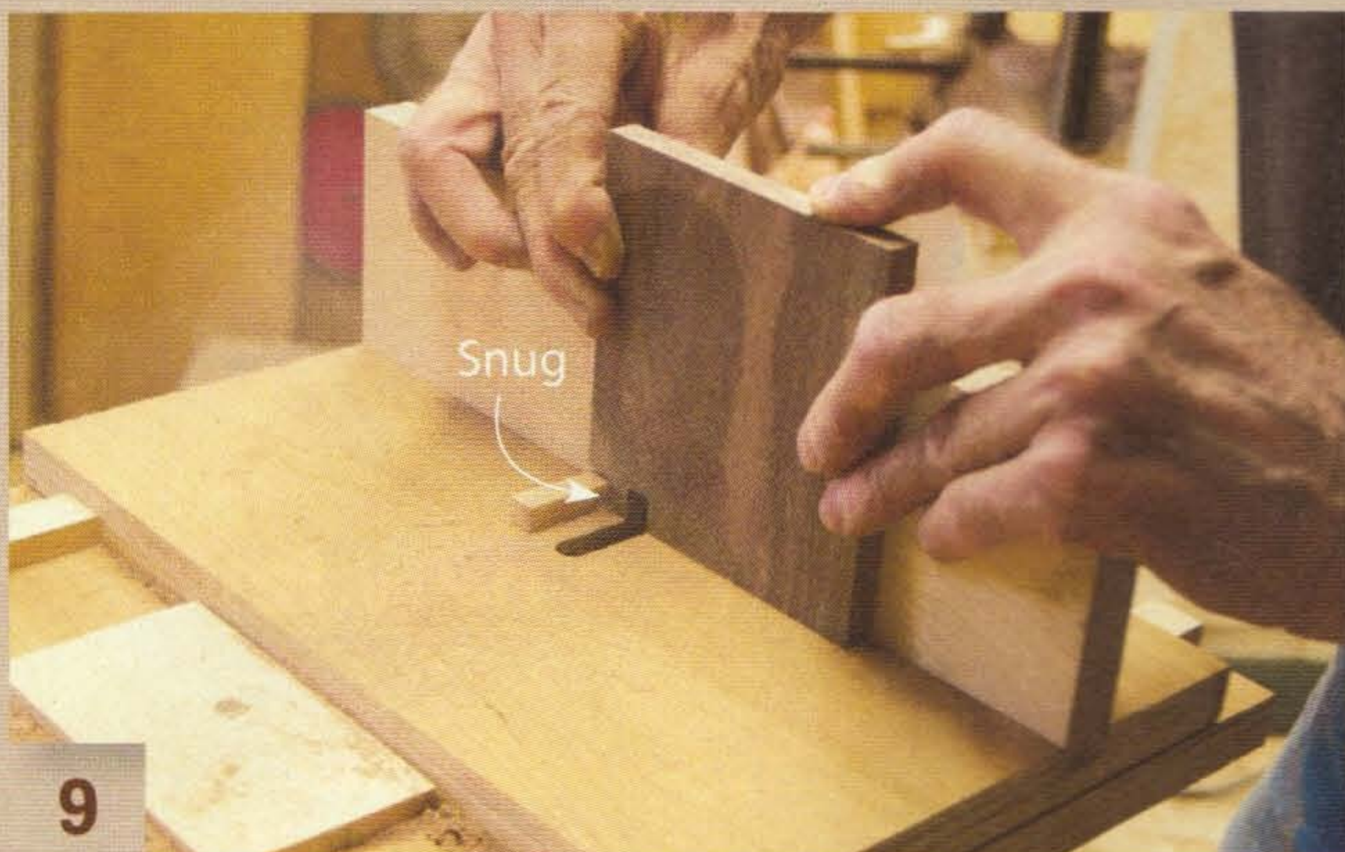
9 Use the key as before, to index the second test piece for routing each remaining socket.
