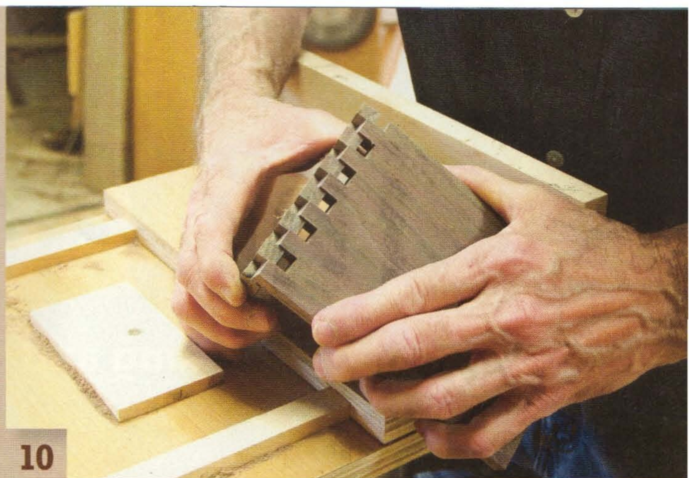
10 Test-fit the joint. The parts should slide together without wobbling or binding and the pins should stand slightly proud, so they're easy to sand flush.
