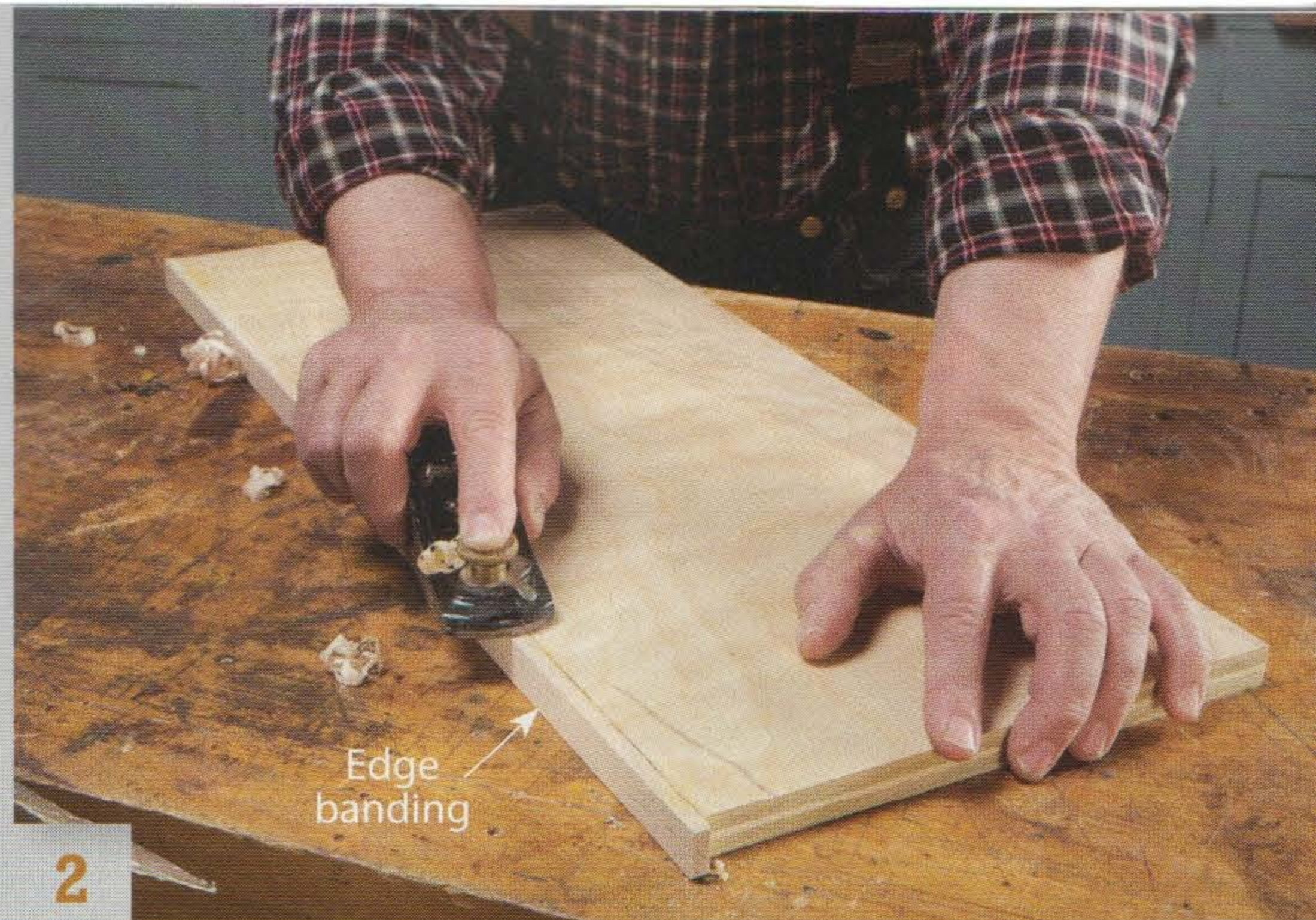
2 Plane the edge banding nearly flush with a block plane. Then finish the job by hand sanding with a block. Power-sanding is risky because the veneer is so thin.
