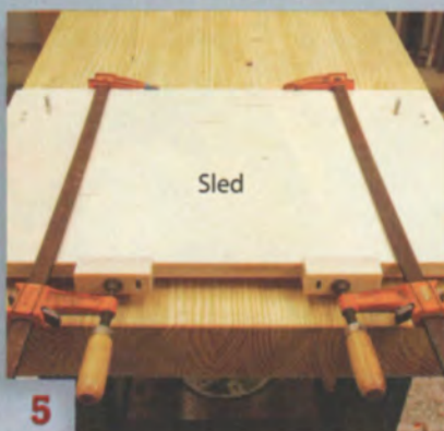
5 Glue the adjustment blocks to the front of the sled, spaced 6" and flush with the bottom.
