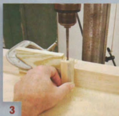
3 Drill a hole through each adjustment block and flipper block. Provide additional support to securely hold these narrow pieces.
