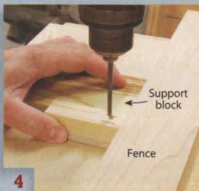
4 Create a housing for the captured nut in each adjustment block by drilling overlapping stopped holes.
