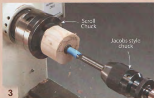
3 Turn the blank end-for-end and mount it in the scroll chuck. Then use a Jacobs style chuck to bore a hole for the doorknob's metal shank.
