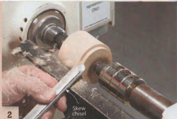
2 Make the doorknob first. Turn the blank to a cylinder. Then cut a tenon on the front end with a parting tool or a skew chisel, so you can mount the blank in a scroll chuck.
