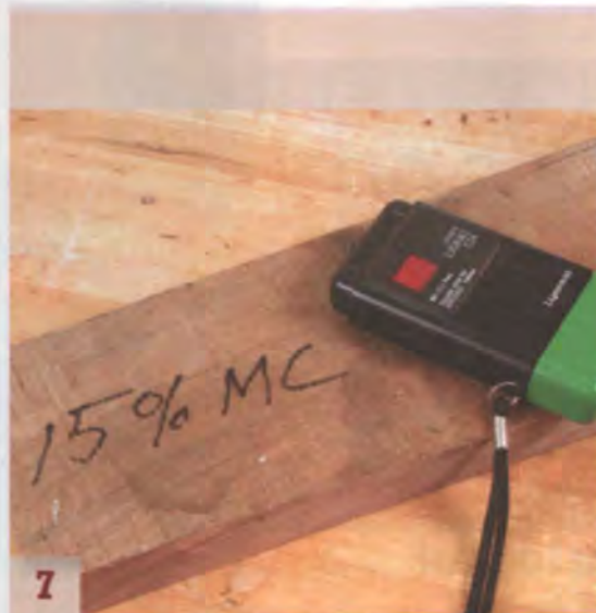
7 Air-drying lumber in my barn will bring the wood down to about 15% moisture content (MC). That's not dry enough for making fine furniture.
