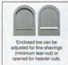
Adjust mouth by loosening front ball knob and sliding forward or backward.
