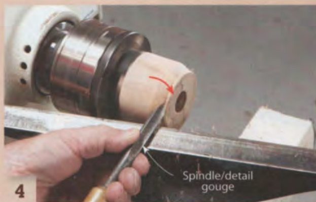
4 Use the spindle/detail gouge to shape the back of the knob. Make a rolling cut toward the hole in the end of the blank.
