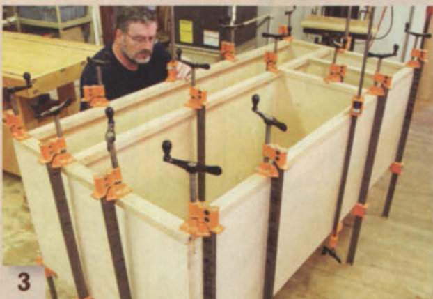
3 Build a face frame and glue it to the front of the box. The face frame consists of parts that are just butted and screwed together.
