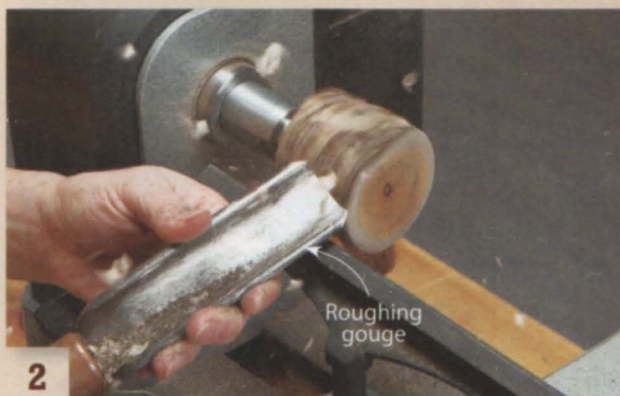
2 Round the blank to a cylinder using the roughing gouge. A large gouge produces a smoother cut than a small one.
