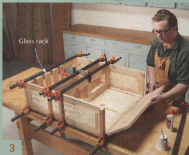
3 Glue the cabinet together in stages. Add the glass racks, web frames, middle shelf, drawer divider and bottom shelf after gluing the sides to the front.
