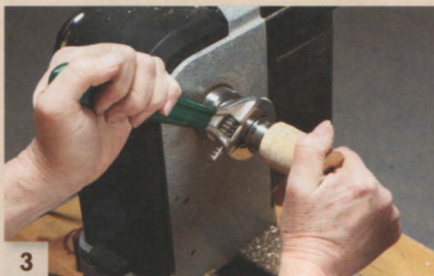
3 Unscrew the blank slightly away from the base of the cone chuck to prepare for the next step. The blank is tightly threaded on the chuck's post, so unscrewing doesn't loosen it.
