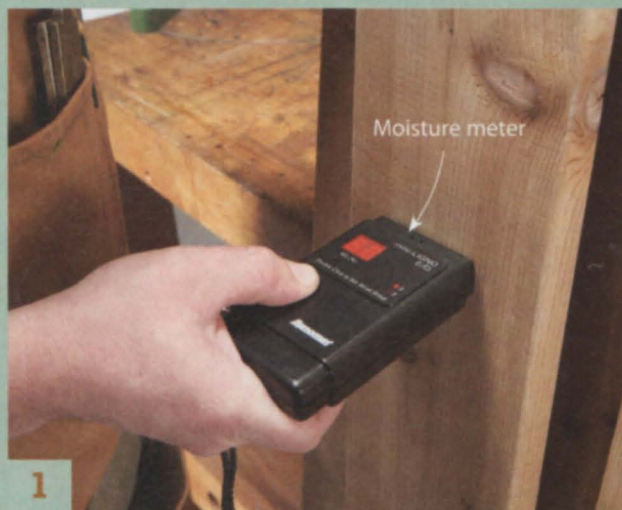
1 Check the moisture content of your lumber. Anything below 12% is fine. Although this patio bar will reside outdoors, it also contains moving parts and precise joinery, like any fine furniture piece.
