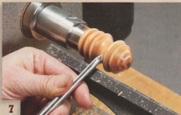
7 Define the stopper's body with coves and beads (seasoned turners call these "innies and outies").
