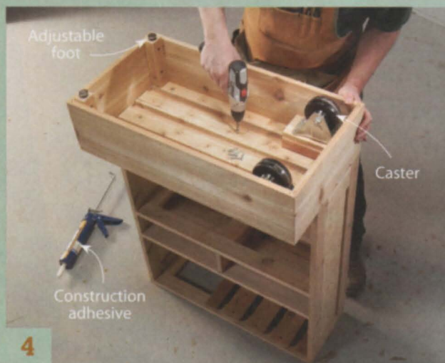
4 Attach the base to the cabinet using construction adhesive and exterior screws. Casters and adjustable feet hidden in the base add mobility and aid stability.
