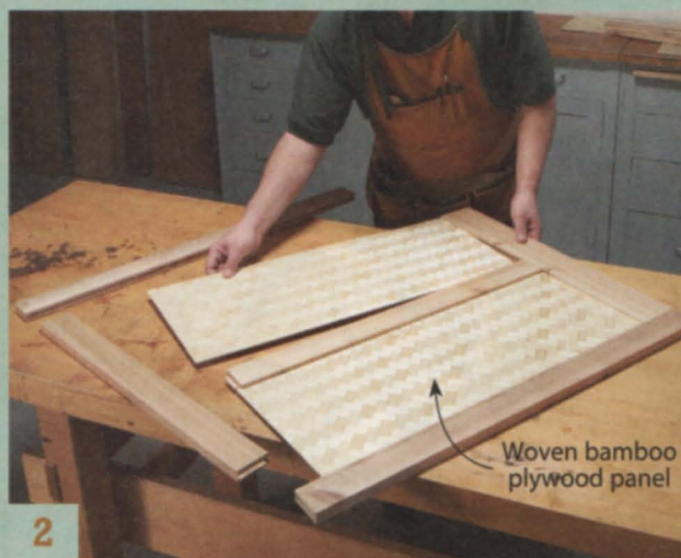
2 Make and assemble the frames for the cabinet's front and sides. These are standard stile-and-rail construction, but the panels are made from woven bamboo plywood.
