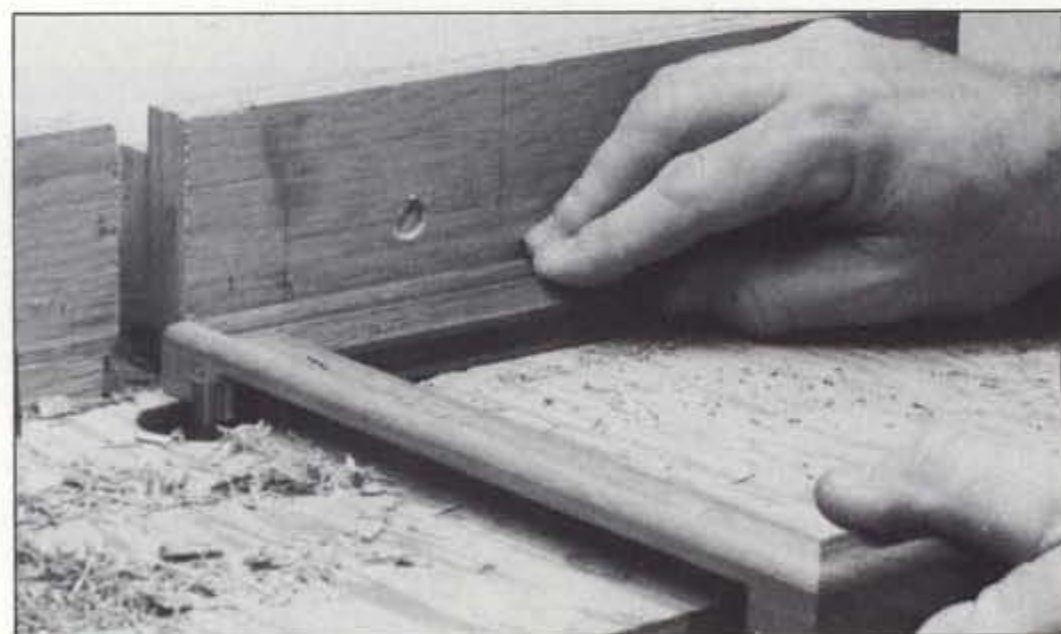
A router is used to remove wood from one end of the frame which allows the back to slide in.
