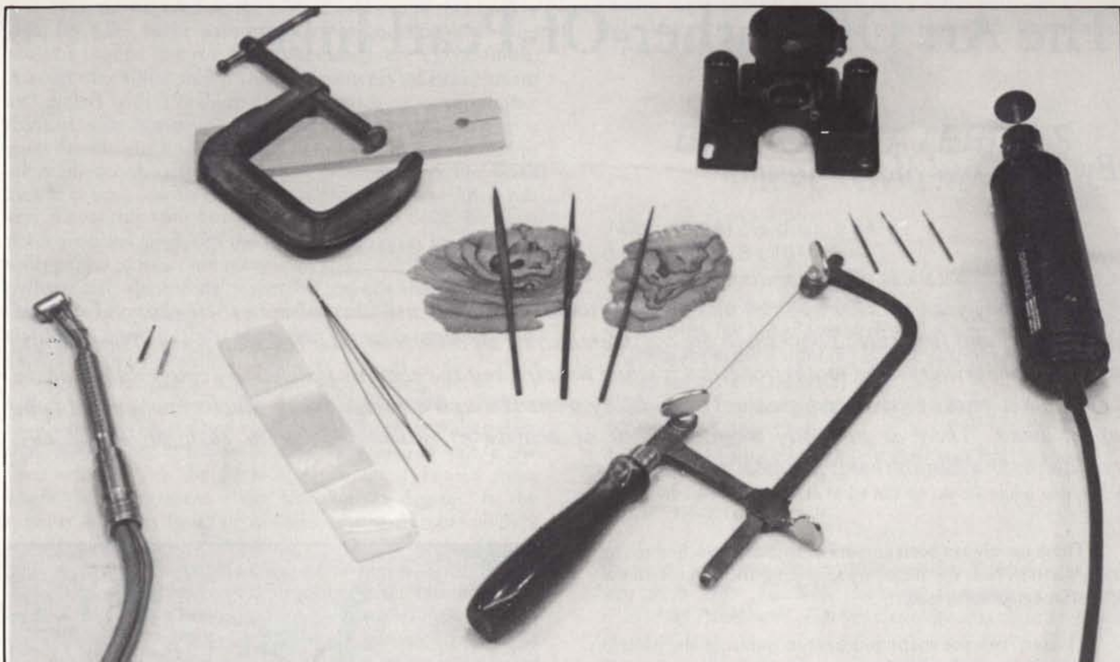
Useful inlaying tools: No. 280 Moto Tool w/cut off disc, engraving cutters and No. 229 base. Jeweler's saw frame and blades. Shell blanks and needle files. Sawing board and clamp. Dental drill and burs (could use flexible shaft instead).
