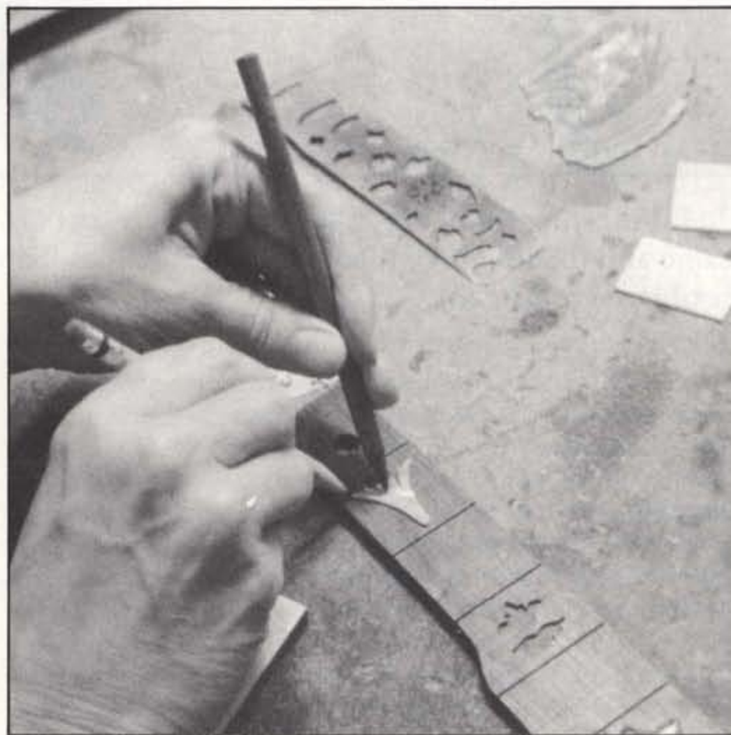
Example of the five steps to inlay. Pattern, draw around, relieve, glue in, sand off.
