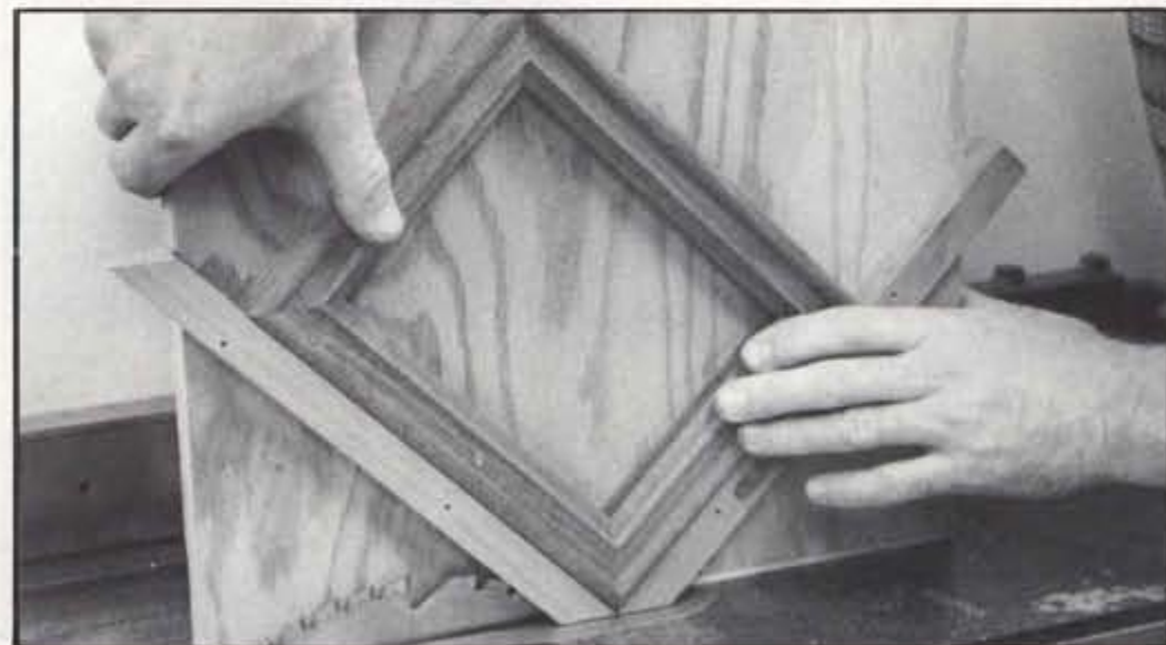
Slots for the 1/8 inch spline are cut across the miter joint. A homemade jig is used to hold the frame vertically, frame and jig are slid past blade.
