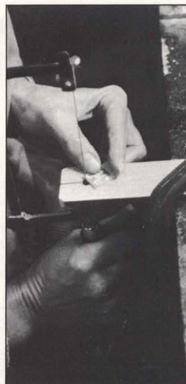
Handsawing an 'M' with the jeweler's saw.
